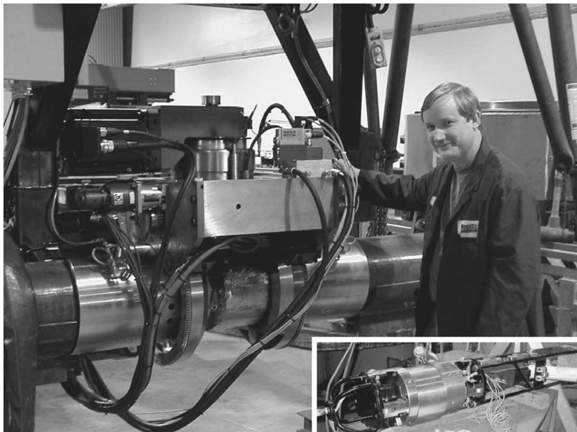
Fig. 13.36 Prototype pipe welding system showing external friction stir welded head and internal mandrel (inset). Courtesy of MegaStir, Inc.
