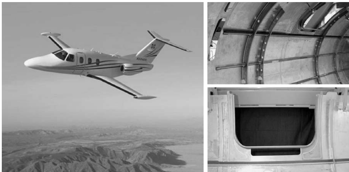
Fig. 13.33 The Eclipse 500 business-class jet is currently in final Federal Aviation Administration certification trials (left). The internal longitudinal and circumferential aluminum stiffeners (top right) and window and door doublers (bottom right) are attached to the aluminum fuselage section with friction stir welded lap joints. Courtesy of Eclipse Aviation
