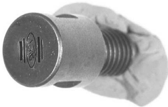
Fig. 12.53 Example of decorative anvil for the spot friction welding process. Source: Ref 48
