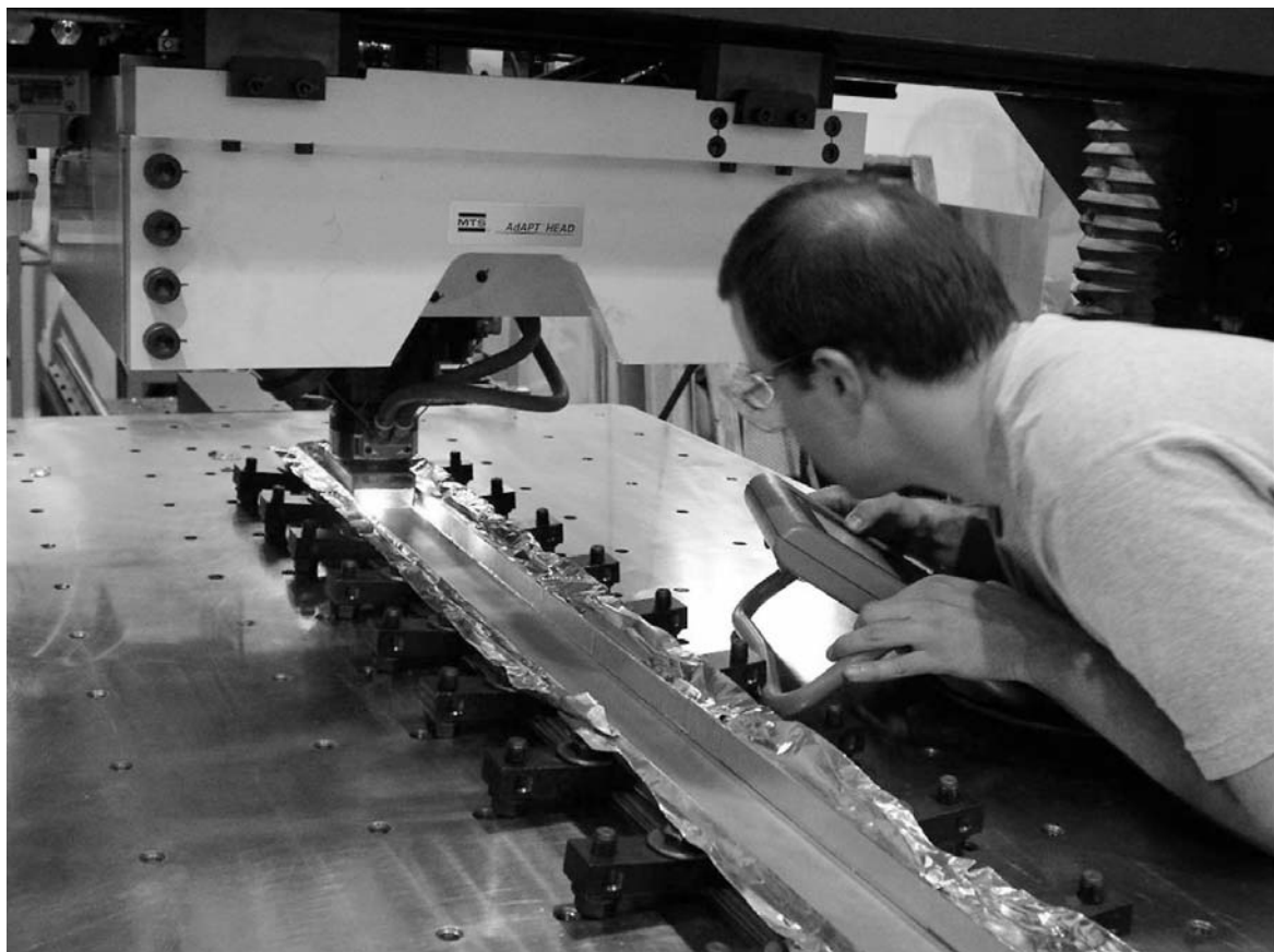
Fig. 13.37 Joining of long lengths of contamination-free Ti-6Al-4V is possible with out-of-chamber friction stir welding, using shrouds and trailing shoe shielding gas systems. Courtesy of Lockheed Martin Space Systems
