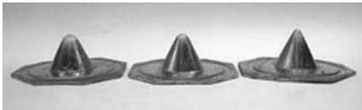
Fig. 14.9 Gas pressure cone tests for different conditions including (a) conventional superplastic 7475 Al alloy, 150 psi (1000 kPa), 95 min, (b) friction stir processed (FSP) 7475 Al, 150 psi, 18 min, and (c) FSP 7475 Al, 100 psi (690 kPa), 49 min
