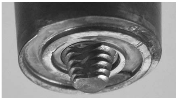
Fig. 2.7 Photograph of a scrolled shoulder tool and a truncated cone pin containing three flats
