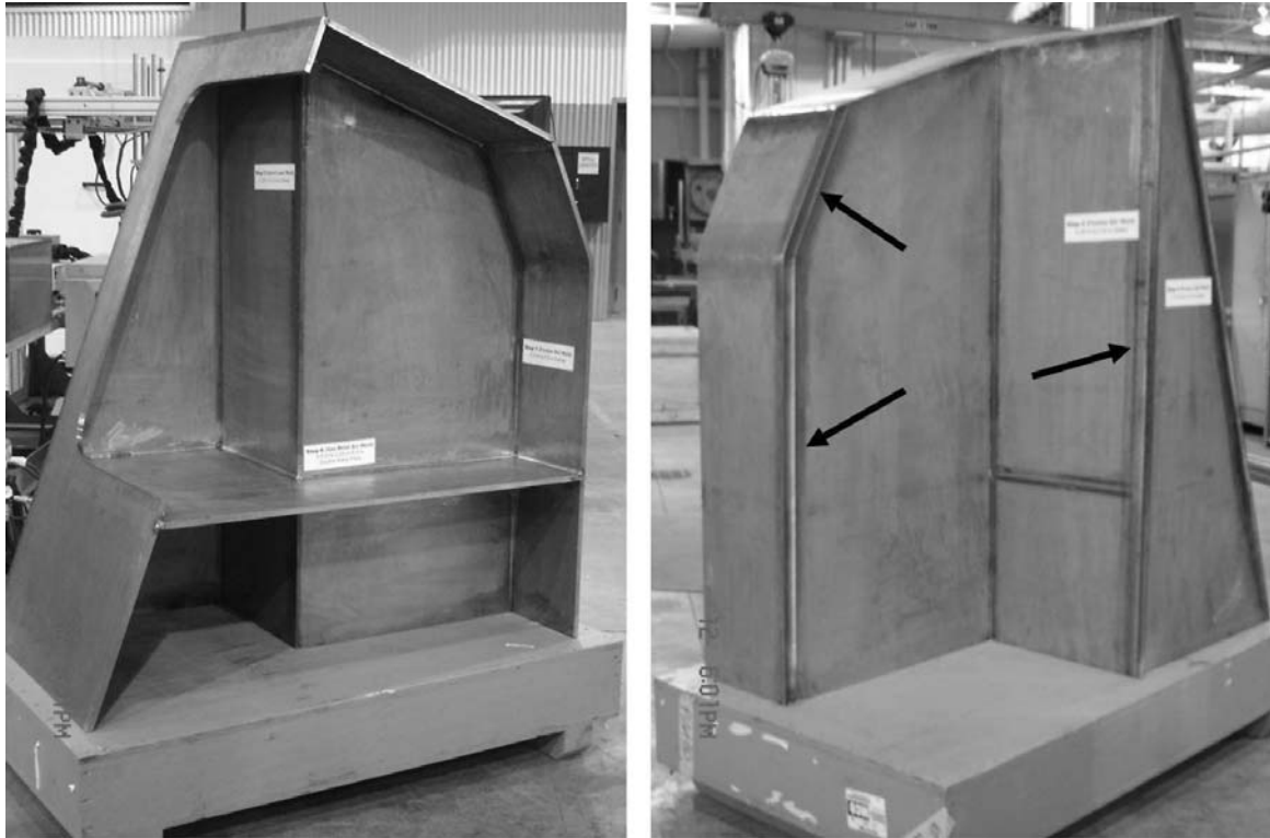
Fig. 13.27 The Edison Welding Institute used a combination of friction stir welding, gas metal arc welding, (GMAW), and hybrid laser welding to fabricate this demonstration article from thick-section titanium plates. Friction stir welding was used to join the 12 mm (0.50 in.) thick plates in a corner joint configuration (arrows) to establish the basic shape of the article, and GMAW and hybrid laser welding were used to complete the assembly. Courtesy of Edison Welding Institute
