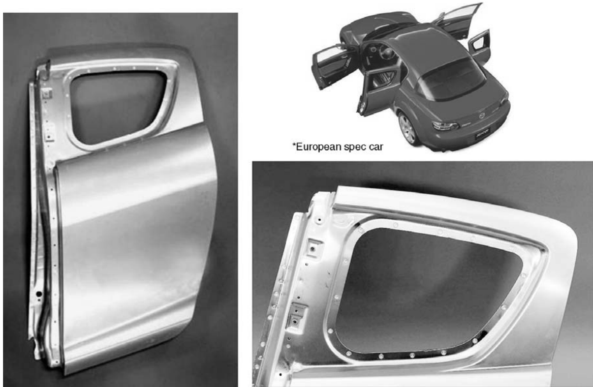
Fig. 13.39 Use of the plunge friction spot welding method on the Mazda RX-8 rear door structure provides for structural stability against side impact and five-star rollover protection at reduced production costs. Courtesy of Ford Motor Company
