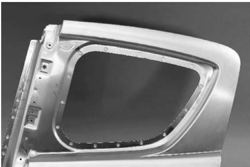
Fig. 12.49 Close-up photo of a completed friction stir spot weld on an RX-8 aluminum rear door. Source: Ref 42
