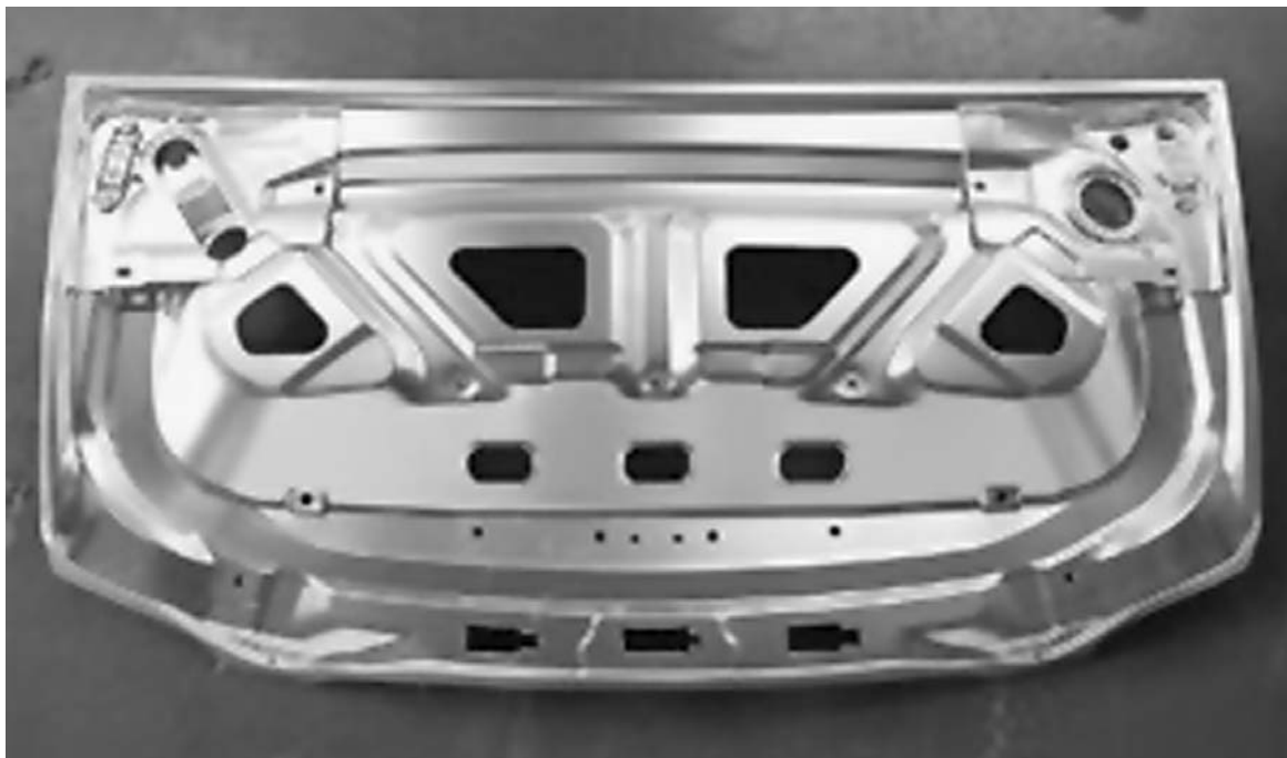
Fig. 12.52 Mazda has used friction welding to join the aluminum deck lid to the steel bolt retainer on the new Mazda MX-5. Source: Ref 47
