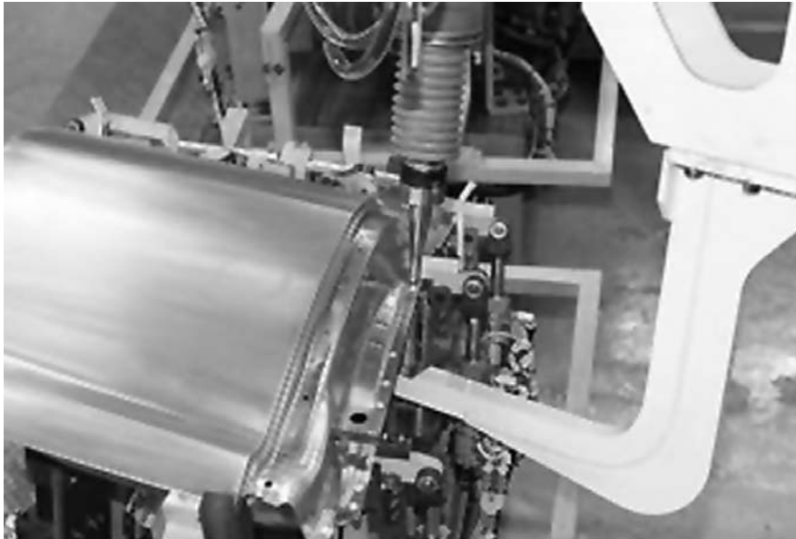
Fig. 12.48 Body panels welded together using friction stir spot welding. Source: Ref 3
