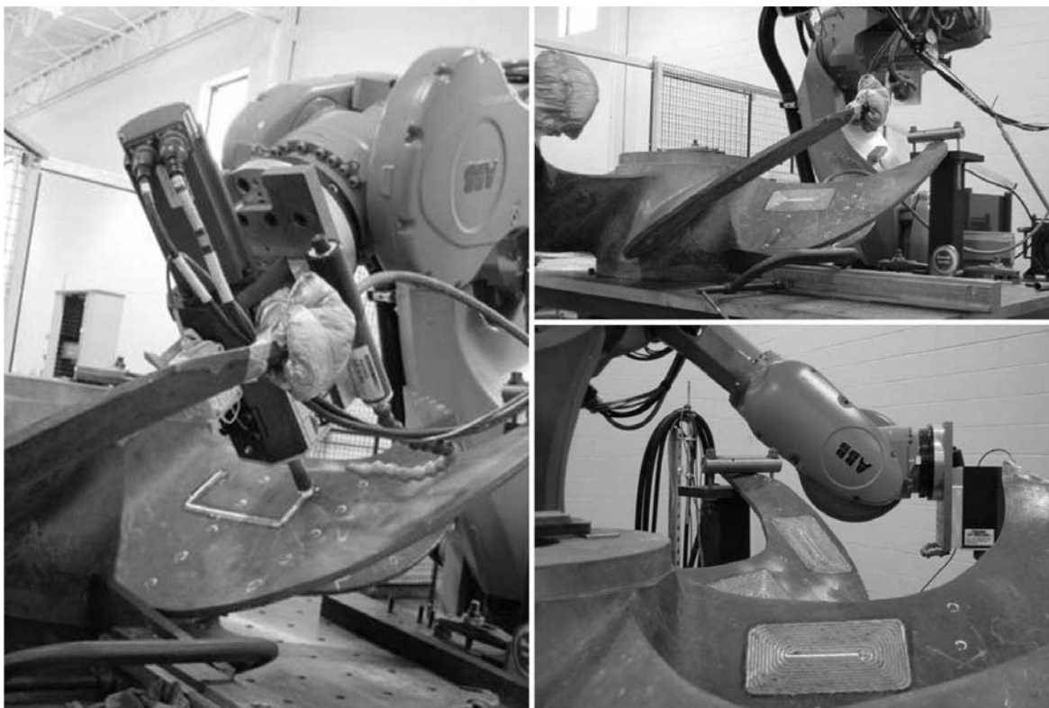
Fig. 13.29 Friction Stir Link, Inc. robotic friction stir weld system processing large areas of NiAl bronze propellers to remove near-surface casting defects. Courtesy of Rockwell Scientific
