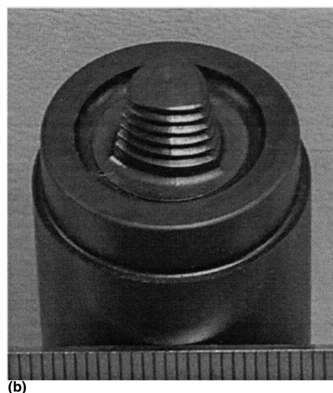
Fig. 2.16 Photos showing details of (a) Trivex and (b) MX Trivex pins. Scale is in millimeters. Source: Ref 93
