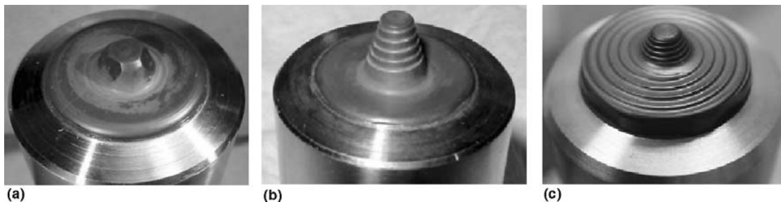
Fig. 6.1 Pin features produced on polycrystalline cubic boron nitride friction stir processing tools, including (a) flats, (b) helical threads, and (c) a combination of convex scrolled shoulder and helical threaded pin
