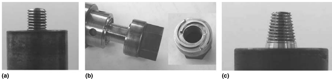
Fig. 13.3 (a) Cylindrical fixed-pin tool, (b) adjustable self-reacting-pin tool, and (c) tapered fixed-pin tool used to join to the aluminum box beam sections
