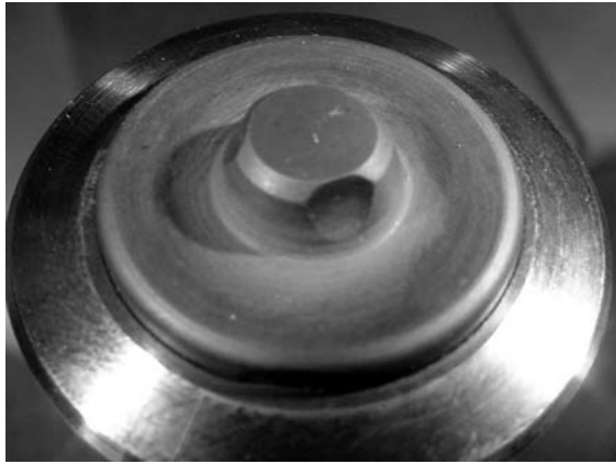
Fig. 2.17 Example of a threadless pin tool. Polycrystalline cubic boron nitride pin tool with three flats at pin tip. Source: Ref 57
