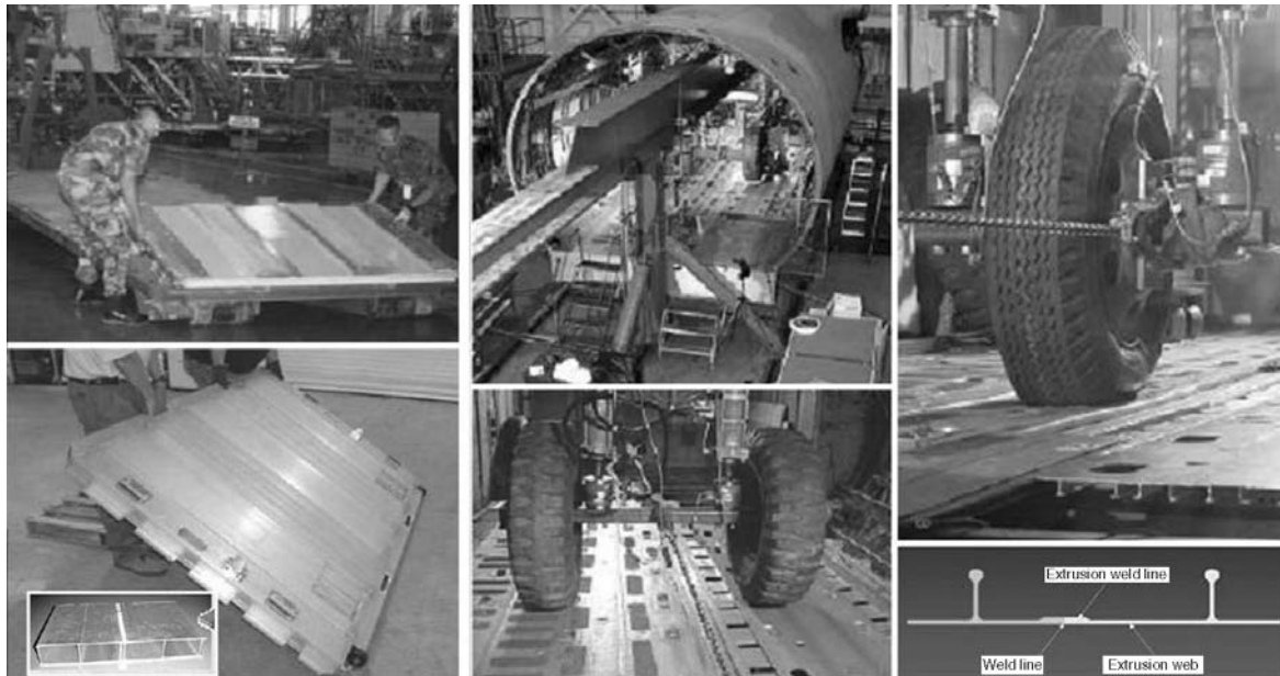
Fig. 13.32 Aircraft hardware items fabricated using friction stir welding under the Air Force Metals Affordability Initiative Program. C-17 cargo ramp (top left) and slipper pallet (bottom left). C-130 cargo floor (right)
