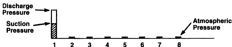
FIGURE 3-35. Condition 1. First pair of rings seals completely.
