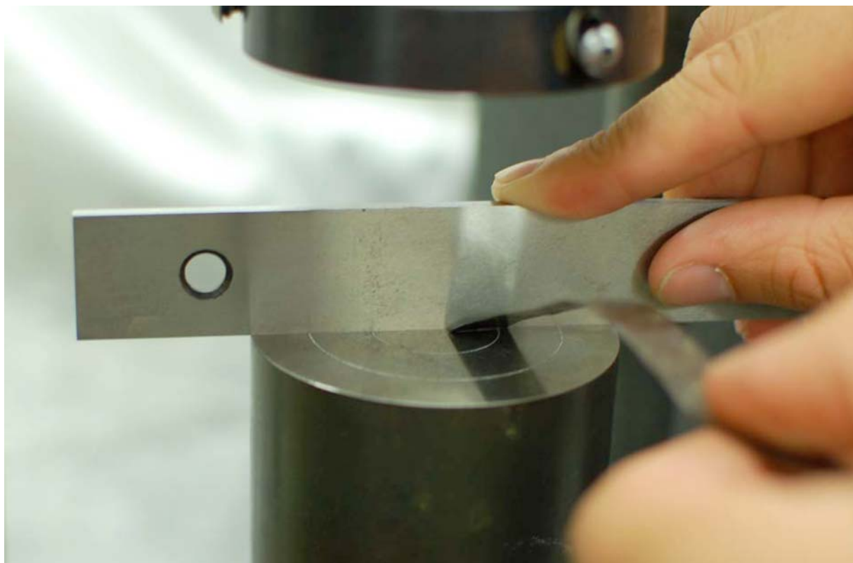
FIG. 2 Determining the Planeness of the Bearing Surface with Machinist Straightedge and 0.001 in. [0.025 mm] Feeler Stock
