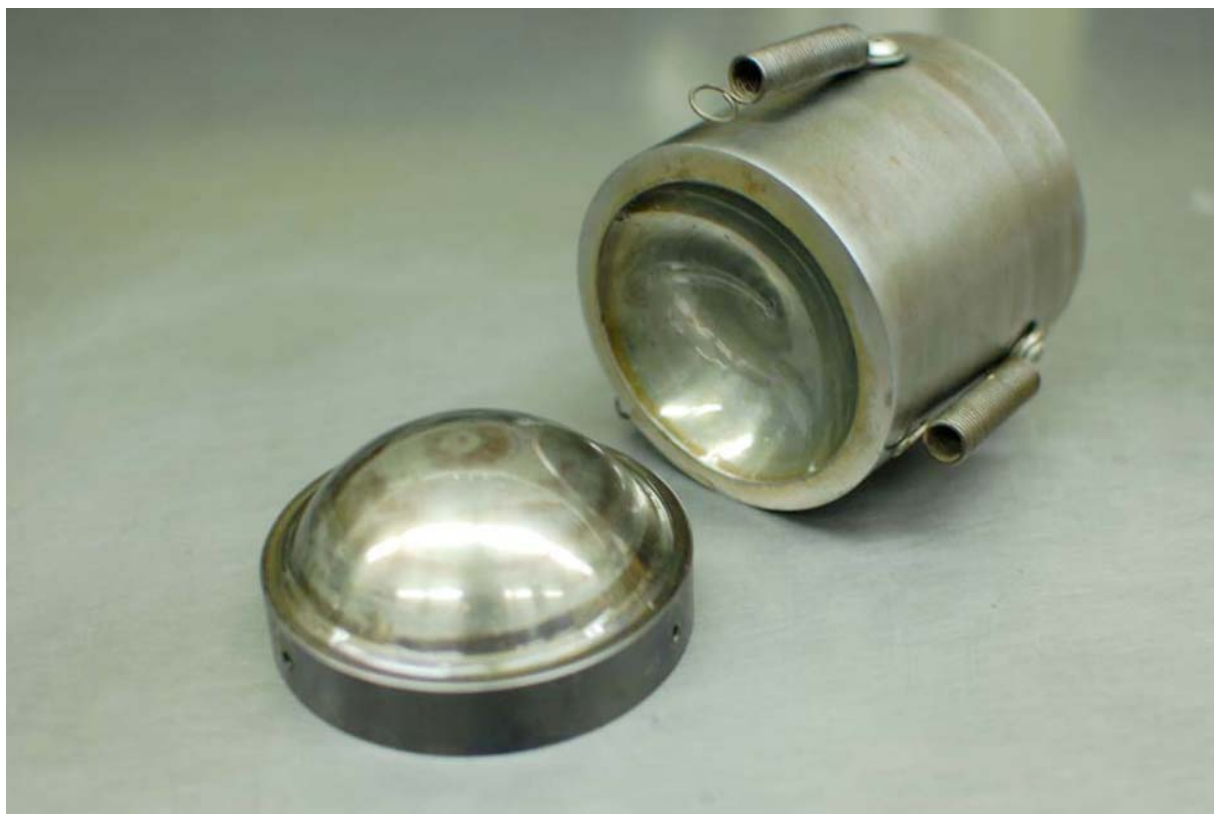
FIG. 3 Disassembled Upper Spherically Seated Bearing Block Displaying the Spherical Portion and Socket Portion of the Bearing Block that Requires Periodic Cleaning and Lubrication
