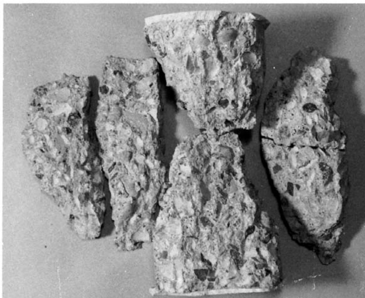
FIG. 2 Typical Conical Fracture Expected in the Compressive-Strength Test
