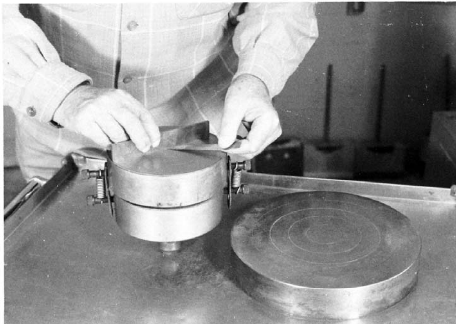
FIG. 4 Checking Planeness of Upper and Lower Bearing Blocks for a Testing Machine Using a Machinist's Parallel and a Feeler Gauge of the Required Thickness
