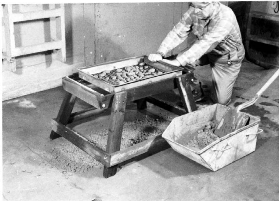
FIG. 5 Equipment for Wet Sieving Concrete by Hand
