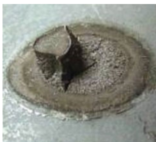
Interfacial Fracture with Button Pull
