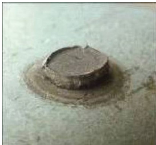
Fig. 4.16 The full button pull indicates acceptable weld quality when testing conventional steels [Source AWS]
