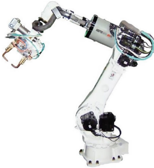
Fig. 3.4 MFDC robotic spot welder [Source T.J. Snow]
