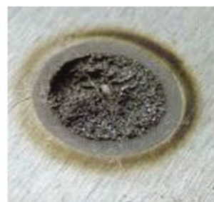
Full Interfacial Fracture
