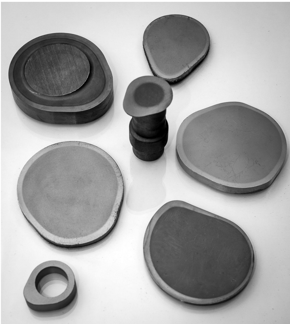
Fig. 10.22 Examples of cam lobe shapes showing nonsymmetrical geometry. Source: Ref 5
