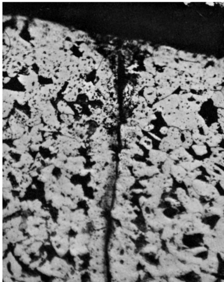
Fig. 9.7 Micrograph of a seam in cross section of a \frac{3}{4} in. diam medium carbon steel bar, showing oxide and decarburization in the seam. 350x. Source: Ref 3
