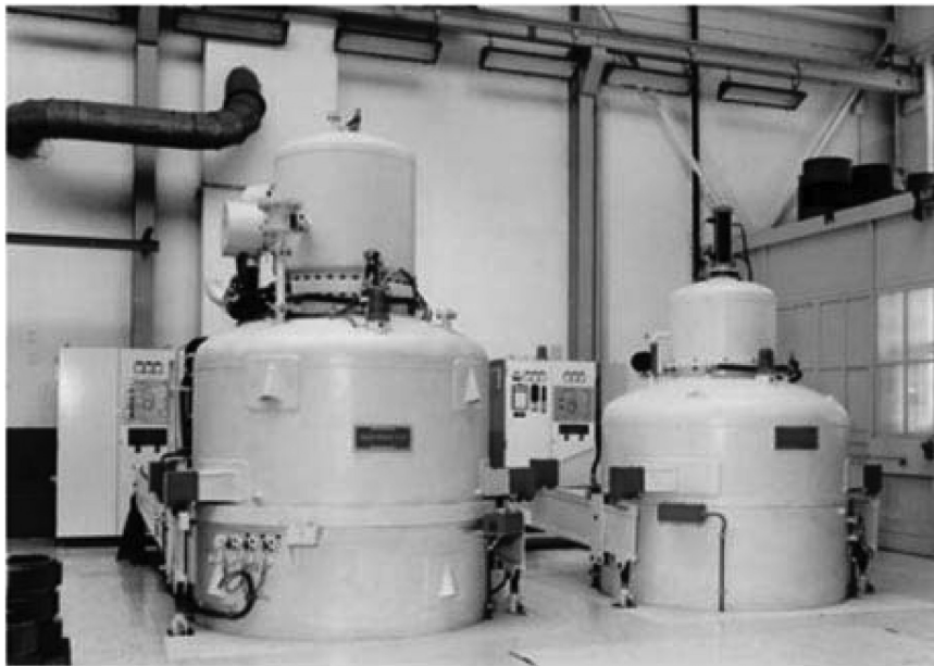
FIGURE 7.10 Typical examples of top-loading vacuum furnaces. (Illustration courtesy of Schmetz GmbH, D-58708, Menden, Germany.)
