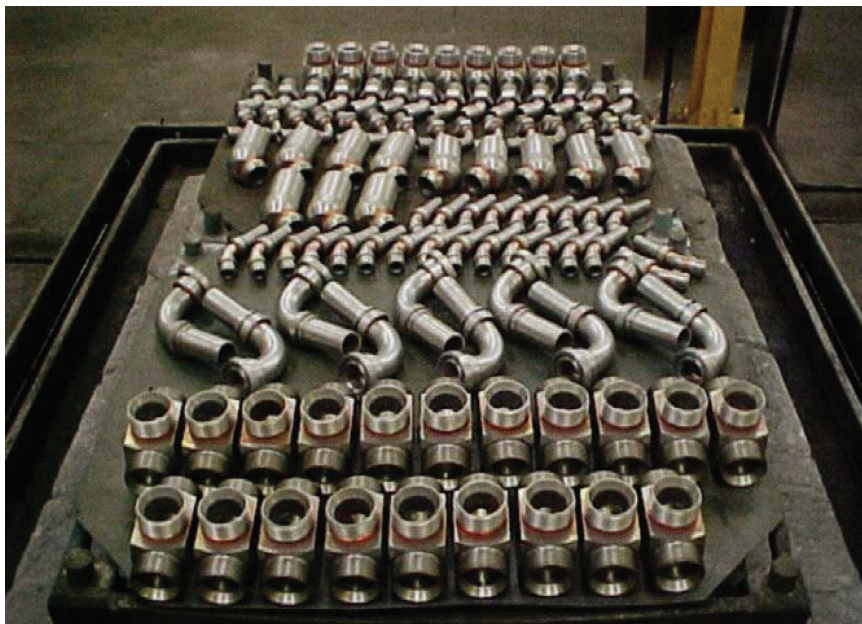
FIGURE 9.15 Hearth of a typical batch-brazing furnace loaded with mild steel parts that have been brazed with pure copper. Note particularly the cleanliness of the surface of the components. (Photograph courtesy of Kepston Limited, Wallsall, England.)
