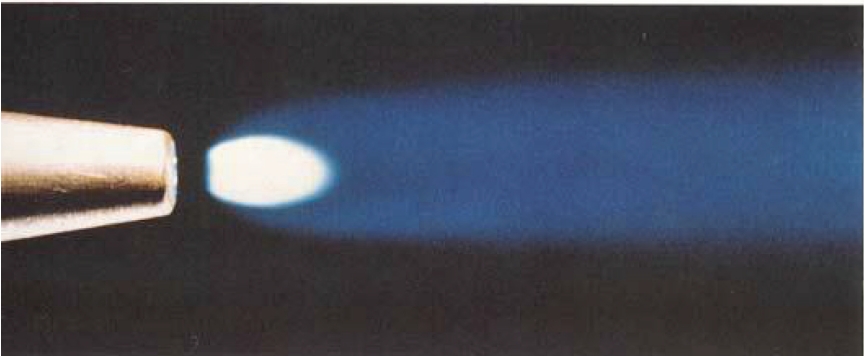
FIGURE 5.10 If the mixture velocity exceeds the burning velocity, flame lift from the torch tip occurs! (Photo courtesy Thessco Limited, Sheffield, UK.)
