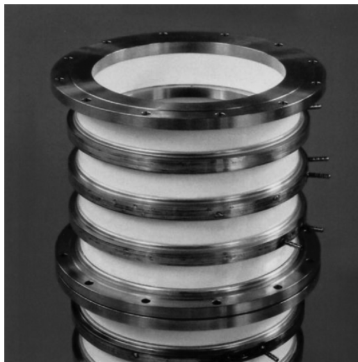
FIGURE 9.3 Technical viability of the brazing of stainless steel to alumina with an active brazing alloy. (Photograph courtesy Umicore AG & Co. KG Business line BrazeTec, Hanau, Germany.)
