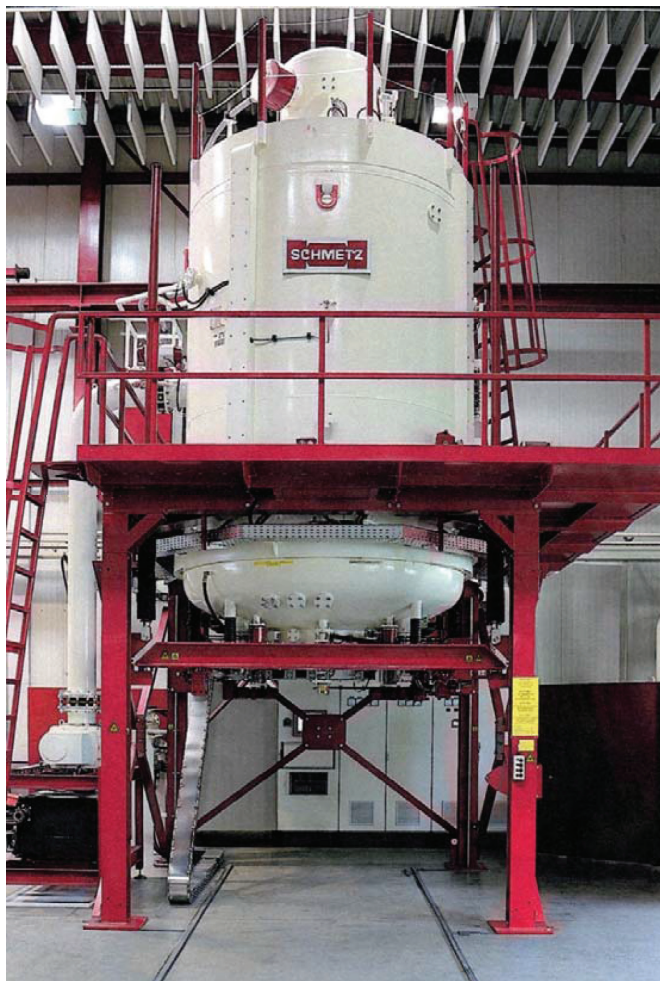
FIGURE 7.9 Good example of a bottom-loading vacuum furnace. (Illustration courtesy of Schmetz GmbH, D-58708, Menden, Germany.)
