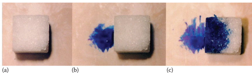
FIGURE 2.5 Diagram of how capillary force will draw ink into a sugar cube. (a) Sugar cube, (b) cube in contact with ink and (c) effect of capillarity.
