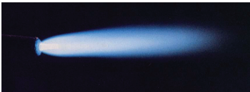
FIGURE 5.13 An increased amount of oxygen has now been mixed with the acetylene. Note particularly how the inner cone is beginning to develop in the flame. While the flame is still acetylene-rich the burning reaction is close to being stoichiometric . (Photo courtesy Thessco Limited, Sheffield, UK.)
