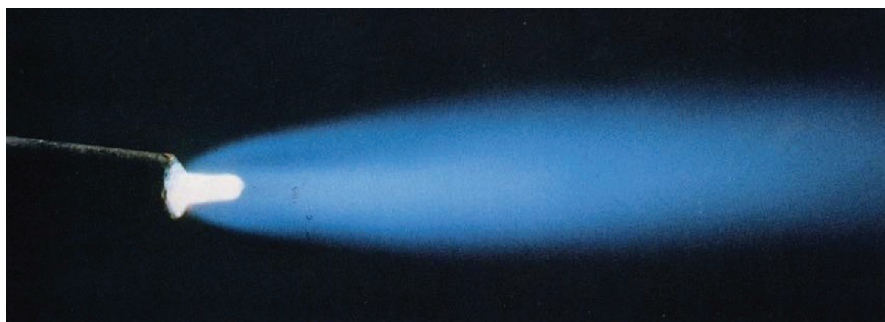
FIGURE 5.14 The reaction is now stoichiometric, and the inner cone of the flame is hard and well defined. The flame is now marginally oxidising, and while it would be suitable for gas-welding processes it is far too hot for brazing. (Photo courtesy Thessco Limited, Sheffield, UK.)
