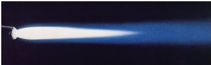
FIGURE 5.12 A modest amount of oxygen has now been mixed with the acetylene. However, the flame is ragged and ill-defined. (Photo courtesy Thessco Limited, Sheffield, UK.)
