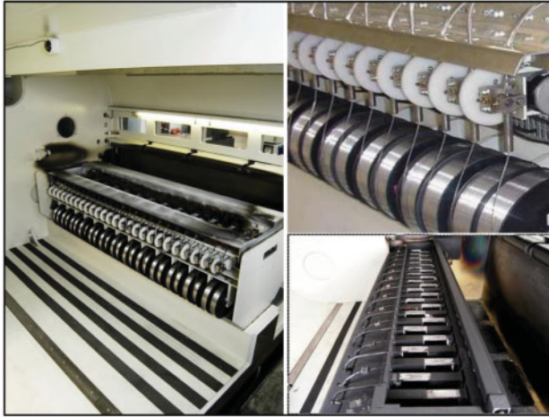
Figure 8.14 Photographs courtesy of General Vacuum Equipment Ltd. showing the inside of an aluminium metallizer. With detail photographs of wire feed system and arrangement of staggered double set of boats.
