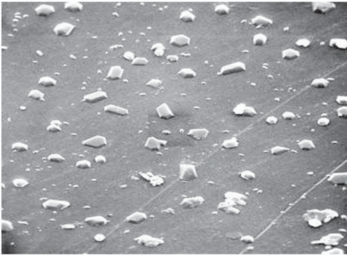
Figure 6.5 Oligomer deliberately grown large by prolonged heating. SEM 2000x magnification.
