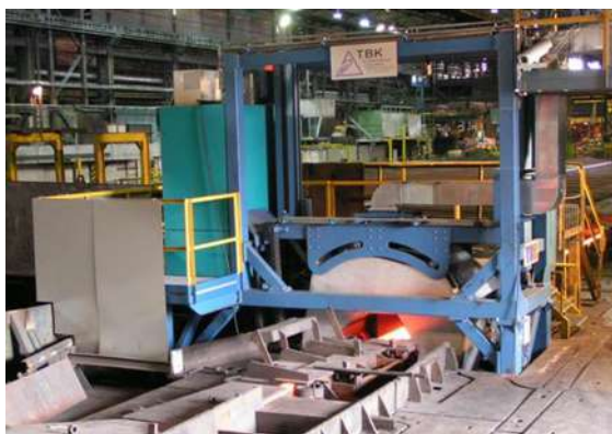
Fig. 7.14 Equipment for hot rail dimensions measurements (TBK)
