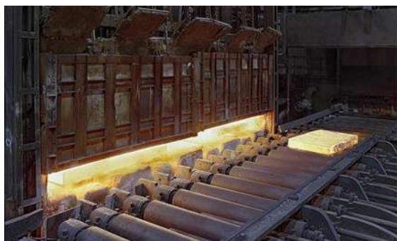
Slab after reheating in walking beam furnace
