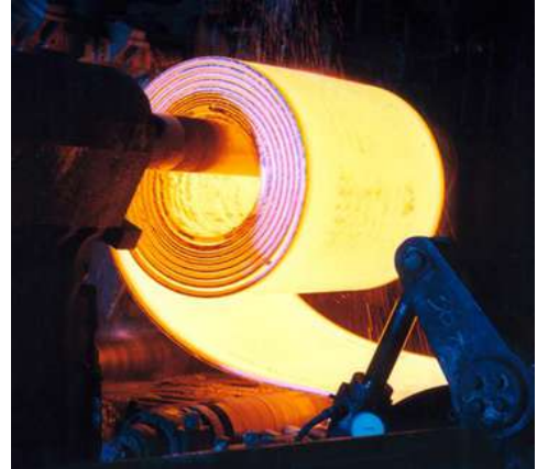
Fig. 2.46 Coilers (cold, hot, furnace coiler)
