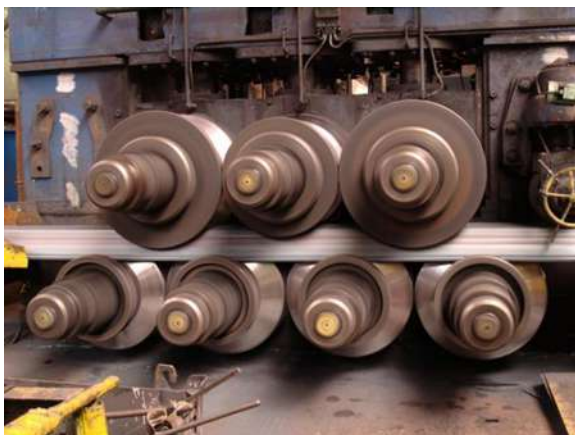
Fig. 7.21 Sheet pile straightening
