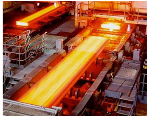
Fig. 4.8 Slab continuous casting with bending of CCS
