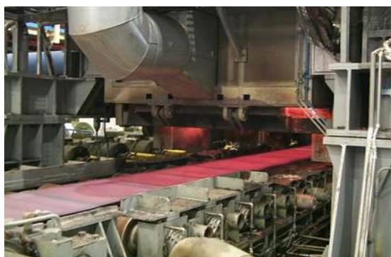
Unequally (inhomogeneously) cooled strip
