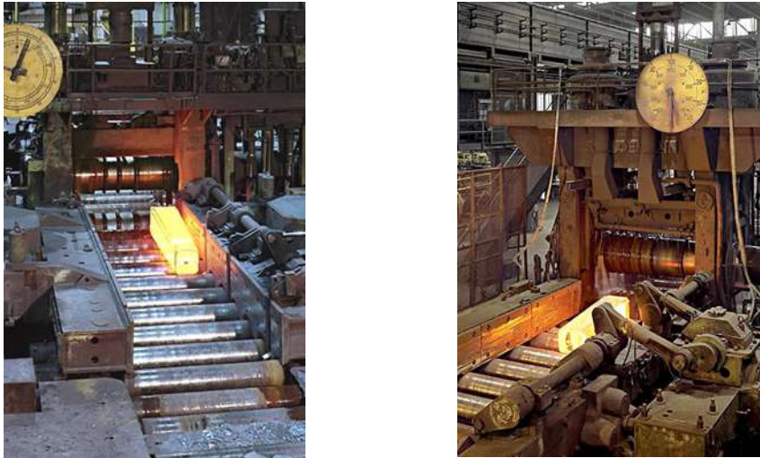
Fig. 4.2 Ingot rolling in blooming
