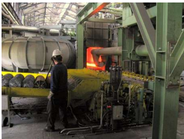
Fig. 14.24 Rotary-hearth furnace – charging of semifinished products in the furnace
