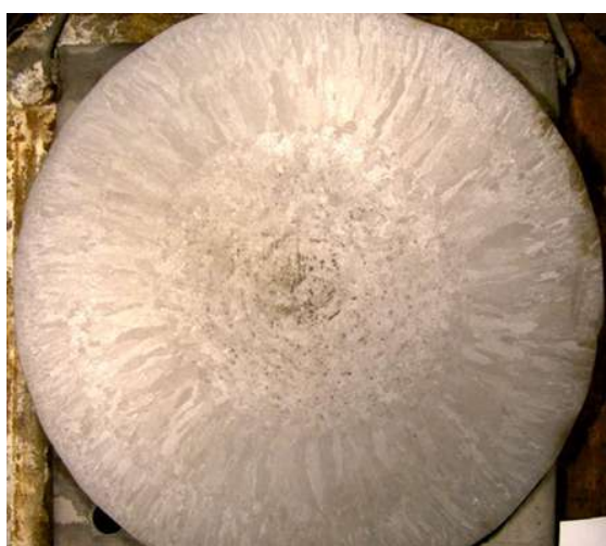
axial shrinkage porosities
