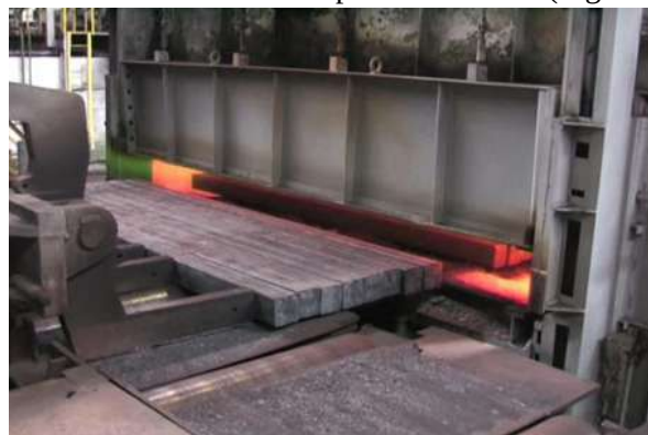
Fig. 7.4 Continuous reheating pusher furnaces of HCC mill
