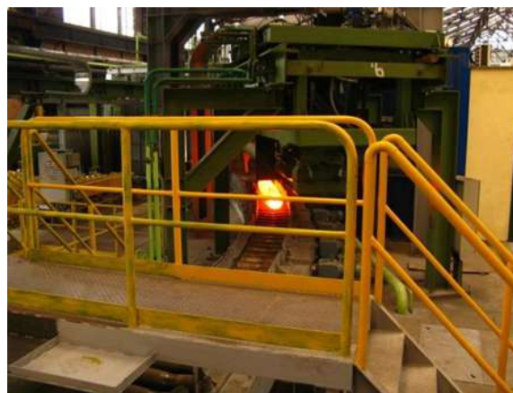
Fig. 14.25 Transport of the semifinished product to the piercing mill
