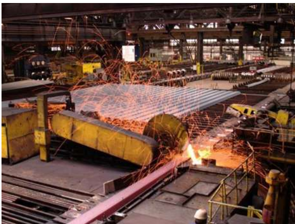
Fig. 7.19 Sheet pile cutting to commercial length
