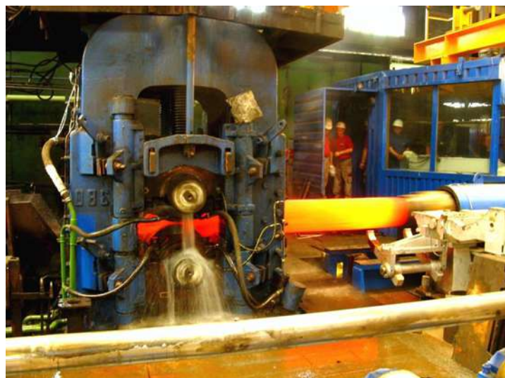
Fig. 14.11 Pilger roll stand – rolls and elongation process
