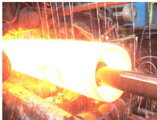
Fig. 1.6 Rolling in piercing mill (seamless tubes)
