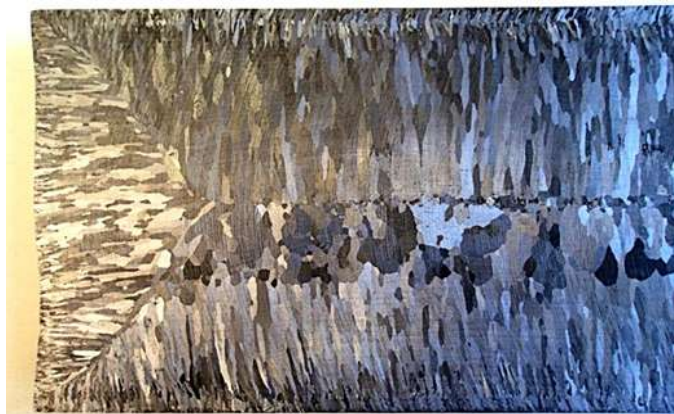
Fig. 4.4 Macrostructure of continuously cast slab with thickness 150 mm (transformer steel with 3 % Si)
