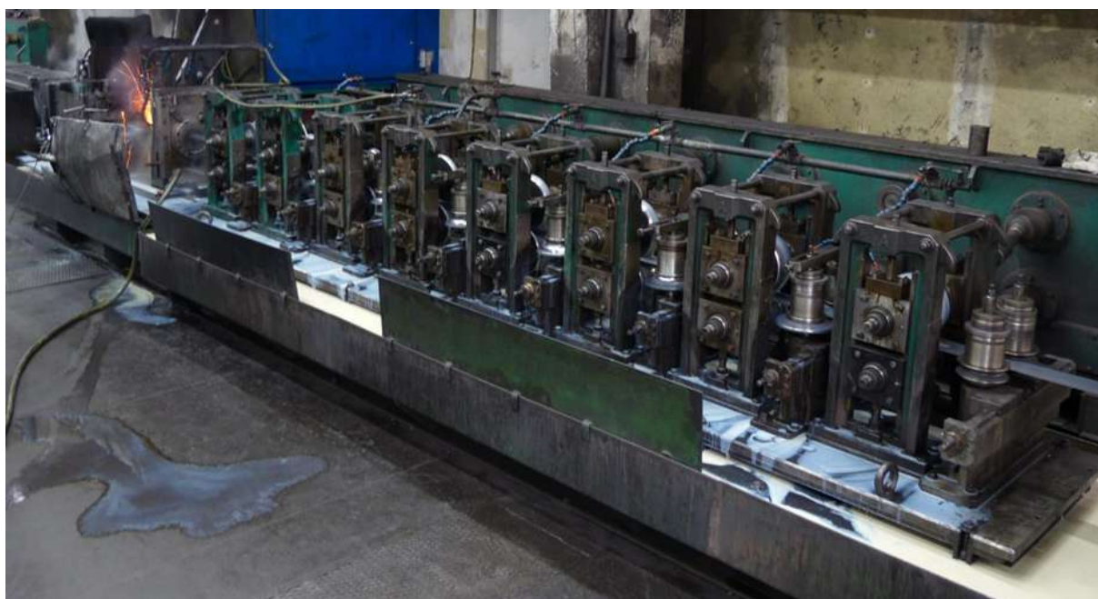
Fig. 13.5 Profiling line for shaping of longitudinally welded tube
