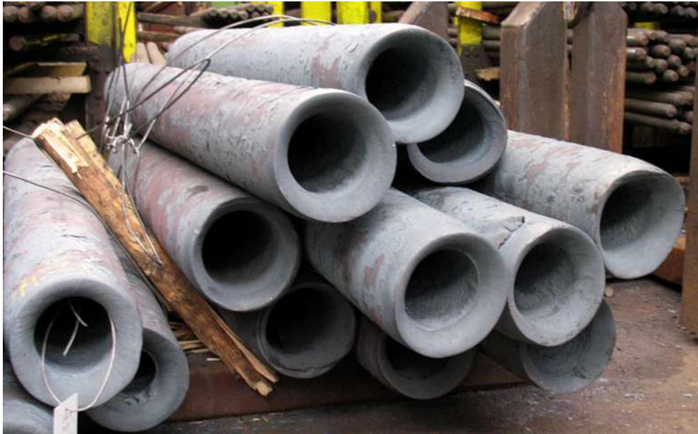
Fig. 14.8 Pierced thick-walled semi-product
