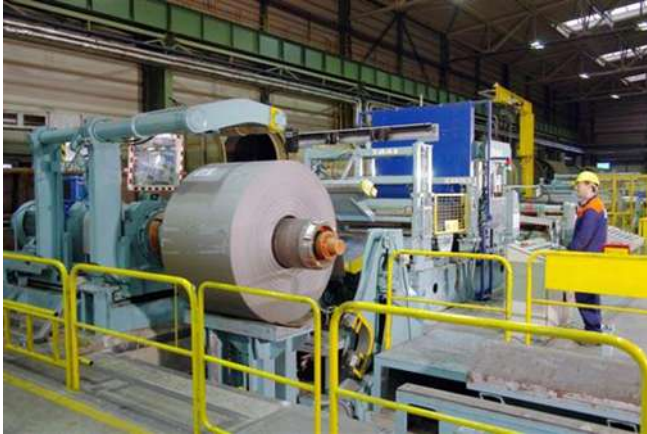
Fig. 2.46 Coilers (cold, hot, furnace coiler)
