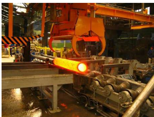
Fig. 14.28 Transport of the thick-walled tube to the pilger mill
