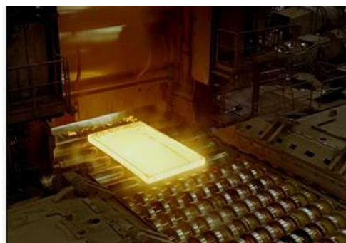
Rolled-out stock of initial slab in plate four-high mill
