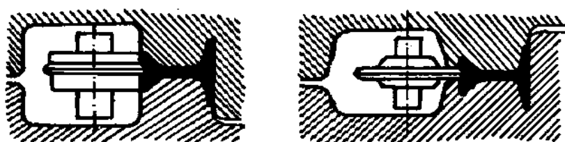
groove before finish rolling
