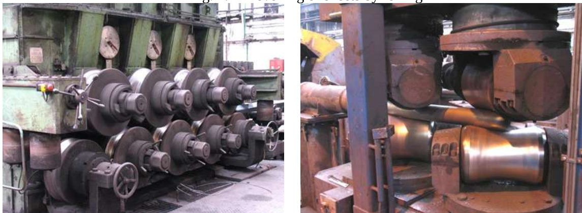
Fig. 2.41 Levelling of sheets by rolling
