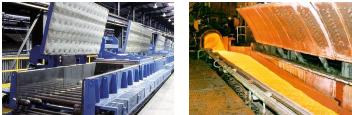
Fig. 7.34 Insulating plates on conveyor Stelmor
