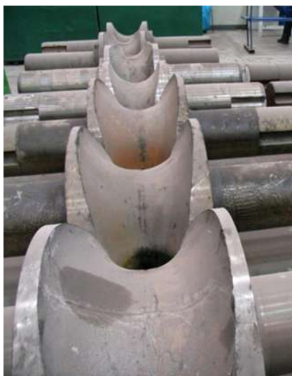
Fig. 14.11 Pilger roll stand – rolls and elongation process
