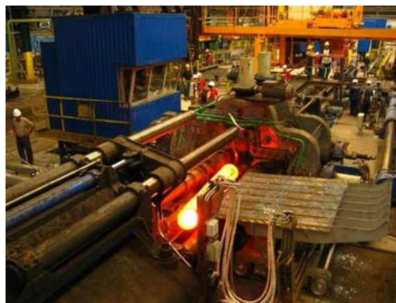
Fig. 14.27 Piercing mill – rear view
