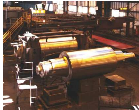
Fig. 5.7 Back-up rolls, front view - “undressed” roll, rear view - roll with chocks and cooling nozzles
