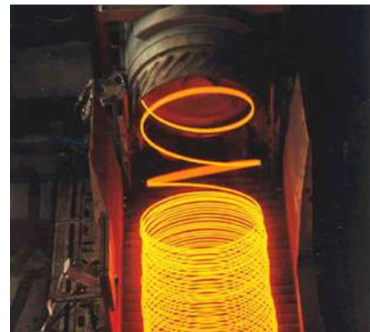
Fig. 7.33 Functional chart of coling equipment Stelmor
