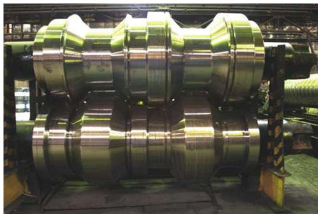
Fig. 7.22 Rolls with two finishing grooves
