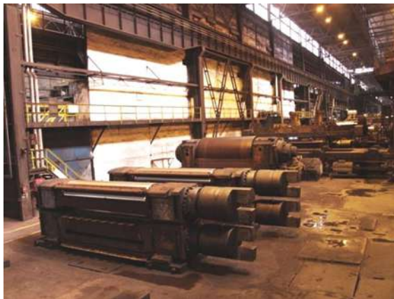
Fig. 5.6 A pair of work rolls with chocks prepared for changing
