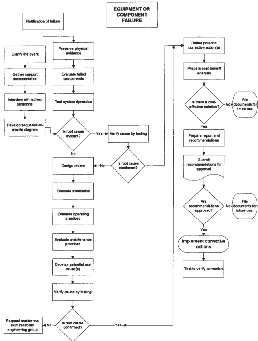
Figure 3-5 Flow diagram for equipment failure investigation.
