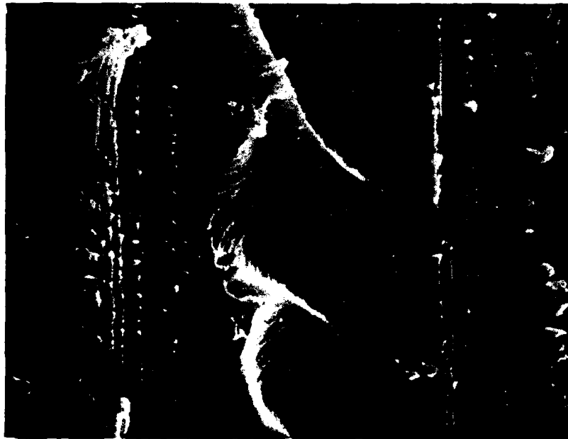
Figure 17 Photomicrograph of Feather Pattern on Mode II Specimen , 5000X
