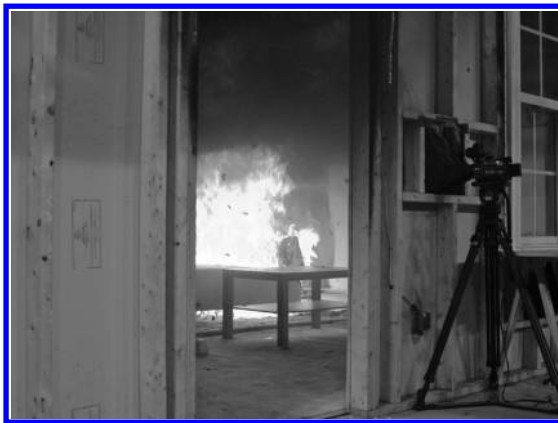
Figure 10.2 Room fire test. (Image courtesy of Jensen Hughes.)
