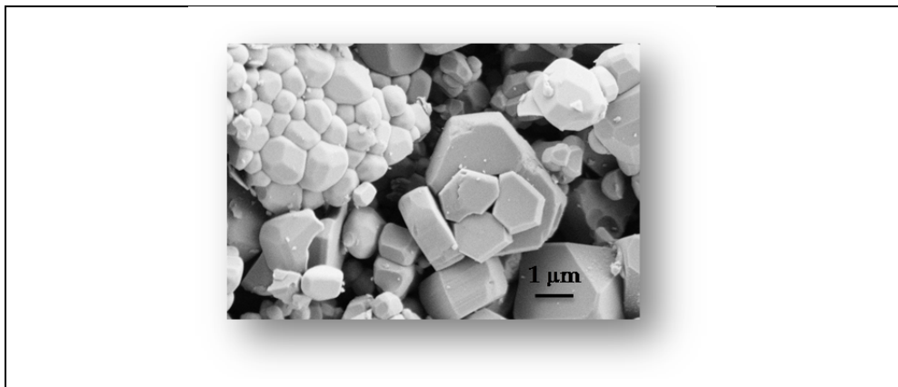
Fig. 13. SEM image of a commercial YAG:Ce powder (Phosphor Tech QMK58/F-U1.).
