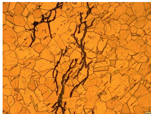
Figure A5: Caustic SCC in CS Base Metal—200X Magnification
