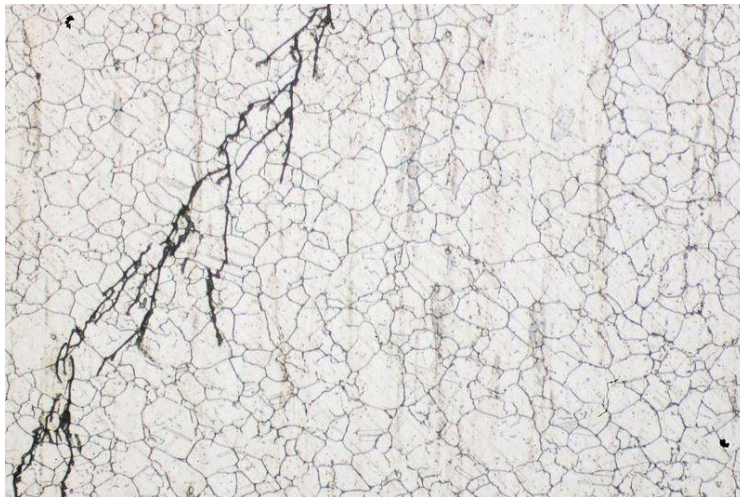
Figure A12: Photomicrograph of Caustic SCC in UNS N08825—Magnification 200X
