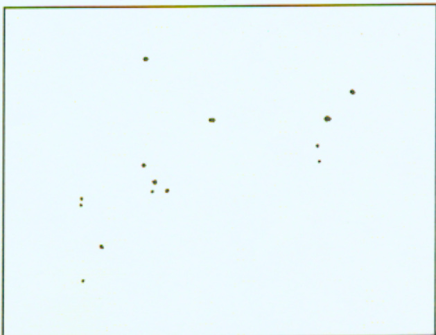
Rust Grade 8-G, 0.1% Rusted
