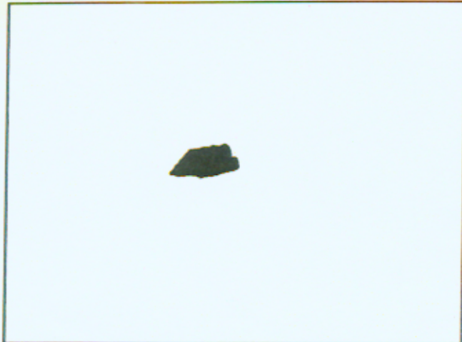
Rust Grade 6-S, 1% Rusted
