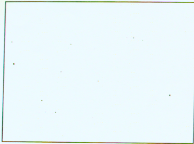
Rust Grade 9-P, 0.03% Rusted
