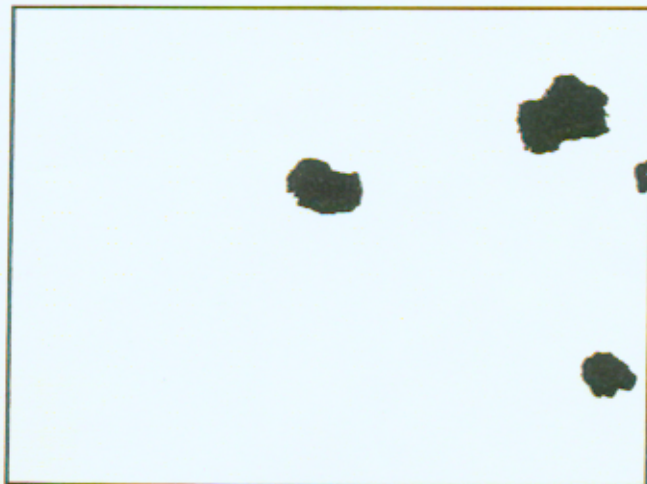
Rust Grade 5-S, 3% Rusted
