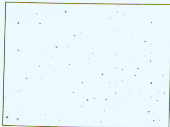
Rust Grade 7-P, 0.3% Rusted
