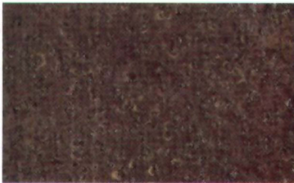
Rust Grade D
