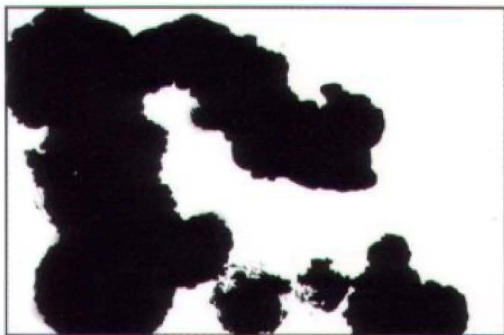
Rust Grade 1-S, 50% Rusted
