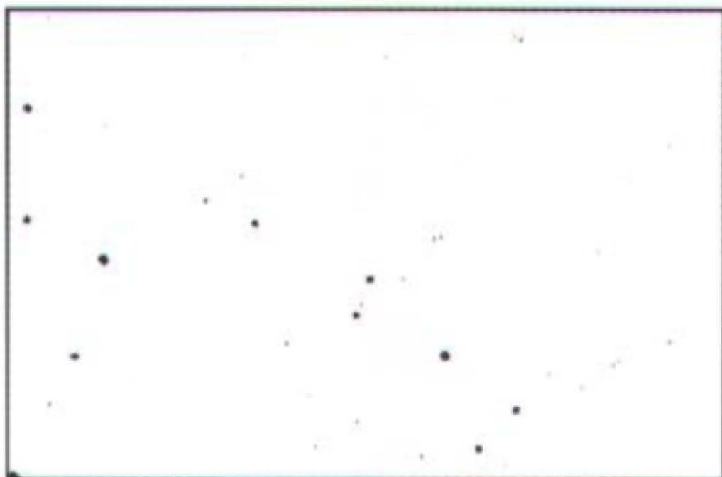
Rust Grade 8-P, 0.1% Rusted
