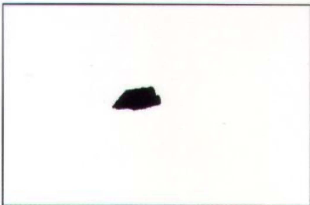
Rust Grade 6-S, 1% Rusted
