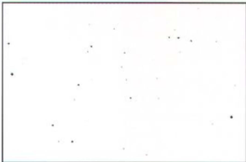
Rust Grade 9-P, 0.03% Rusted
