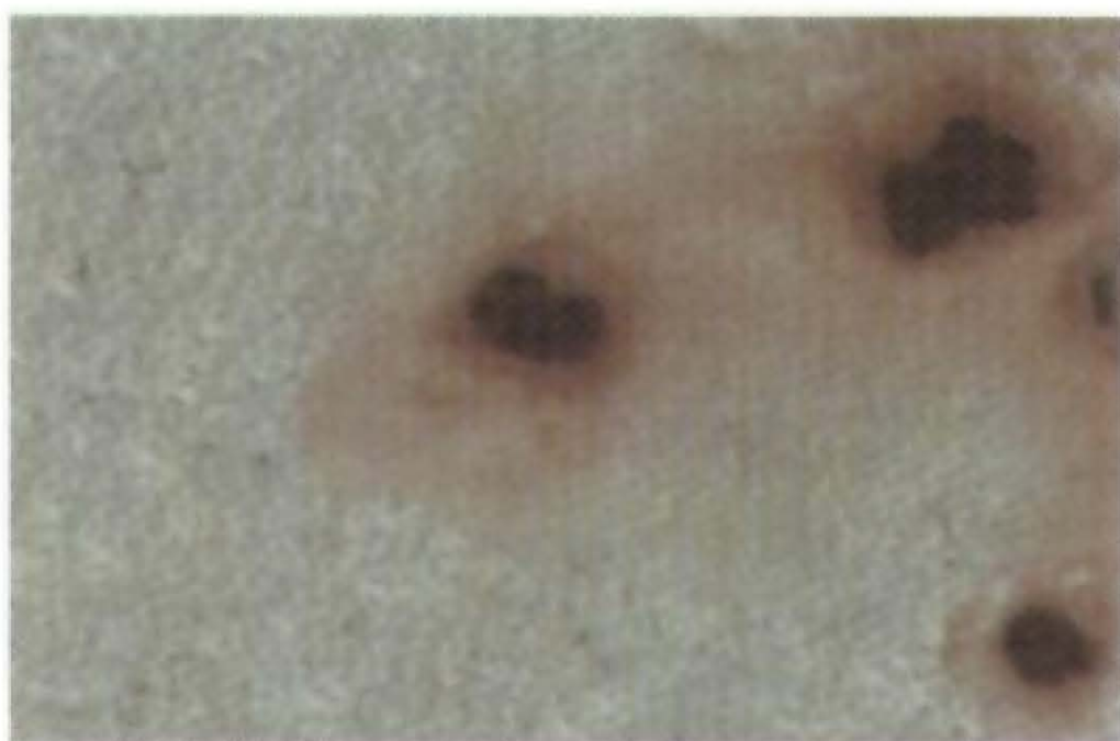
Rust Grade 5-S, 3% Rusted
