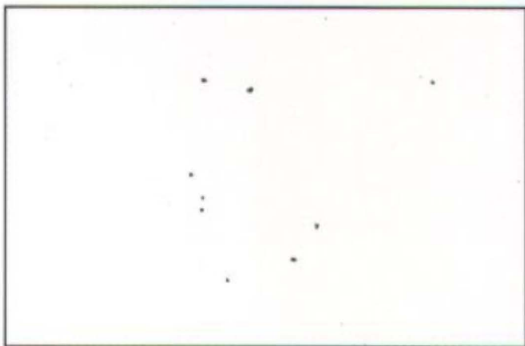
Rust Grade 9-G, 0.03% Rusted
