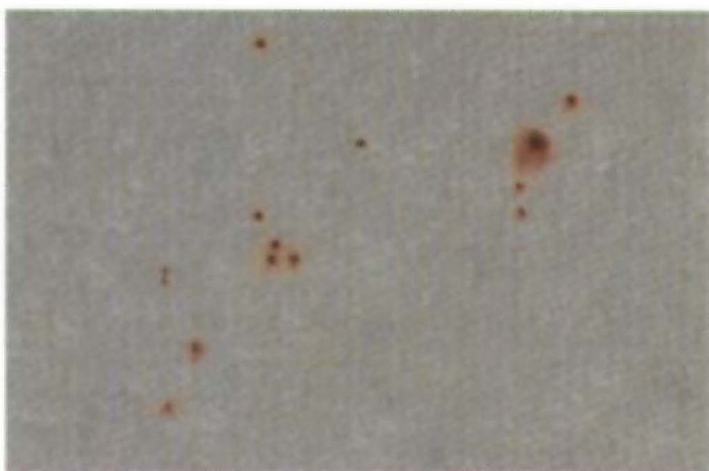
Rust Grade 8-G, 0.1% Rusted
