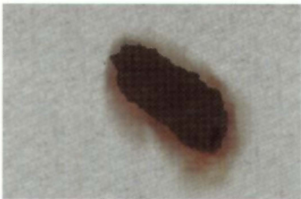
Rust Grade 4-S, 10% Rusted
