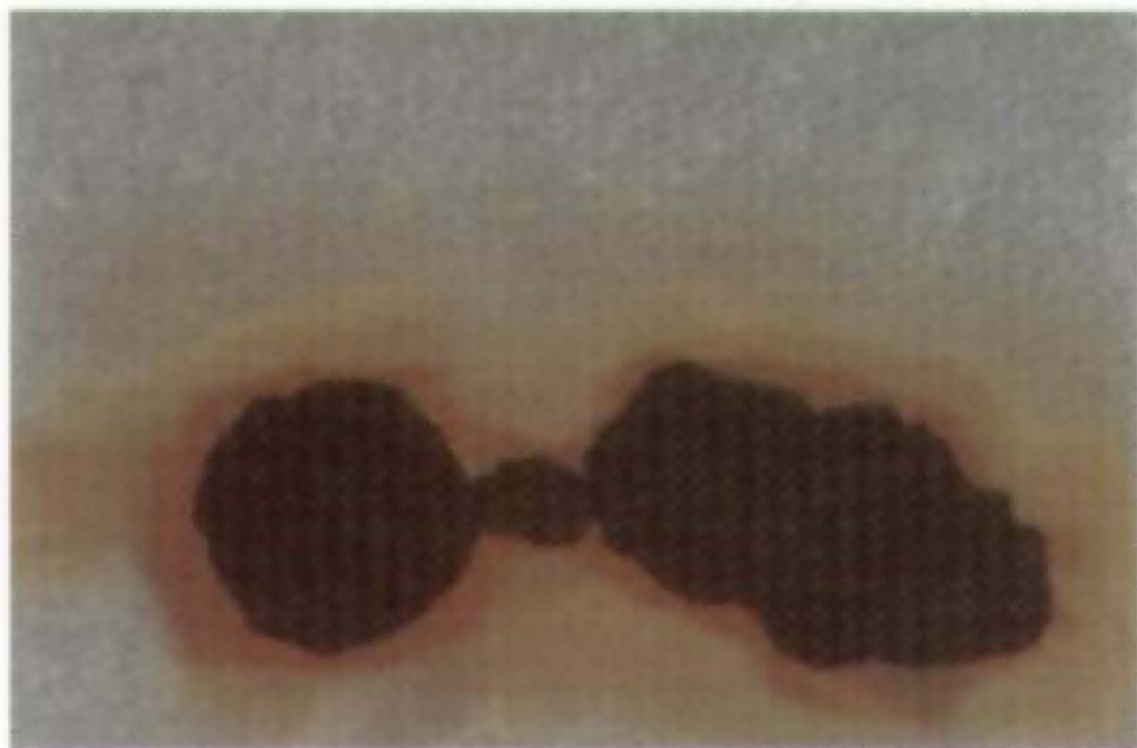
Rust Grade 3-S, 16% Rusted
