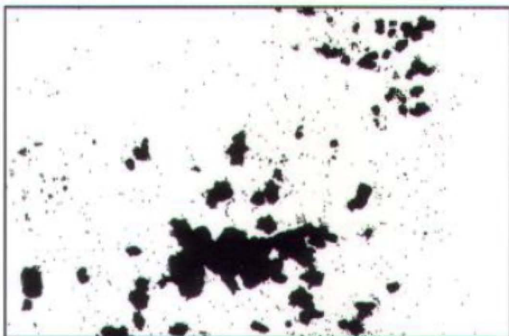
Rust Grade 4-G, 10% Rusted
