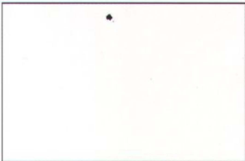
Rust Grade 9-S, 0.03% Rusted
