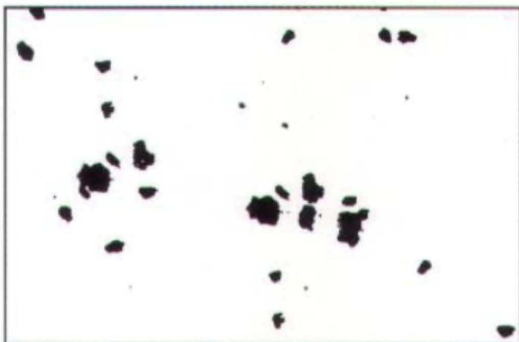
Rust Grade 5-G, 3% Rusted
