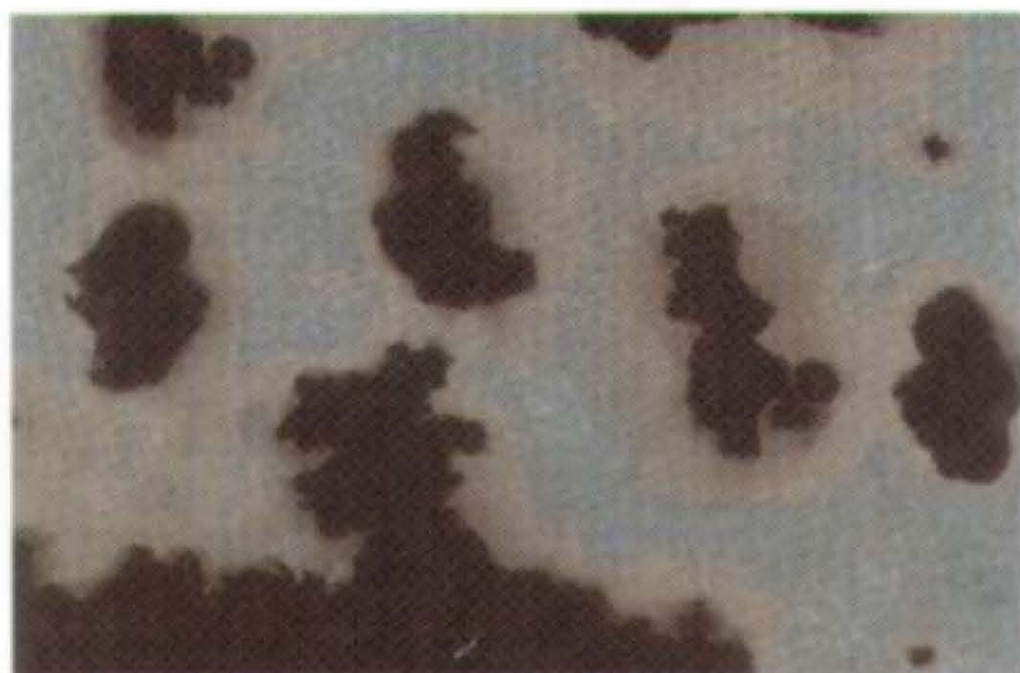
Rust Grade 2-G, 33% Rusted
