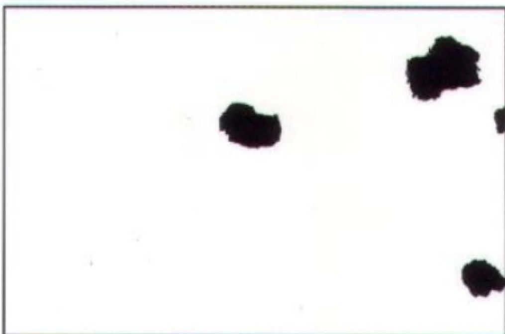
Rust Grade 5-S, 3% Rusted
