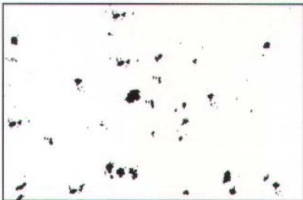
Rust Grade 6-G, 1% Rusted
