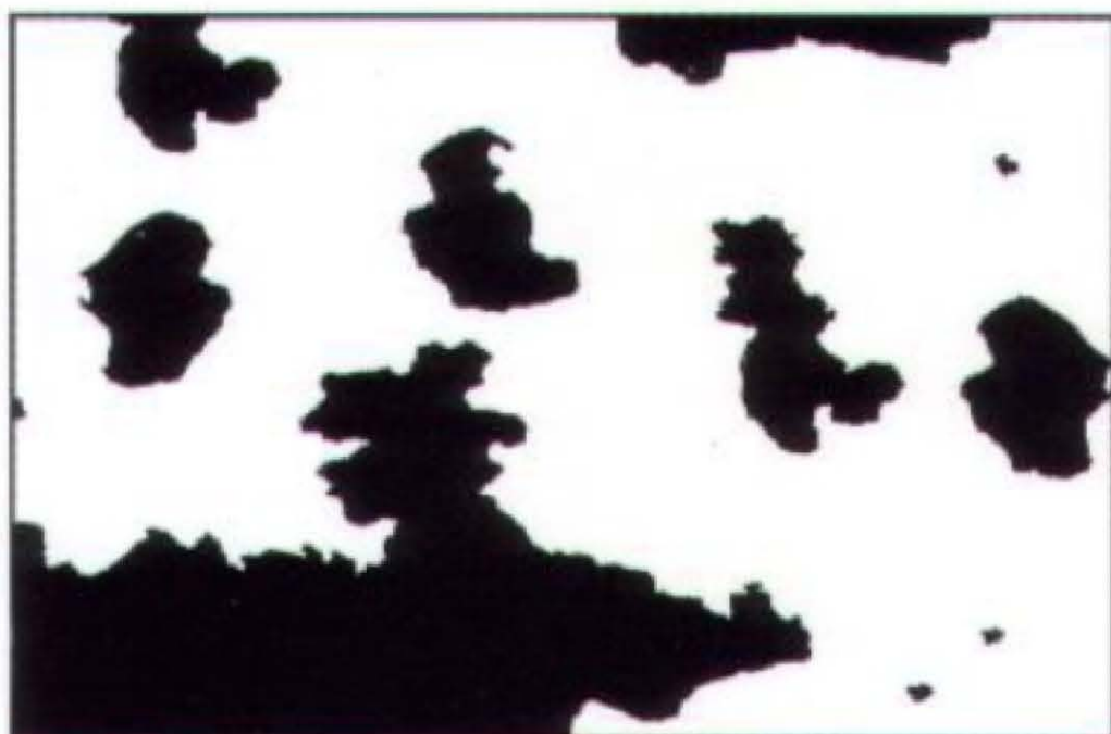
Rust Grade 2-G, 33% Rusted
