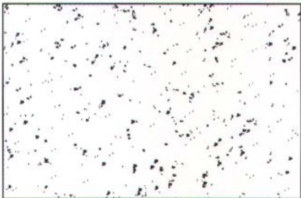
Rust Grade 6-P, 1% Rusted
