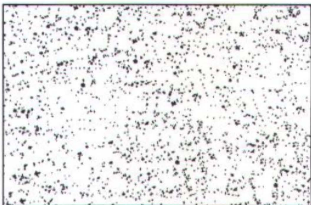
Rust Grade 5-P, 3% Rusted
