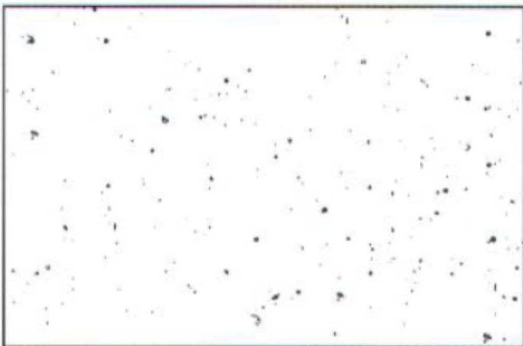
Rust Grade 7-P, 0.3% Rusted
