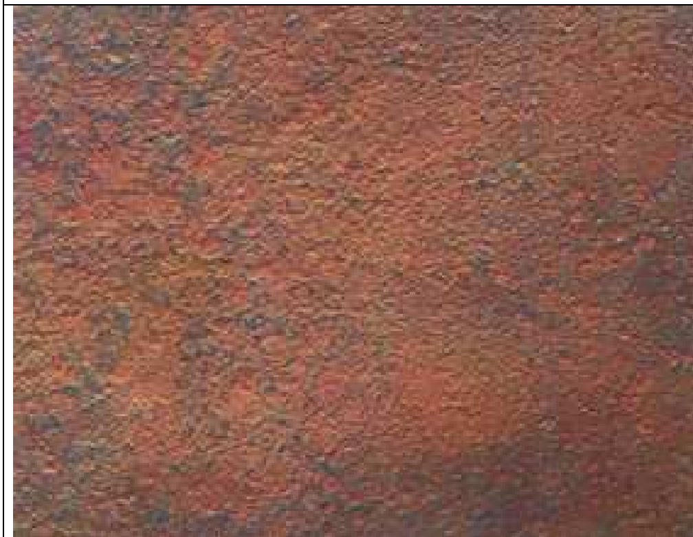
D St 2 - hand tool cleaning
