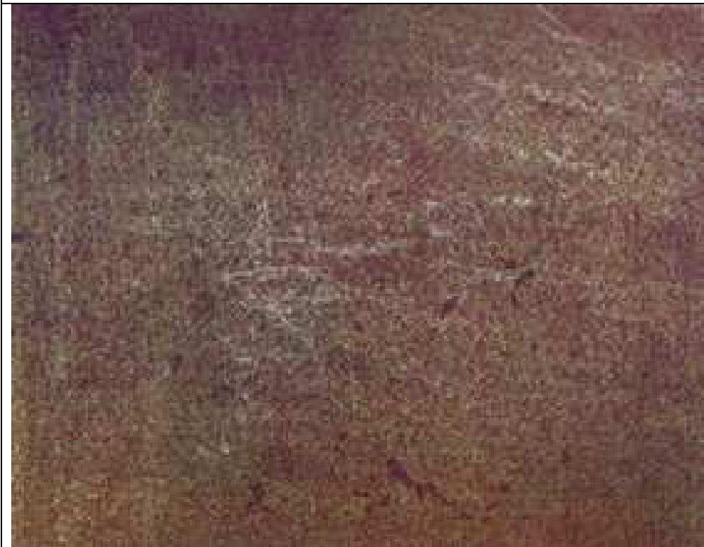
C St3 - power tool cleaning
