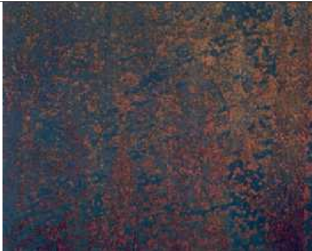
B St 2 - hand tool cleaning
