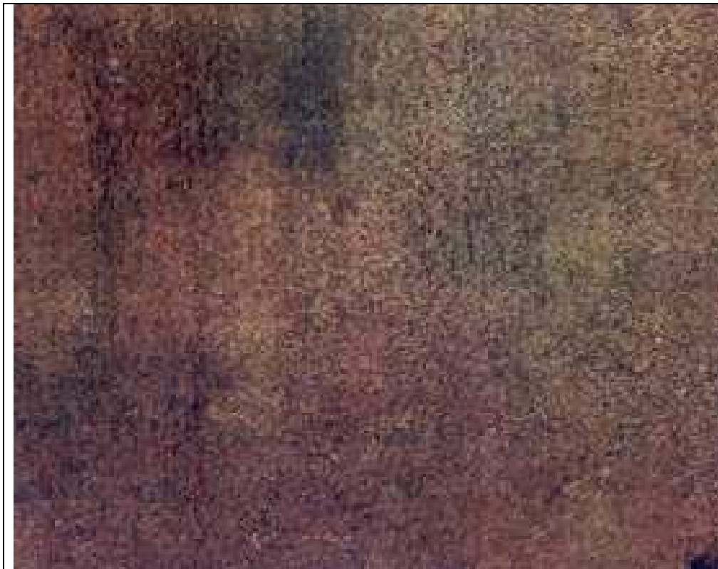
C St 2 - hand tool cleaning
