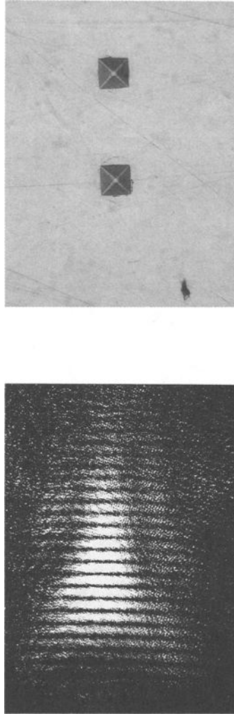
FIG. 2—Photomicrograph of a set of indentations and photograph of an interference fringe pattern. The centers of the indentations are 100\text{ }\mu\text{m} apart.
