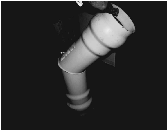
FIG. 2—Forty-five-degree elbow, female-by-female, with BullDog restraint mechanism.
