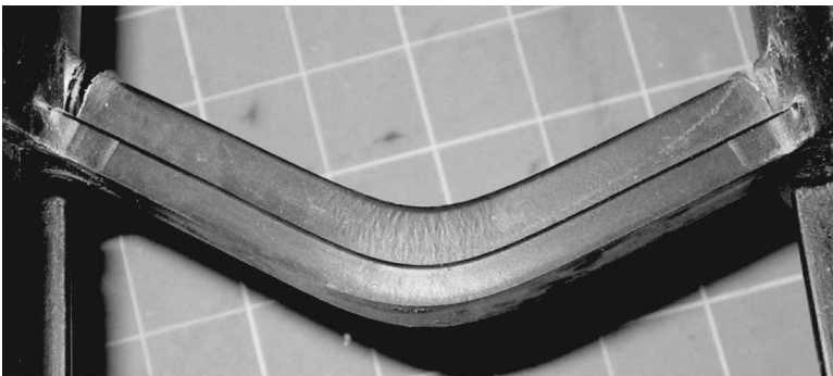
FIG. 6—Brittle fracture at ends of buckled strut.
