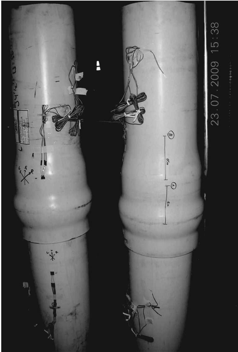
FIG. 5—Strain gage rosettes attached to specimens collected strain data.
