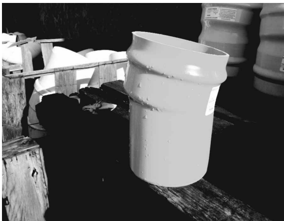
FIG. 1—Five-degree, male-by-female, bend.
