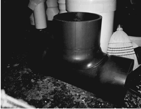
FIG. 6—A spout has been thermoformed over the stiffener.
