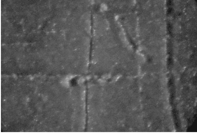
FIG. 9—Cracks seen in CPVC pipe specimen HB after only 42 hours of contact with a quaternary ammonium salt, 250 \times magnification.
