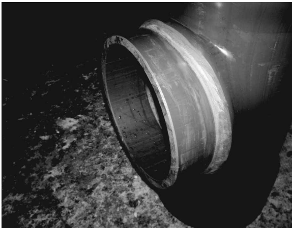
FIG. 5— Pulled hole with stiffener.
