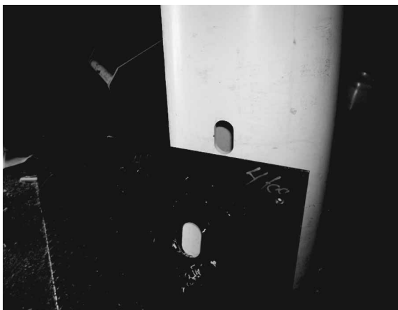
FIG. 3—Hole routed into 16-in. running leg. The hole will later be thermoformed into a pulled hole.
