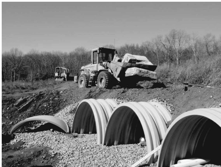
FIG. 7—Live-load testing of chambers and end caps.
