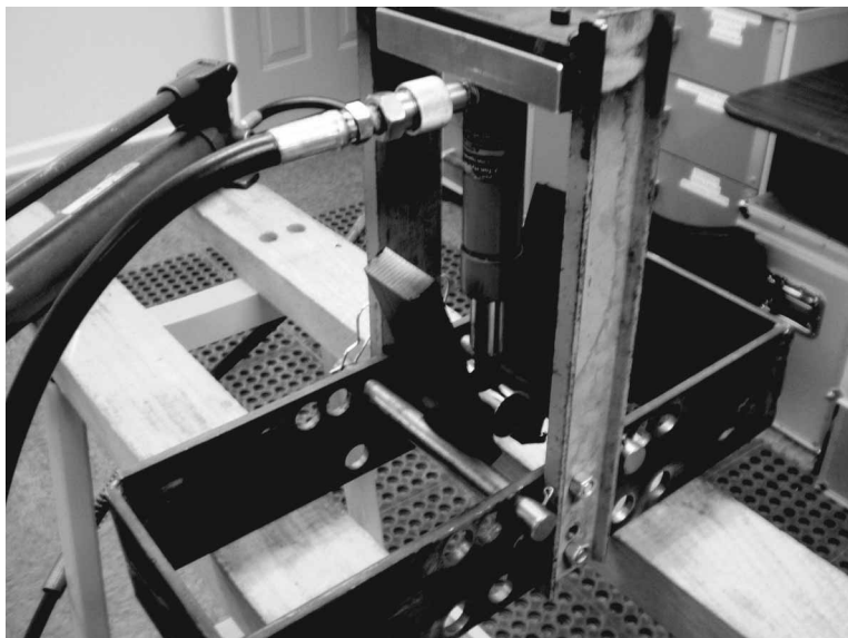
FIG. 10—GSB test apparatus with failed test result.
