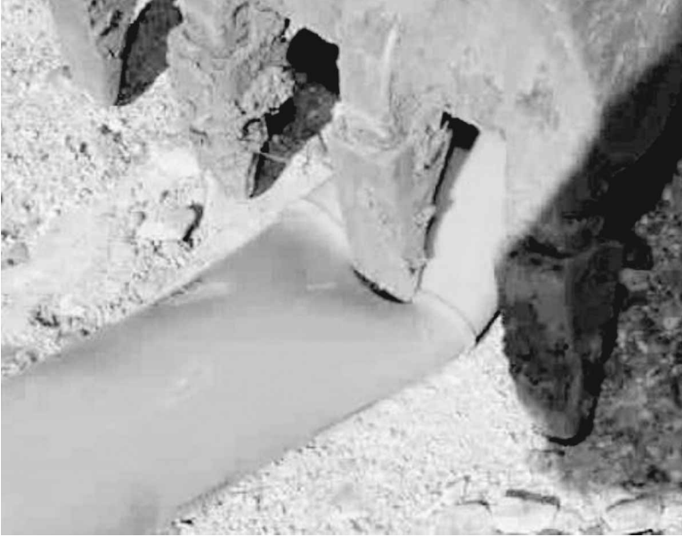
FIG. 13— Close-up of backhoe tooth impingement.
