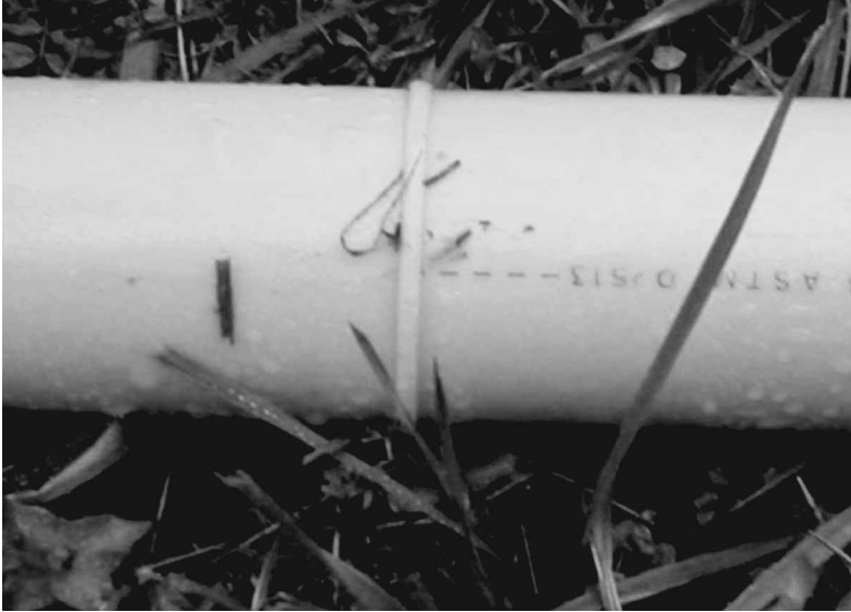
FIG. 6—Typical butt fusion joint in 2 NPS PA-11 piping.
