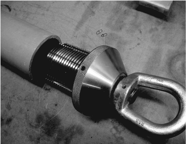
FIG. 6—End grip used for a 4 in. specimen.
