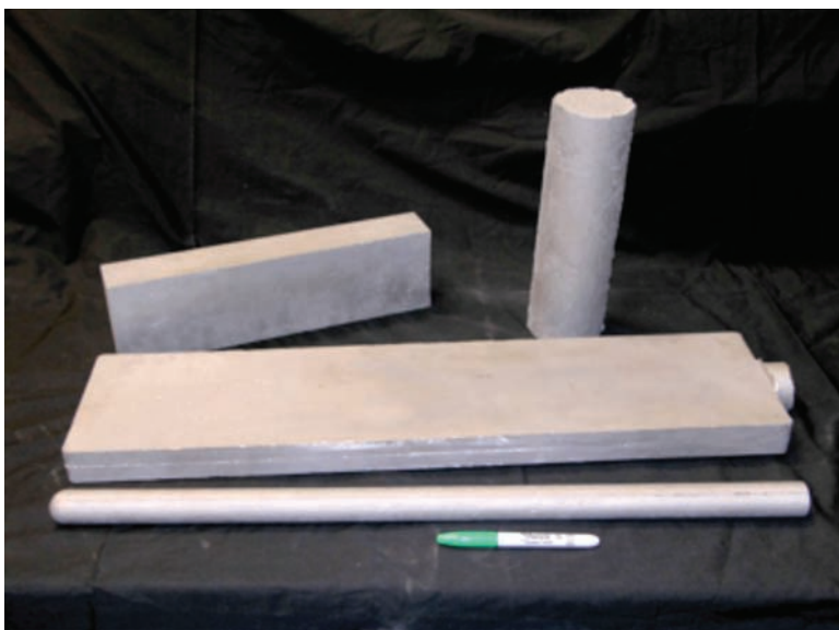
FIG. 2—60NiTi cast ingots from which test specimens were fabricated.
