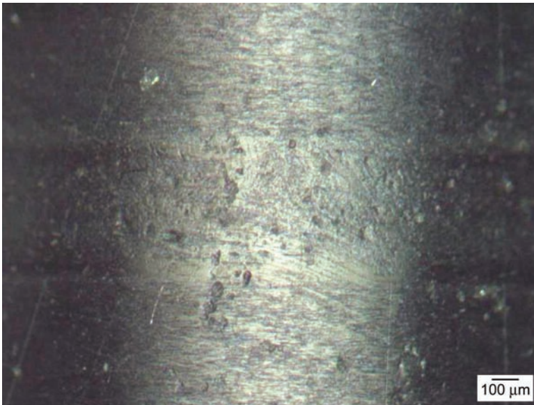
FIG. 7—Wear track surface following RCF test at 360 ksi; no failure observed.
