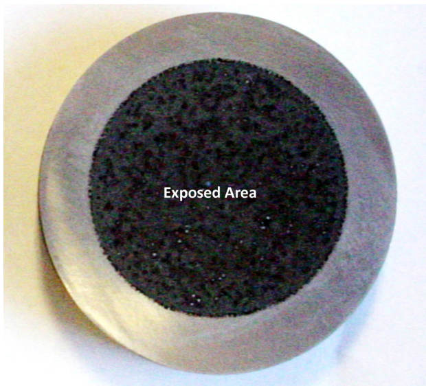
FIG. 1 ASTM D4340 hockey-puck-shaped specimen.
