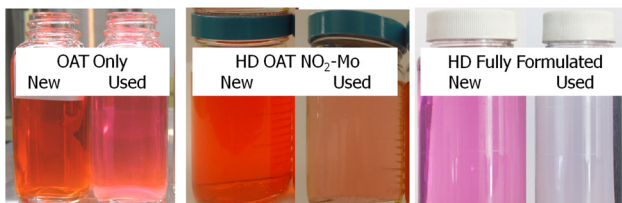
FIG. 9 Coolant color change after exposure to post-brazed aluminum heat exchanger tubes.
