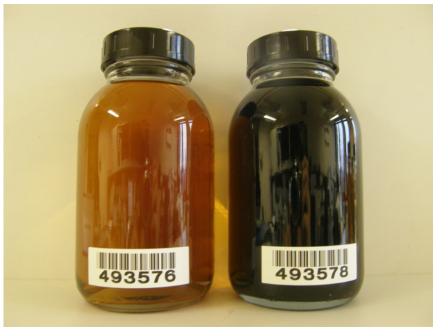
FIG. 3 Visual appearance of Coolant A and Coolant B after the high temperature oxidation test in the presence of a cast iron ring (left Coolant A / right Coolant B).
