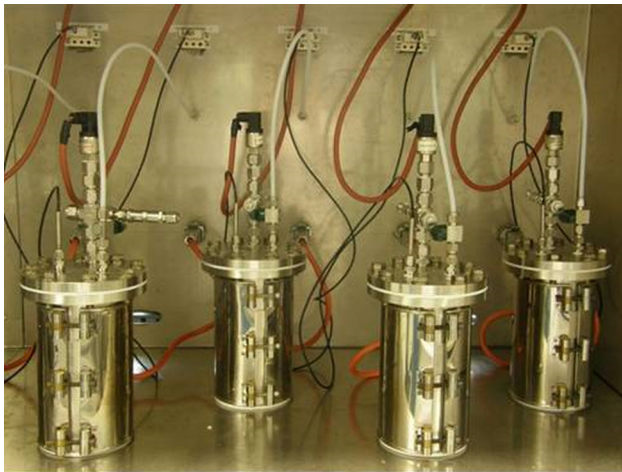
FIG. 1 Picture of the high temperature oxidation test setup.
