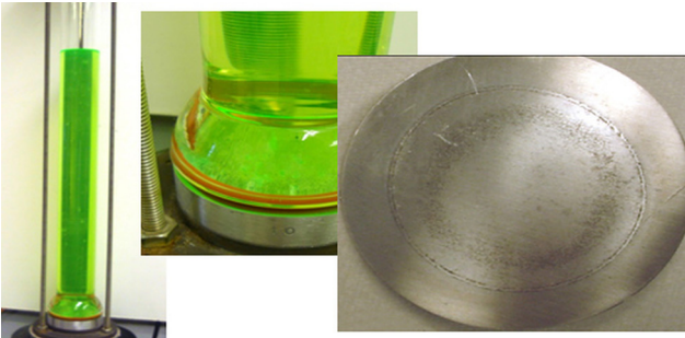
FIG. 6 Satisfactory test result: clear fluid, no deposit, no weight loss.
