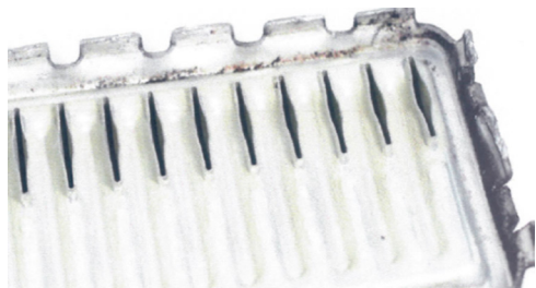
FIG. 4 Post-braze flux residue in radiator header channel.
