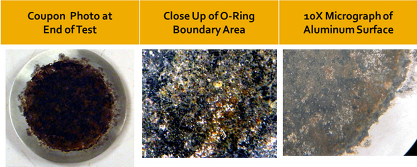
FIG. 5 Corrosion of aluminum specimen.
