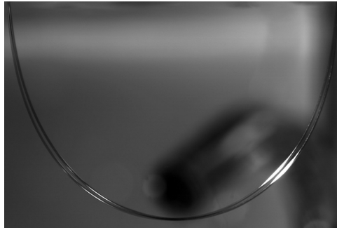
FIG. 6—Two superimposed frames from a high-speed video of a nitinol wire illustrating the lateral rocking motion. The alternating strain was 1.0 %, and the test speed was 60 Hz.
