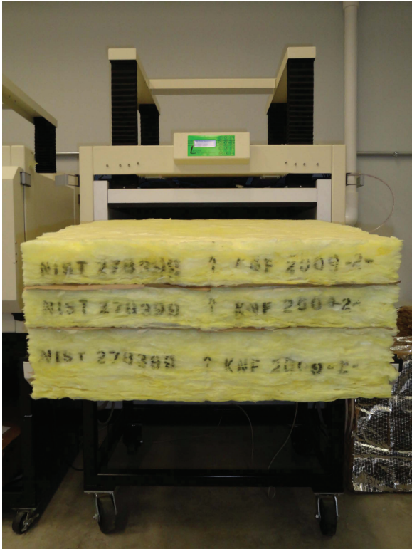
FIG. 3 Slab No. 3 added to the stack. Last 3 in. primary CTS fiberglass standard of known thermal conductivity added with septums between layers with a total stack thickness of 305 mm (12 in.).
