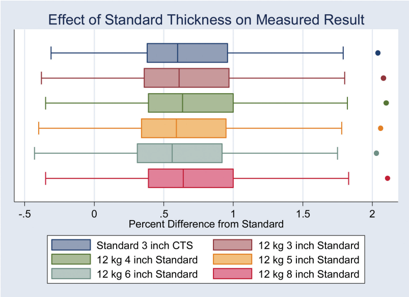
FIG. 11 Effect of standard thickness on measured result. The density is 12 kg/m 3 .
