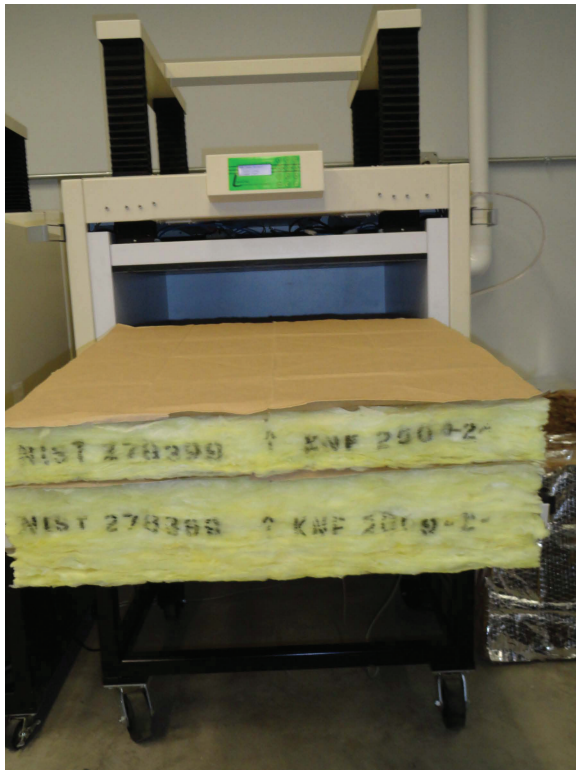
FIG. 2 Slab No. 2 added to No. 1. Slab No. 1 is 6-in.-thick primary CTS fiberglass standard with septum between next slab No. 2, a 3-in.-thick primary CTS fiberglass layer in the middle.
