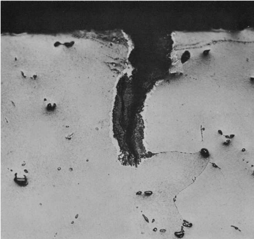
FIG. 22—(a) Profile of crack in specimen A after twenty-five loading cycles located at minimum cross-section. (Magnification of 260).
