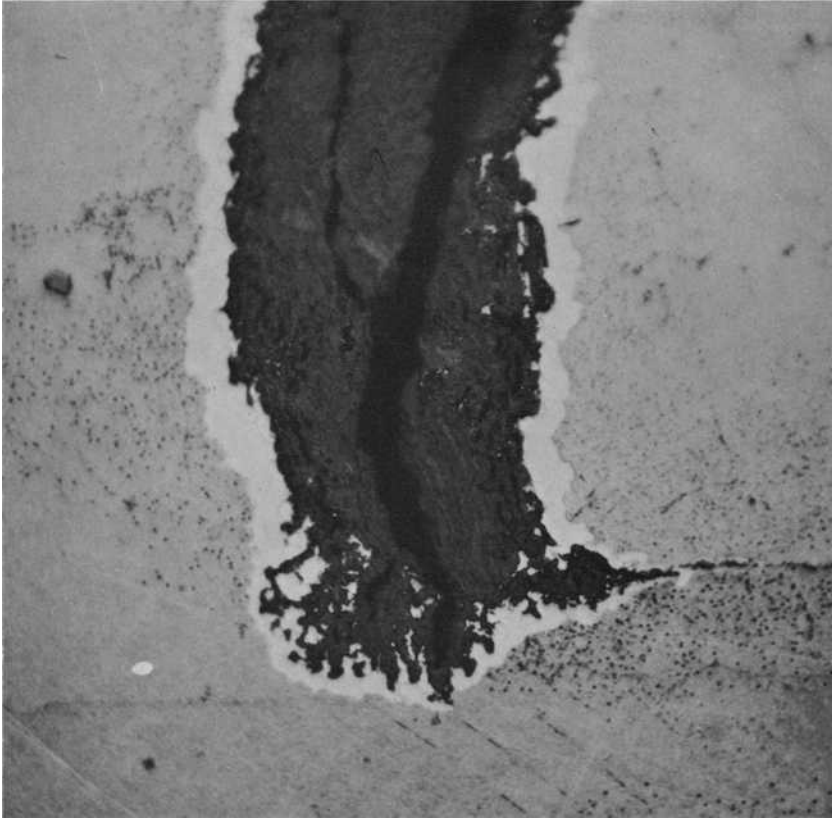
FIG. 22 (Continued)—(b) Detail of tip of crack in (a) showing tendency of oxidation to follow grain boundary. Note Area of depleted \gamma' at periphery of oride. (Magnification of 780).
