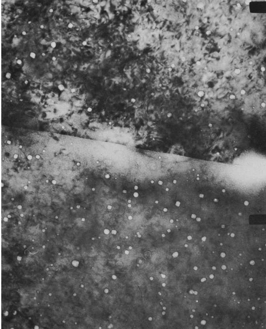
FIG. 18—Voids in irradiated type 304 stainless steel[42] (Distance between marks equals one micrometer.).
