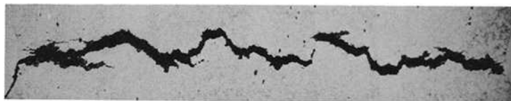
FIG. 11—Transverse cross section of nearly fractured ductile low alloy steel notch specimen.
