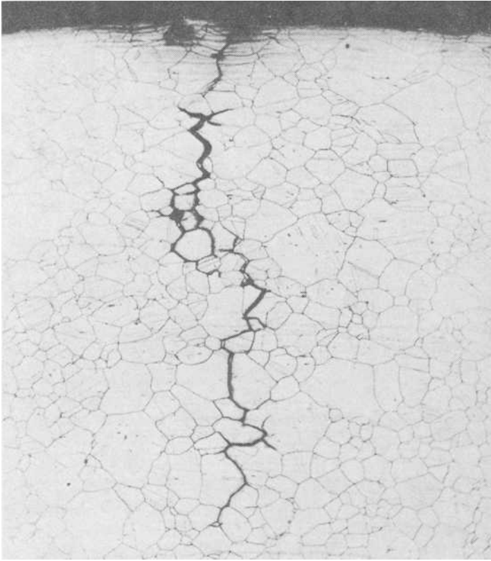
FIG. 3— Intergranular stress corrosion cracking of Inconel 600 in high temperature water (X 70).
