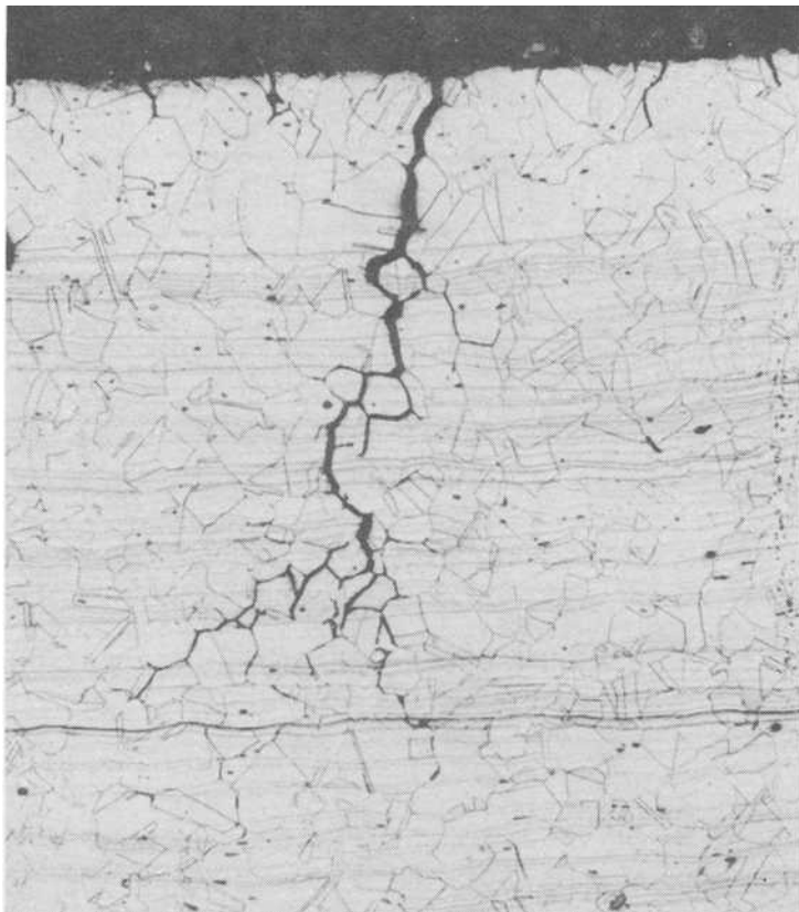
FIG. 2—Intergranular stress corrosion cracking of Monel 400 in steam ( \times 100 ).
