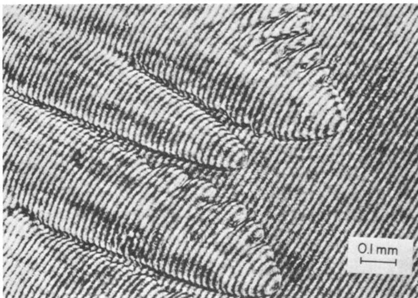
FIG. 6—Dendrites of camphene, reconstructed from a hologram. The arrangement of Fig. 4 was used to generate the interference fringes, with the beam splitter being tilted to align the fringes perpendicular to the dendrite axis.
