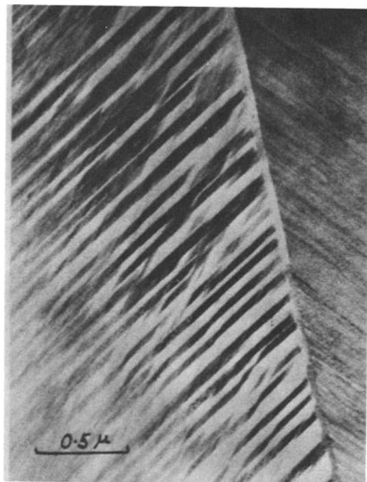
FIG. 18—Micrograph of fine twins on \{112\} planes of martensite plates in a Fe-24Ni-0.5C alloy.
