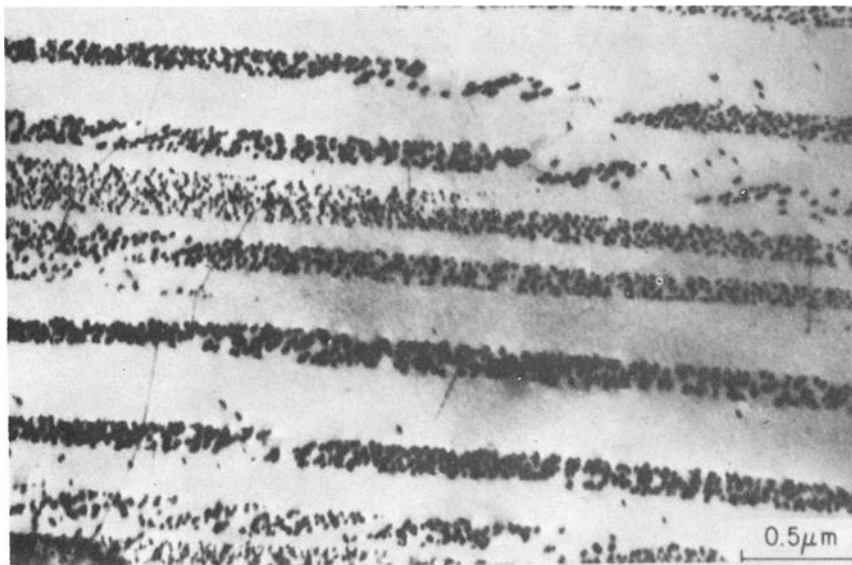
FIG. 24—Walls of columbium carbide formed at ferrite-austenite interface as a result of discontinuous transformation (1000 kV).
