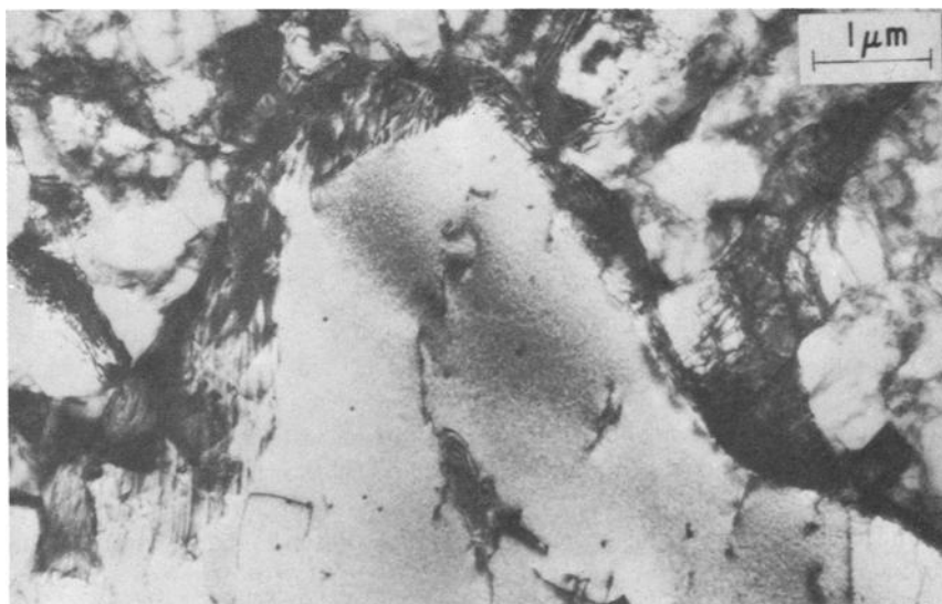
FIG. 20—HVEM micrograph illustrating partial recovery ahead of mobile boundary in recrystallizing iron (1000 kV).
