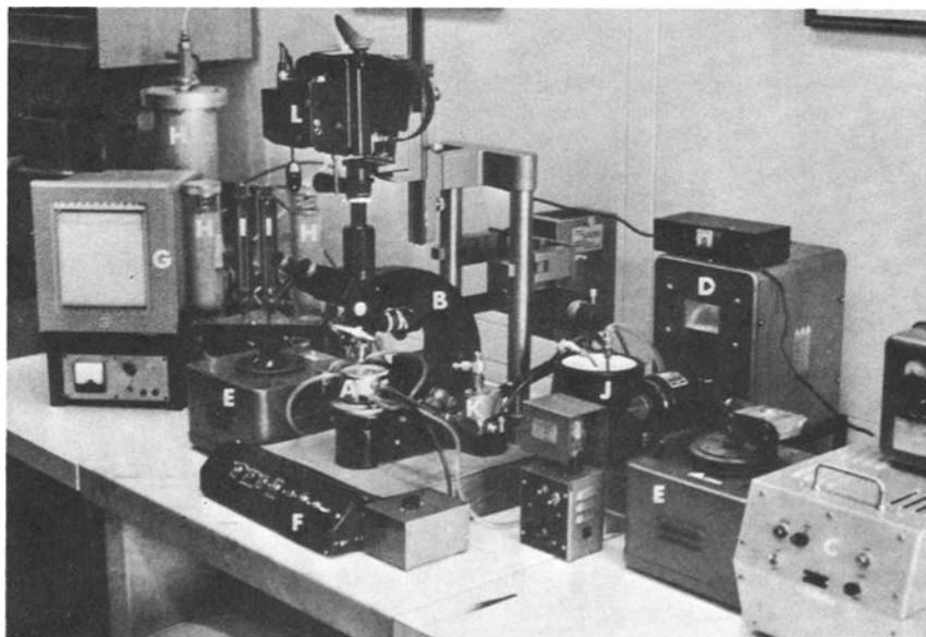
FIG. 1—Overall view of the hot-stage setup used for this study showing the basic system: (A) Leitz 1750 heating stage, (B) Leitz Ortholux microscope with xenon lamp, (C) Leitz power supply for 150-W xenon lamp, (D) power furnace transformer (5 V, 750 W), (E) regulating transformers, and the modifications: (F) control switching unit, (G) strip chart recorder (AZAR), (H) gas drying system, (I) gas flow meters, (J) liquid nitrogen bath (Dewar flask), (K) solenoid valve, and (L) Bolex 16-mm camera.
