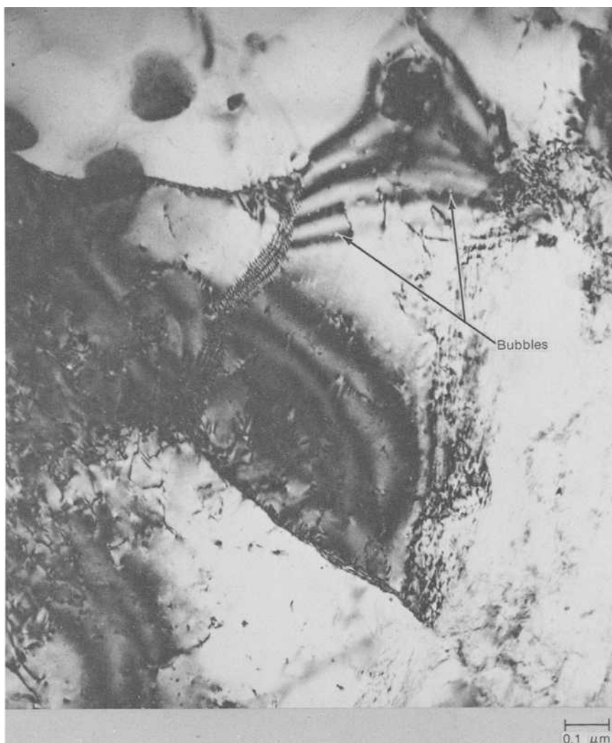
FIG. 7—TEM micrograph showing bubbles and remains of some clusters, loops, and dislocations after annealing at 1047 K for 1 h.
