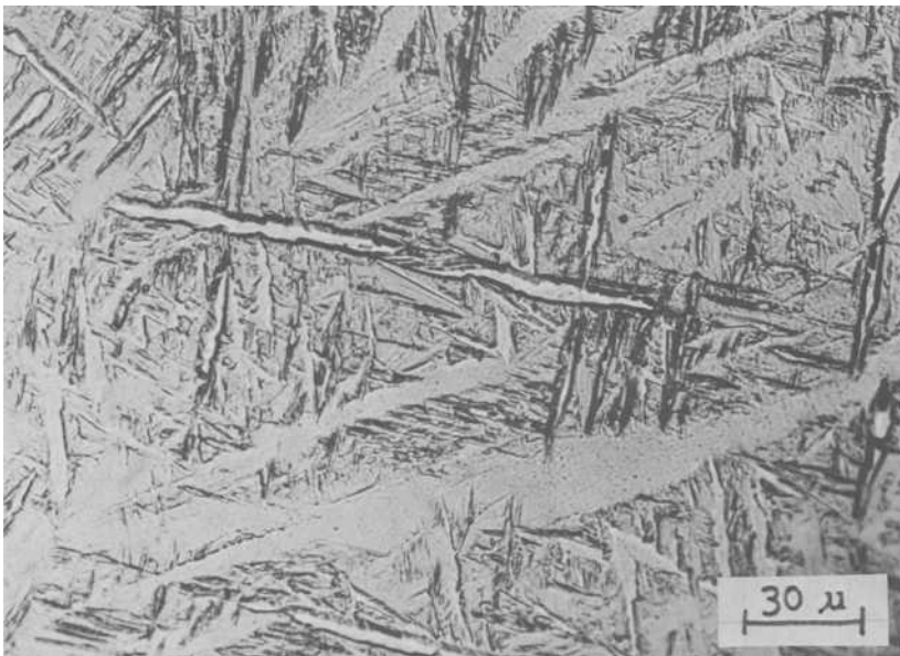
FIG. 18—Martensitic \alpha with some \beta and prior \beta -grain boundaries in the fusion zone of the laser-beam weldment of the titanium alloy. The hardness is 32 to 38 HRC. The material is etched in Kellers.
