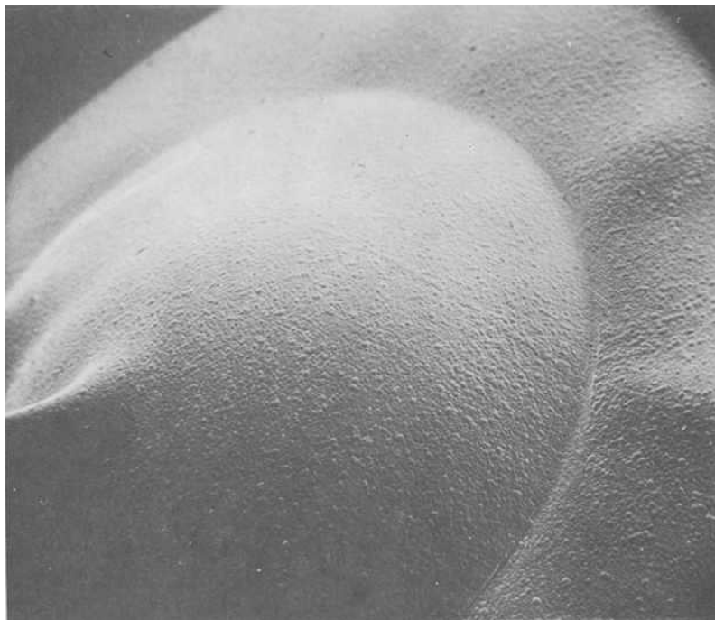
FIG. 4—Hemispherical cup formed in testing ductile foil ( \times 40 ).
