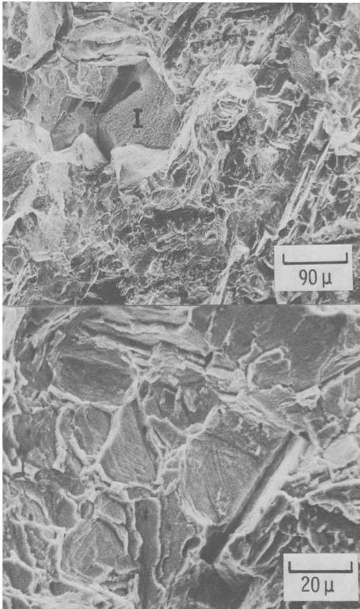
FIG. 9—Fractographs of the 427°C fracture surface: (top) intergranular dimple-rupture network (I) surrounded by a faceted transgranular morphology; (bottom) evidence of a rather flat, faceted appearance, coupled with poorly defined dimples.
