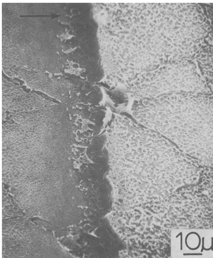
FIG. 12—A photomicrograph of a PVC fracture surface showing boundary failure around the original resin particles. Note the prominent stretch zone. M_w = 1.41 \times 10^5 , 6 percent DOP, \Delta K = 1.00 \text{ MPa } \sqrt{m} .
