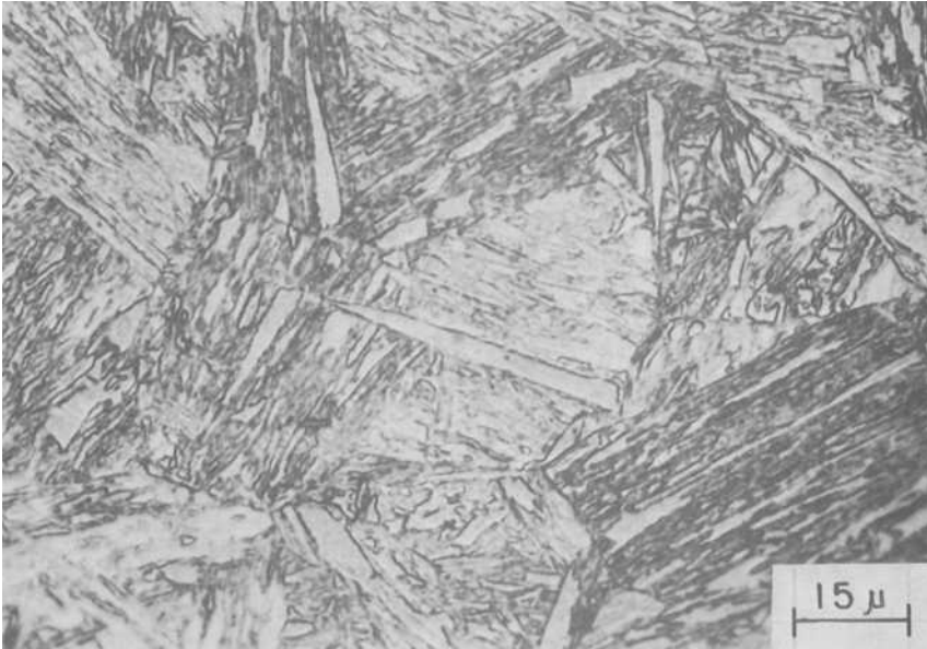
FIG. 3— Untempered martensite and bainite in the fusion zone of the HY-80 laser-beam weldment, etched in 1 percent nital. The hardness is 44.0 HRC.
