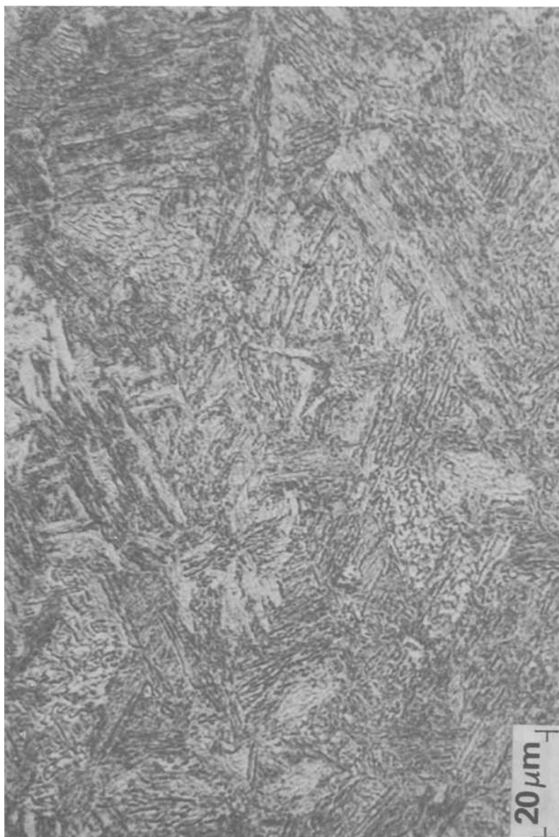
FIG. 16—HY-180 (9 nickel) EF-VAR specimen, tempered, with heavily tempered martensite and bainite. The specimen is etched with 2 percent nital.
