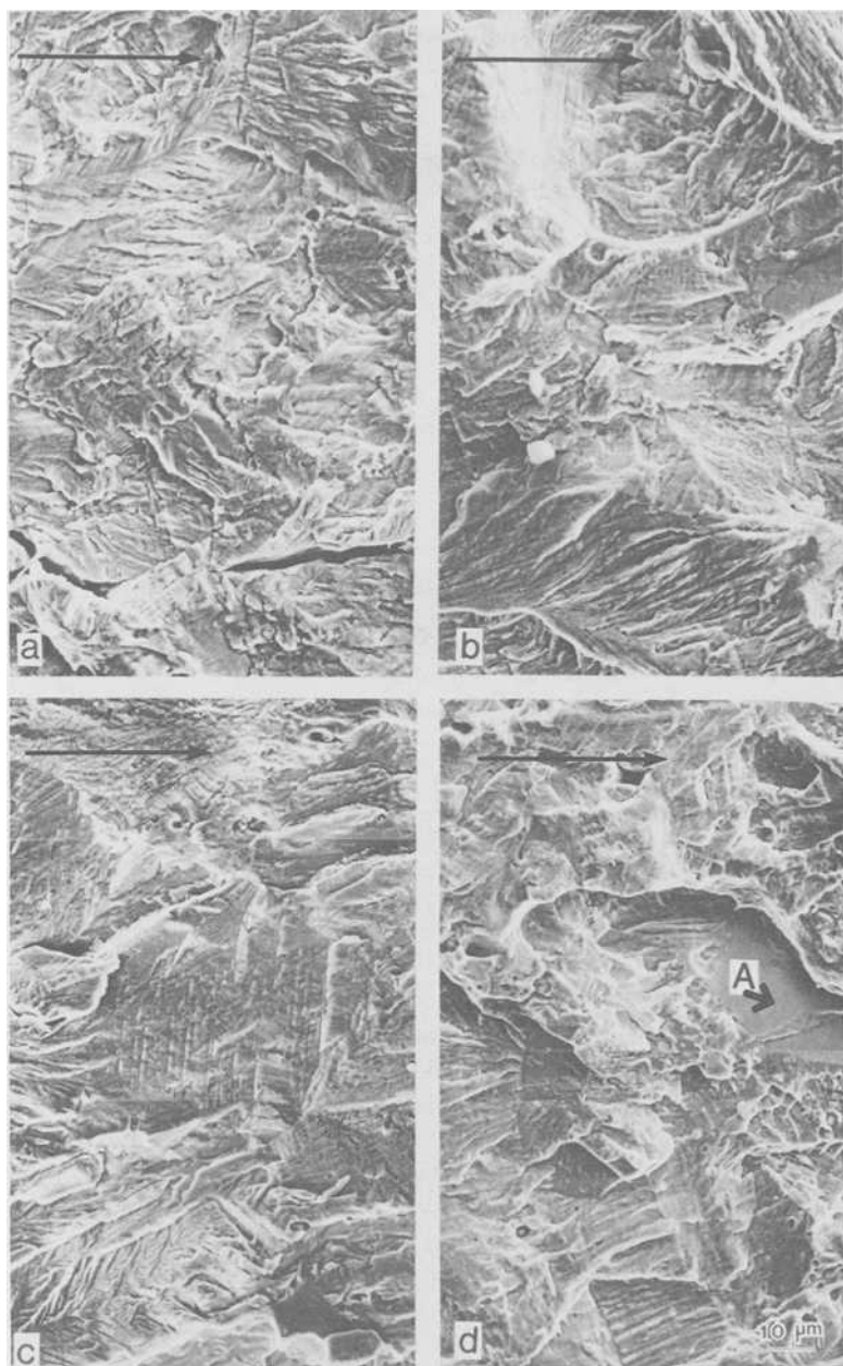
FIG. 5—Fracture surfaces after fatigue cracking at 4 K. (a) As-rolled, \Delta K = 35 \text{ MPa}\sqrt{\text{m}} . (b) As-rolled, \Delta K = 45 \text{ MPa}\sqrt{\text{m}} . (c) Solution-treated, \Delta K = 35 \text{ MPa}\sqrt{\text{m}} . (d) Solution-treated, \Delta K = 45 \text{ MPa}\sqrt{\text{m}} . Arrows indicate macrocrack growth direction ( da/dN ). (A) indicates smooth grain facet.
