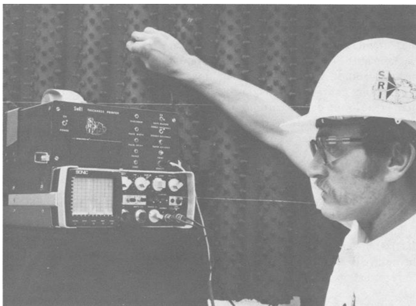
FIG. 1—Thickness printer mounted on ultrasonic instrument.
