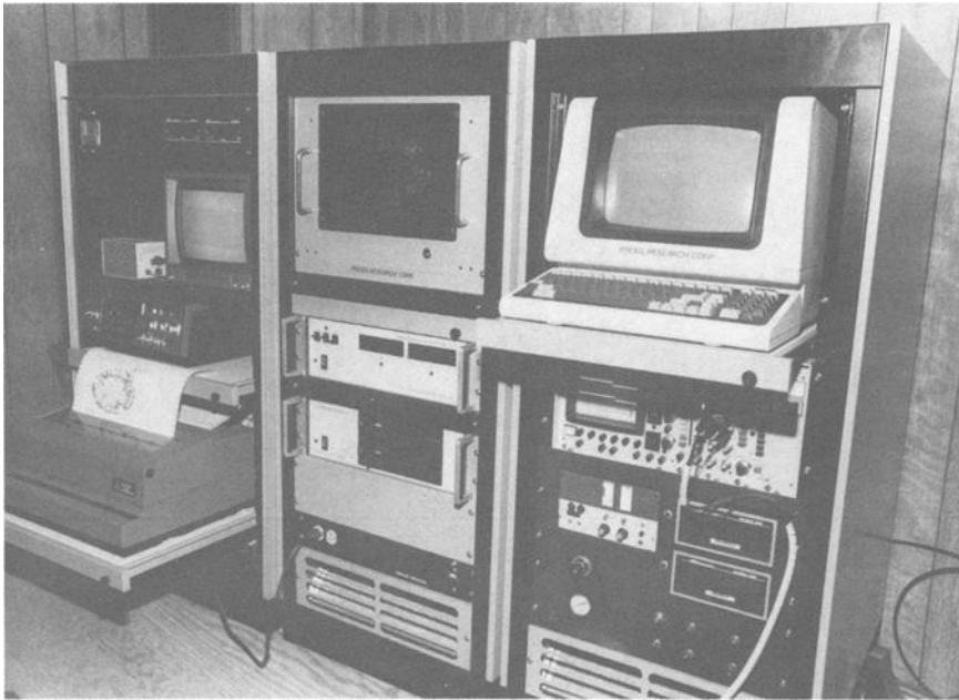
FIG. 4—Ultrasonic inspection system housed in three portable cabinets (exclusive of probe assembly and positioner).
