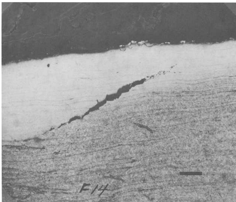
FIG. 14—Bore crack in tube manufactured from Steelmaker 2 continuous-cast steel (marker is 200 \mu\text{m} ).
