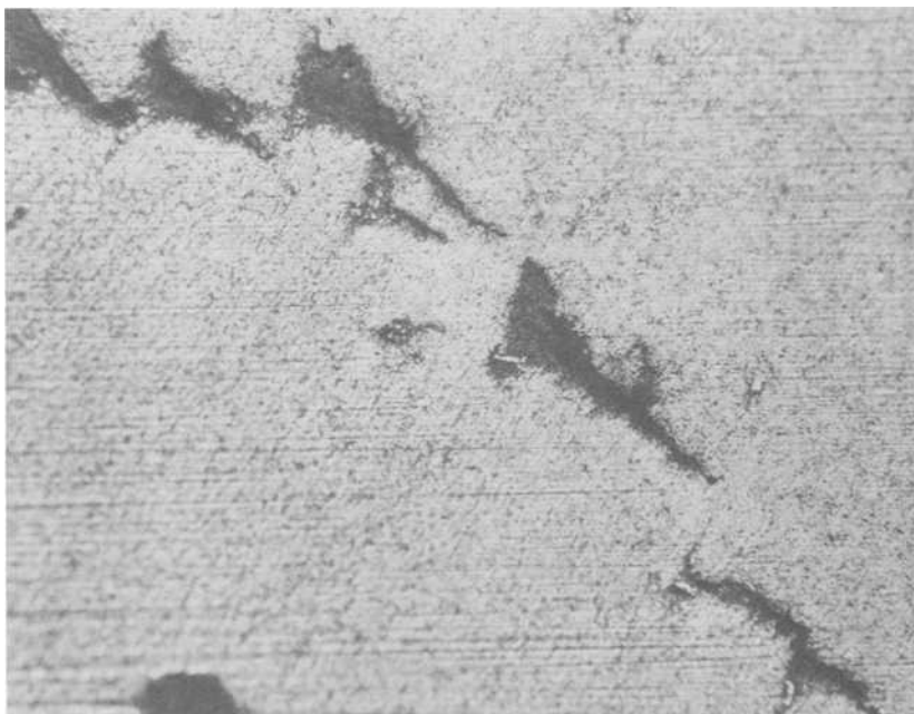
FIG. 4—Peeling pattern in raceway. Nital etched to show carbides at apex of triangular peeled areas. \times 200 .
