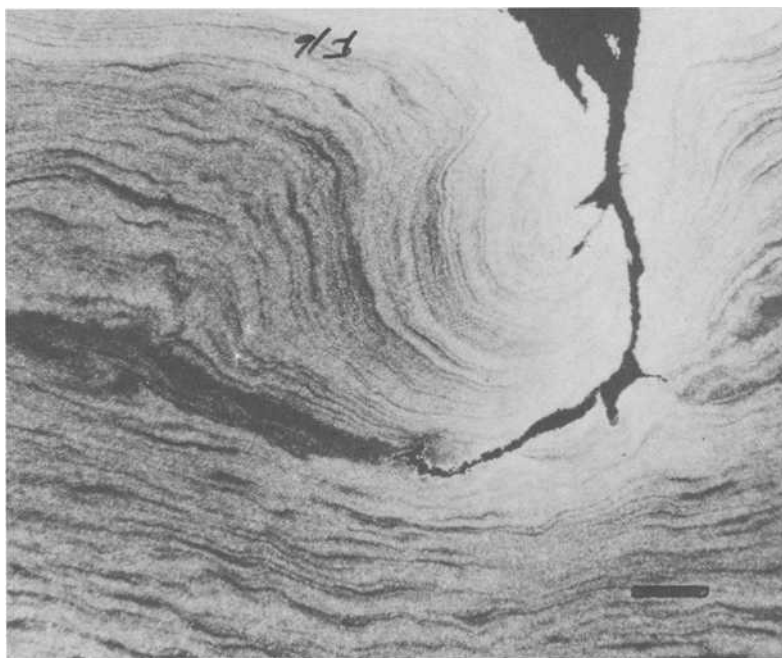
FIG. 16—Bore cracking associated with carbide segregation in tube manufactured from Steelmaker 4 continuous-cast steel (marker is 200 \mu\text{m} ). (Photograph courtesy of TI Desford, Ltd.).
