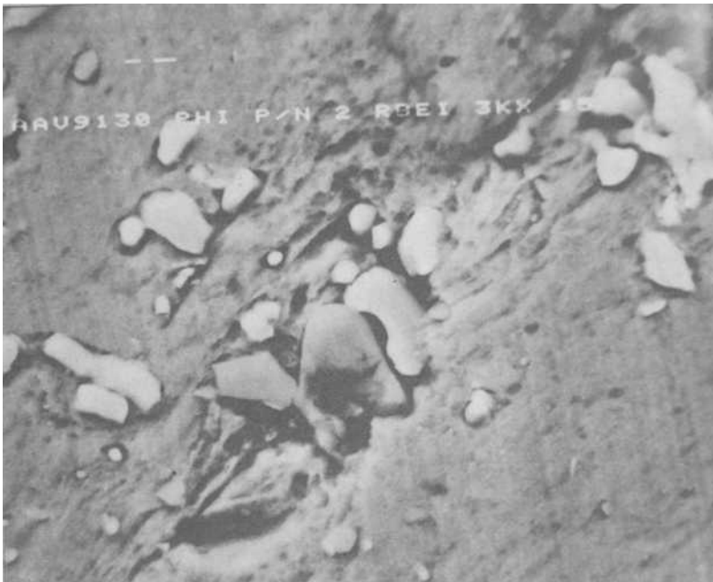
FIG. 6—Cracked and broken carbides at apex of peel. SEM, \times 3000 .
