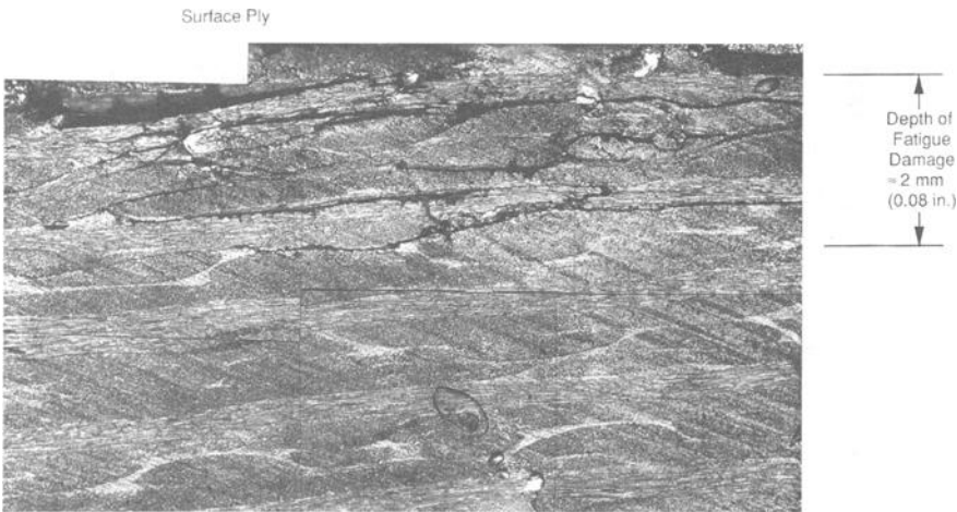
FIG. 14—Photomicrograph of stitched AS4/3501-6 after 650 000 cycles. R = 10 , 167-MPa maximum compressive stress, 822 000 total cycles to failure.
