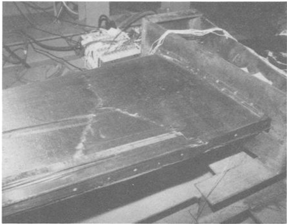
FIG. 10—Full-span test piece after failure.
