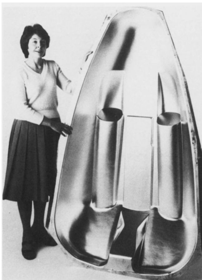
Fig. 1. A lower engine cover from a Turbo-Prop aircraft formed in Superplastic Aluminium alloy. (Courtesy of Superform Metals Ltd.)
