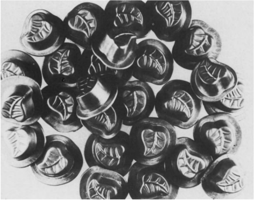
Fig. 6. A group of positive replicas made in a zinc-based alloy by pressing at 250°C into a cavity, itself made by hot-pressing of a steel master into an aluminium-silicon alloy at 500°C.
