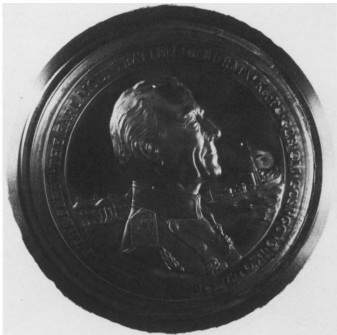
Fig. 4. A 180mm diameter replica plaque made in a superplastic zinc-aluminium alloy, showing the degree of detail that can be reproduced accurately.
