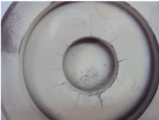
Figure 48. Typical Thermal Fatigue Cracks in a PM.
