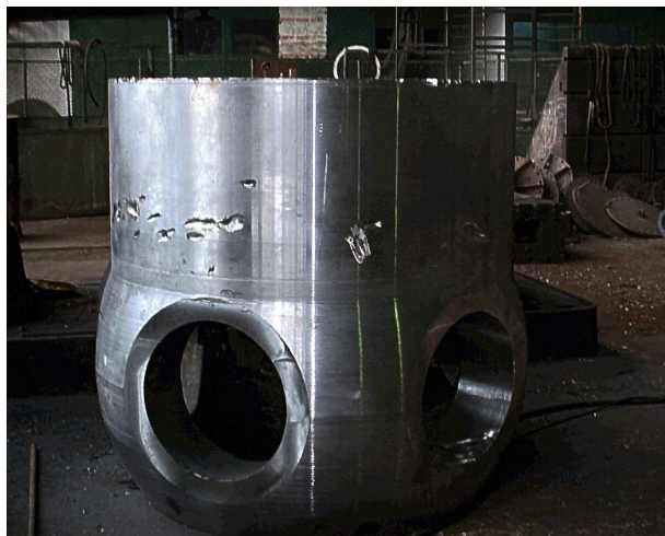
Figure 31. Porosity-type casting defects in the block window and on the exterior surface.
