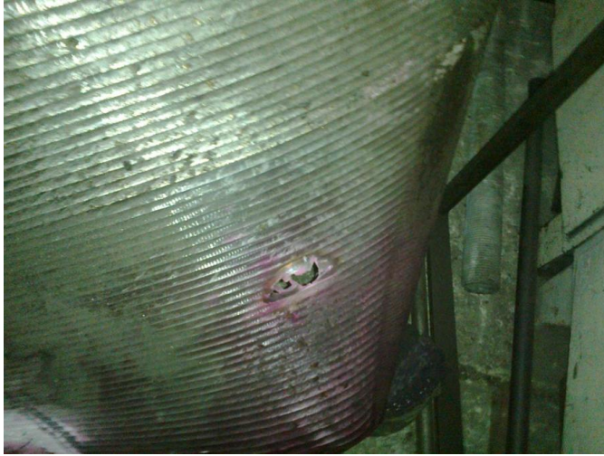
Figure 52. Position of the bubble open defect and of pores and oxides.
