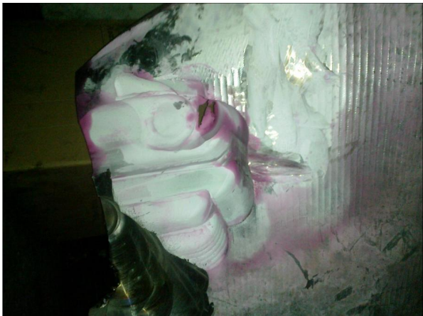
Figure 51. Detail in the analysis of the effect of penetrating substances on the blade surface.
