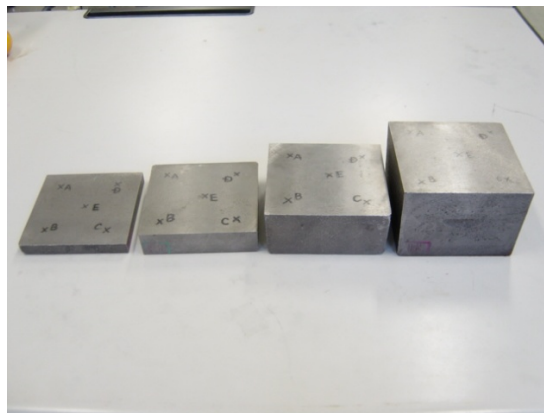
Figure 10. The specimens with three kinds of surface conditions (as-cast, machined and shot-blasted: 100 mm square, continuously cast bar).
