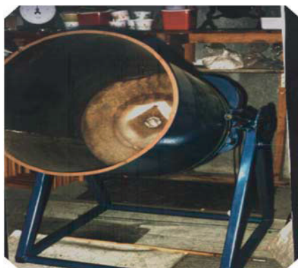
Fig. 65 Suitable for larger quantities than the small manual bowl (described below) and electrically or motor driven but still operated by manual input of all ingredients is this standard coating [and precision pelleting] bowl similar to a small concrete mixer but with some important differences.
