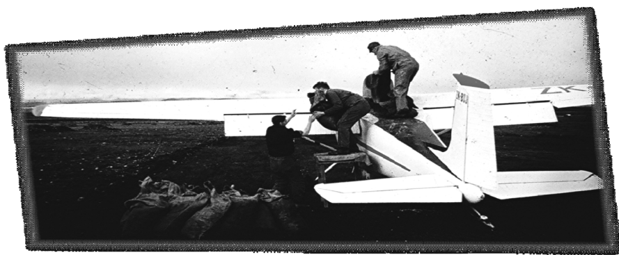
Fig. 32 Manual loading of topdressing aircraft may be necessary where a loader vehicle is not available, however, it allows less expensive pre-mixing and bagging a day or two prior to flying on. Bags need to be weighed so the aircraft does not exceed its operating weight limit.
