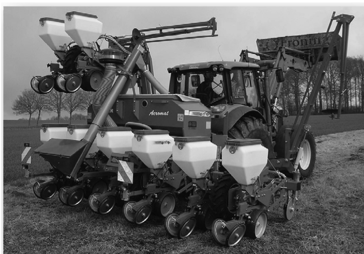
Fig. 4 A modern precision drill. This is a top class model Becker Kongskilde Aeromat Profi-Line machine. It has a classic eight row electronically controlled (from the tractor cab) hydraulic fan (compressed air) metering system. Twin side units are retractable (as shown above on the left side) for passing through gates, etc. This is an ideal machine for large farms or contractor use.
