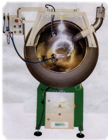
Fig. 54 A fully equipped precision pelleting drum fitted with electrically controlled and adjustable liquid spraying device (left) plus pelleting solids by aerated tube (right) and is well illuminated by a fixed light (centre top).
