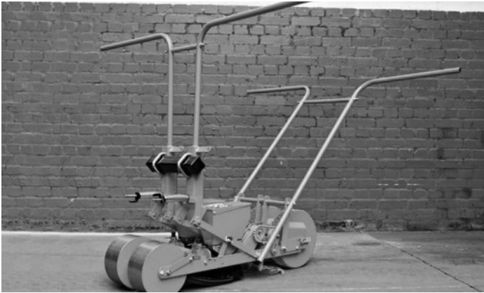
Fig. 47 Two Stanhay 820 belt drive precision drill units connected up for 4 person push pull operation] at minimal cost.
