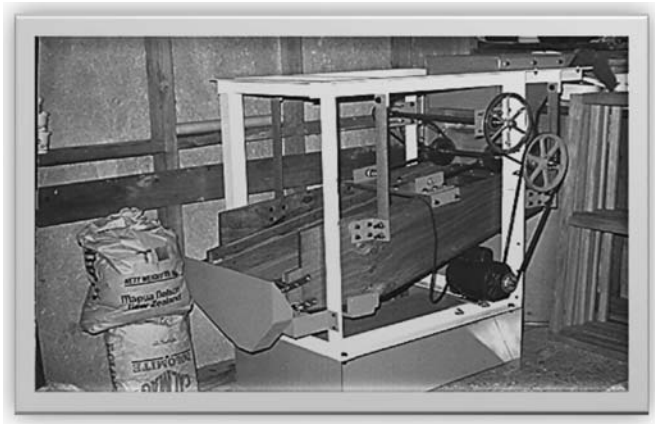
Fig. 70 Built for quite small production, more clearly demonstrates the way these screeners work. This illustration is repeated here as in Chapter 5 because it is also suitable for precision pellet screening].
