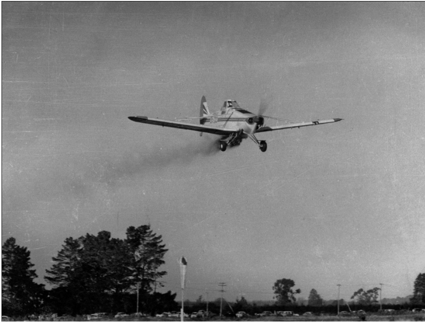
Fig. 27 Superphosphate and coated seed are dispersed to a known width and known rate of spread but is subject to wind direction and strength, height and speed of aircraft—all under control of an experienced pilot. The fertilizer seen leaving the aircraft here is dusty, not granulated, the “fines” can travel long distances, undesirably onto neighbours land, into riverbeds, the sea or scrub and bushland. Accuracy is essential.
