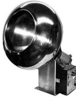
Fig. 53 This bowl is specially suitable for processing smaller runs of precision pelleted seed but also for preparation of coated seed and research treatments over the whole range—as used by Axis Associates, Nelson, New Zealand. A similar bowl to this can be purchased from Disha Engineering Works, India called a lab coating bowl [ http://www.dishaengineering.co.in ].
