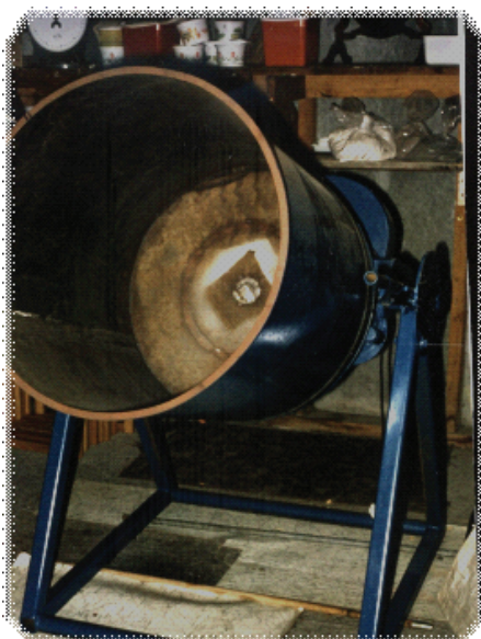
Fig. 52 A simple pelleting drum capable of producing about 2 Tonne per day of precision pellets when operated by a skilled technician. Costing $1,000 in 1979 it is constructed of 1/8" mild steel plate, the bowl diameter being .7 metre wide and .8 metre depth with a clear interior and the bottom lip of the bowl being 1 metre from the ground. It has an exterior chain drive from a 1 h.p. electric motor geared to rotate the bowl at 25 r.p.m. The frame comprises 1½ inch mild steel legs which are adjustable in height (threaded) and the base plate holding the drive cog is reinforced. This simple machine has given good service and is all that an operator needs to commence a simple pelleting operation but requires skills which can be acquired using some reject seed about to be dumped, to develop and practice the skills essential for continuous commercially acceptable product. This bowl is also suitable for processing inoculated coated legumes and coated grass seed.
