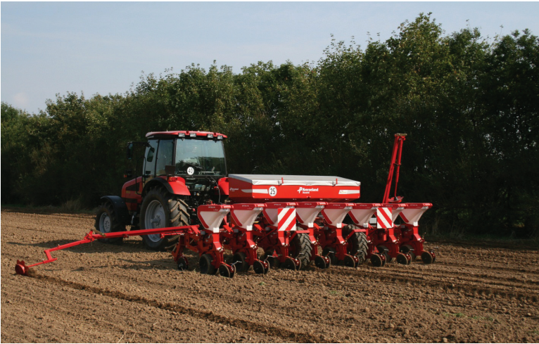
Fig. 50 The illustration (above) shows a “Kverneland Accord” pneumatic precision drill which has an important rapid change wheel for various sized seeds and pellets (Illustration by courtesy of www.kvernelandgroup.com/accord and their New Zealand Agency “Power Farming New Zealand Ltd.”).
