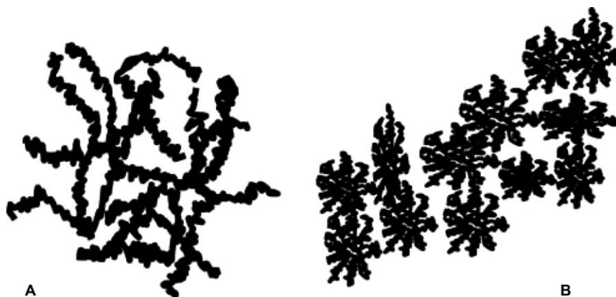
Figure 6.11 A cartoon showing linear weakly cross-linked and highly branched clusters, A: acid catalyzed B: base catalyzed hydrolysis. Reproduced from ref. 60 with permission from the Royal Society of Chemistry.
