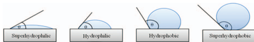
Figure 6.4 Schematic of the contact angle of a droplet on different surfaces.
