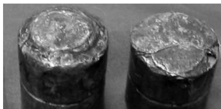
FIGURE 2.10 (See color insert.) Electrode wear in welding steel.
