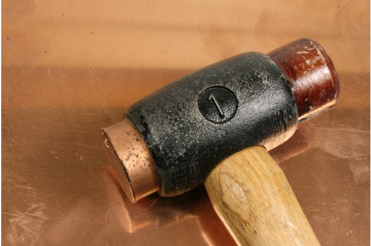
Fig. 1-6: Copper-headed hammer on a copper sheet.
