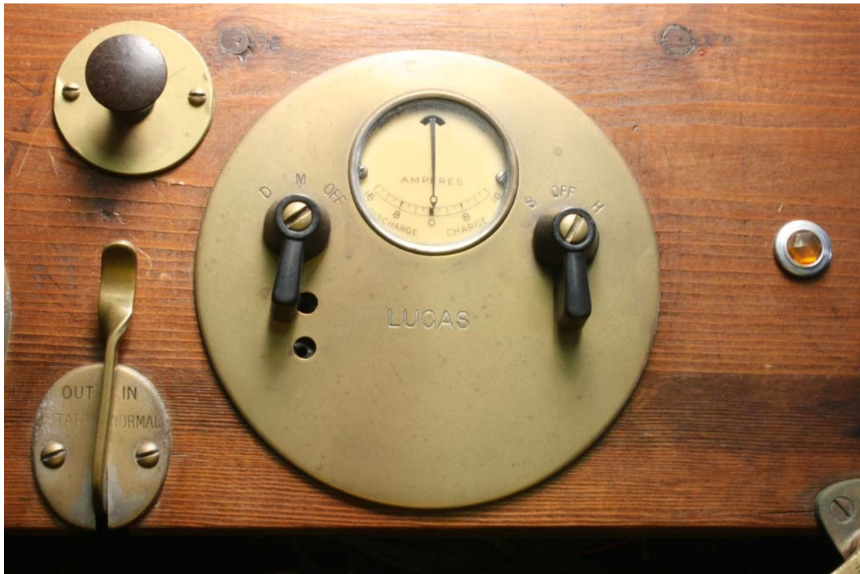
Fig. 1-4: Brass plates used as instrument housings; these items would originally have been plated with nickel or chrome. The vehicle in this photograph is owned by Dennis Nutt.
