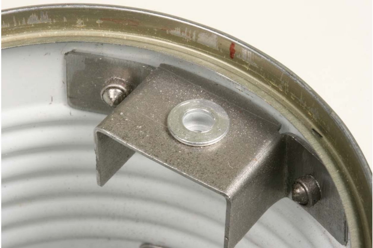
Fig. P2-24: Fit a rivnut to each bracket.
