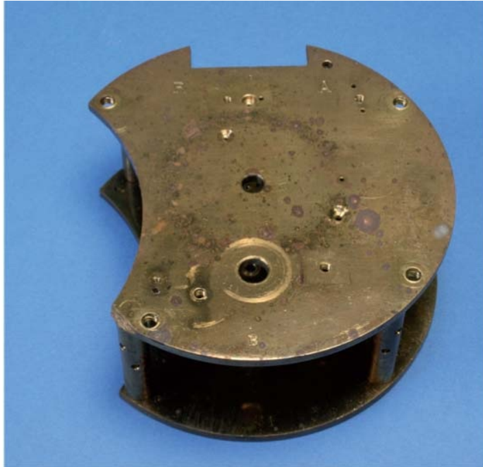
Fig. 10-14: Brass tarnishes and may mark badly, requiring the use of abrasives to remove the stains.
