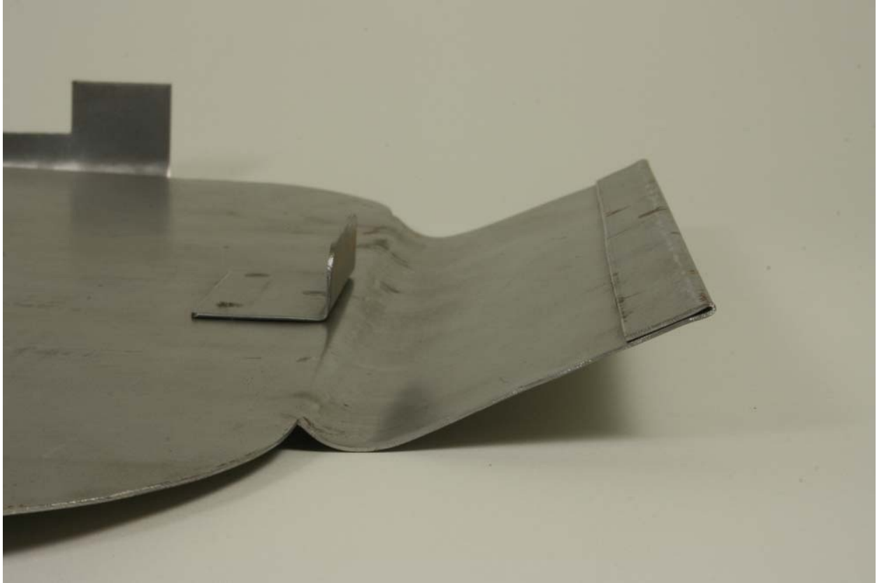
Fig. P6-8: Base locating stop welded in place.
