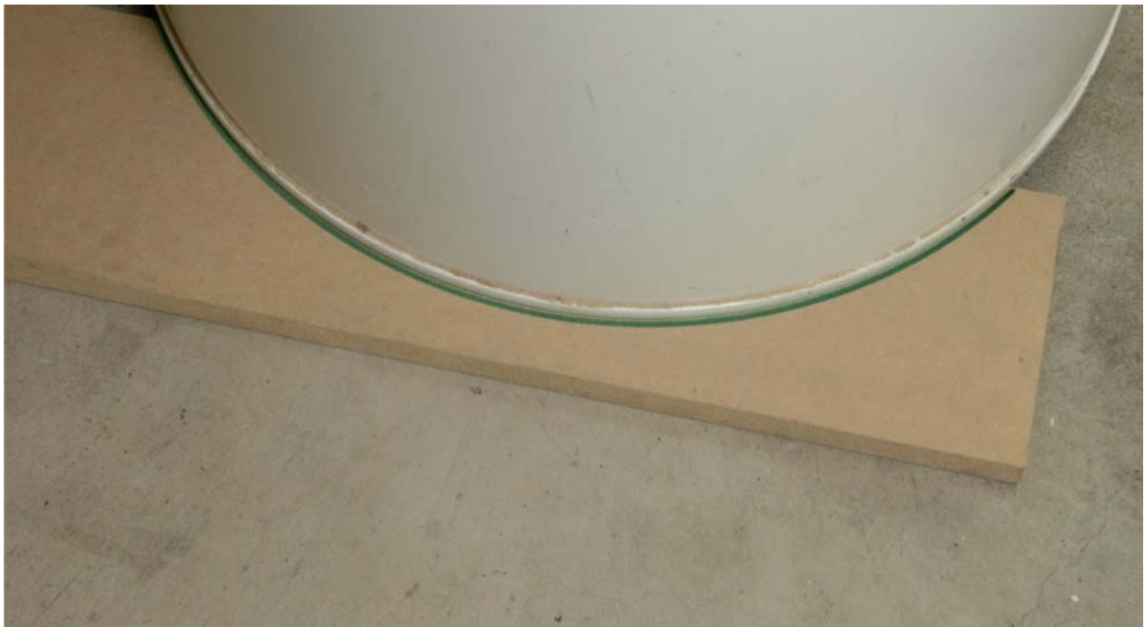
Fig. P4-10: Scribing a board to act as a template.
