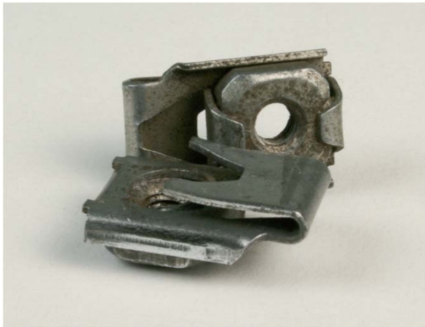
Fig. 8-11: U nuts hold captive nuts and, like U clips, can be located by pushing them over an edge.
