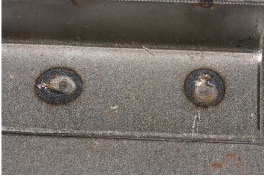
Fig. 8-50: Spot welds. The central silver spots are where pressure and current are applied to make the welds. The blue circles are heat marks.
