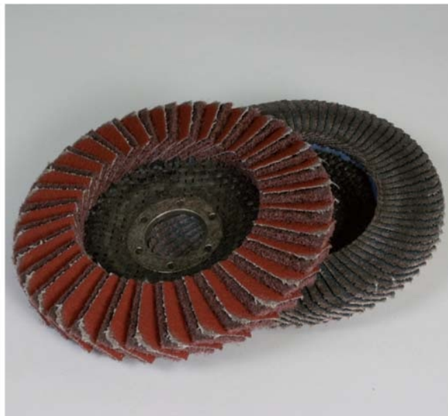
Fig. 10-4: Flap discs are available in a range of abrasives and grit sizes: the higher the grit, the finer the abrasive.
