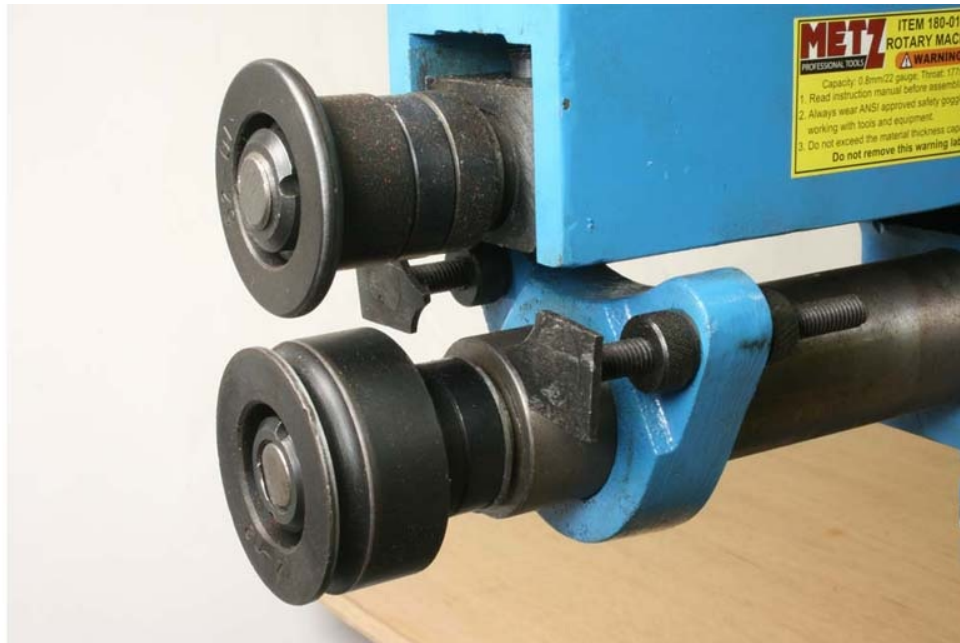
Fig. 7-10: Adjustable backstop (shown behind the lower roller) carrying two flat pads and which can slide along the lower shaft.
