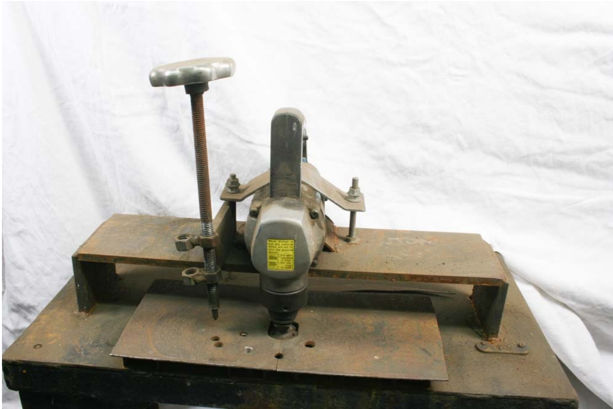
Fig. 4-25: Nibbler on a stand, for cutting external circles.
