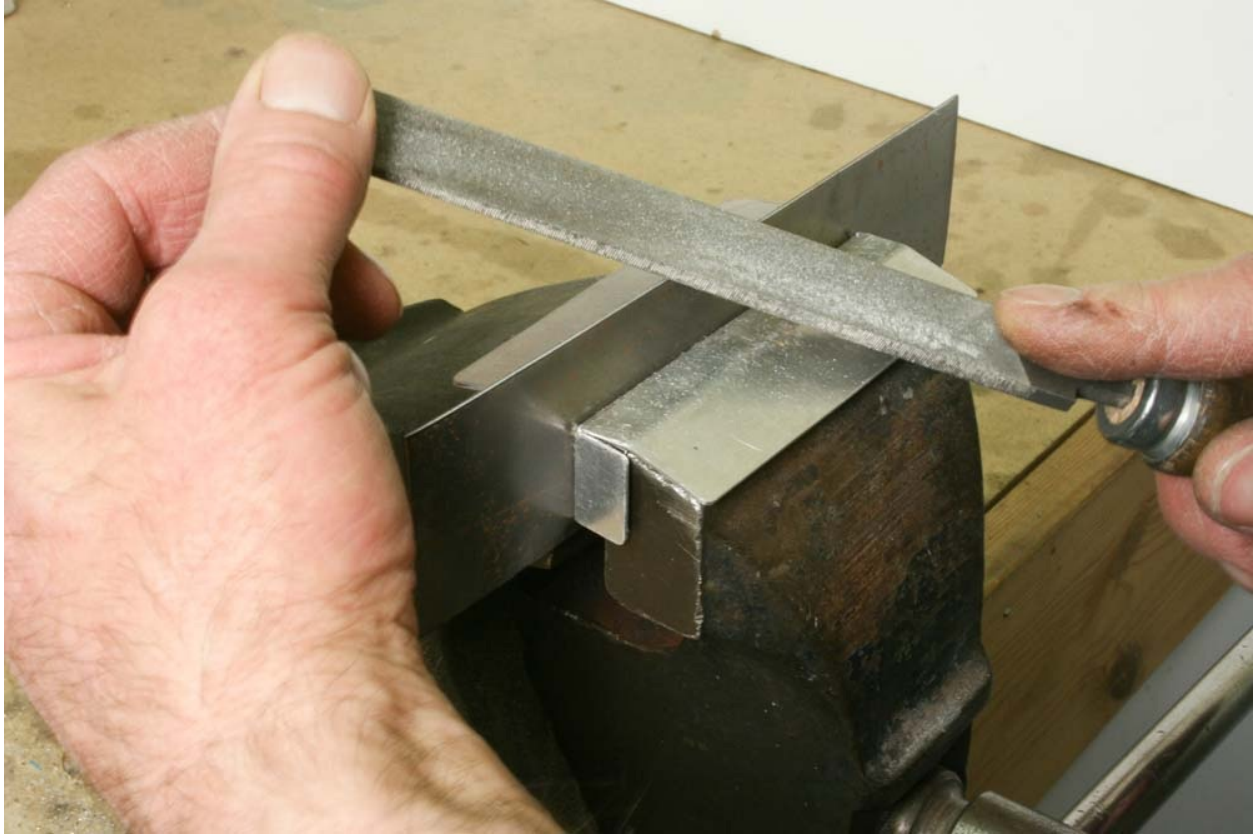
Fig. 4-32: File an edge at an angle of 45 degrees to the horizontal and 45 degrees to the vertical.
