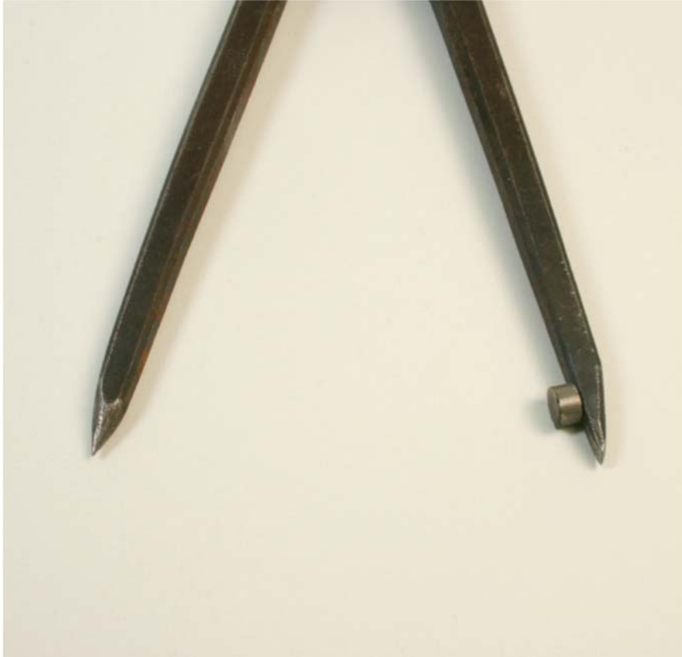
Fig. 3-16: A magnet may be used to make a jenny divider.
