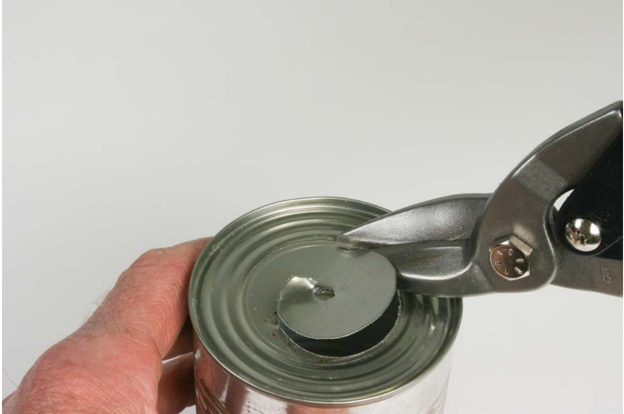
Fig. P2-10: Use the snips to cut in a spiral to reach the circumference of the circle, then cut round to create the hole for the ammeter.
