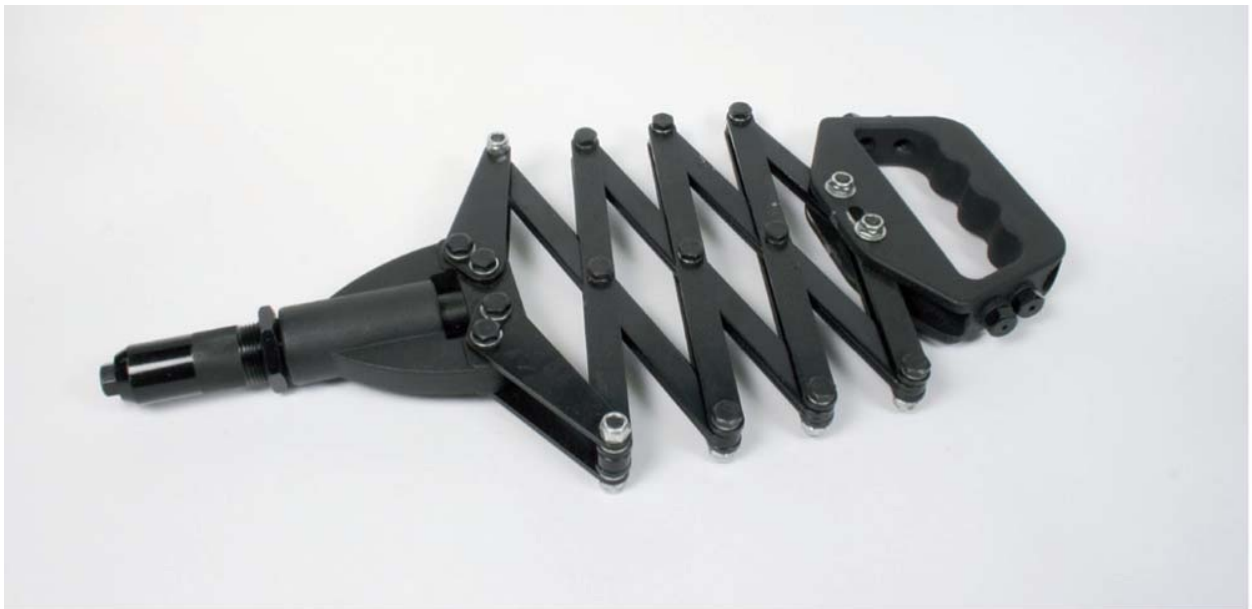
Fig. 8-29: Lazy tongs: concertina-style pop-rivet pliers that work using a pushing rather than a squeezing action.
