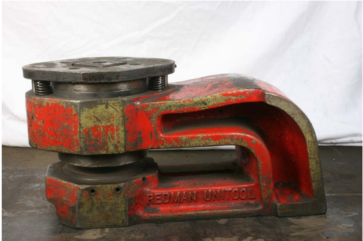
Fig. 5-17: Redman punch, designed to be used in a powerful press to punch large holes.
