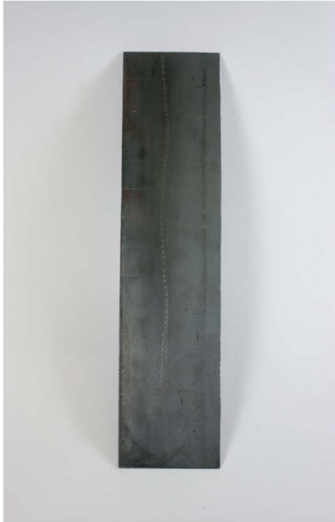
Fig. P4-6: Marking out for the external tube.
