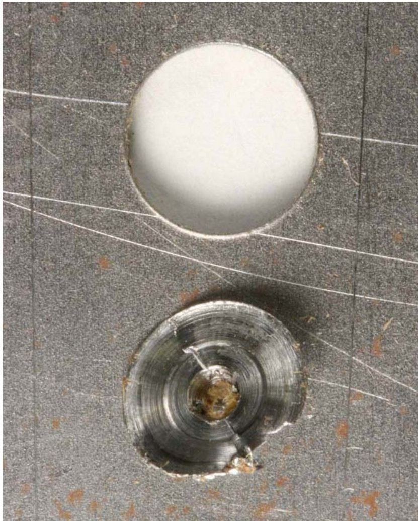
Fig. 5-6: Waste removed by a butterfly drill.
