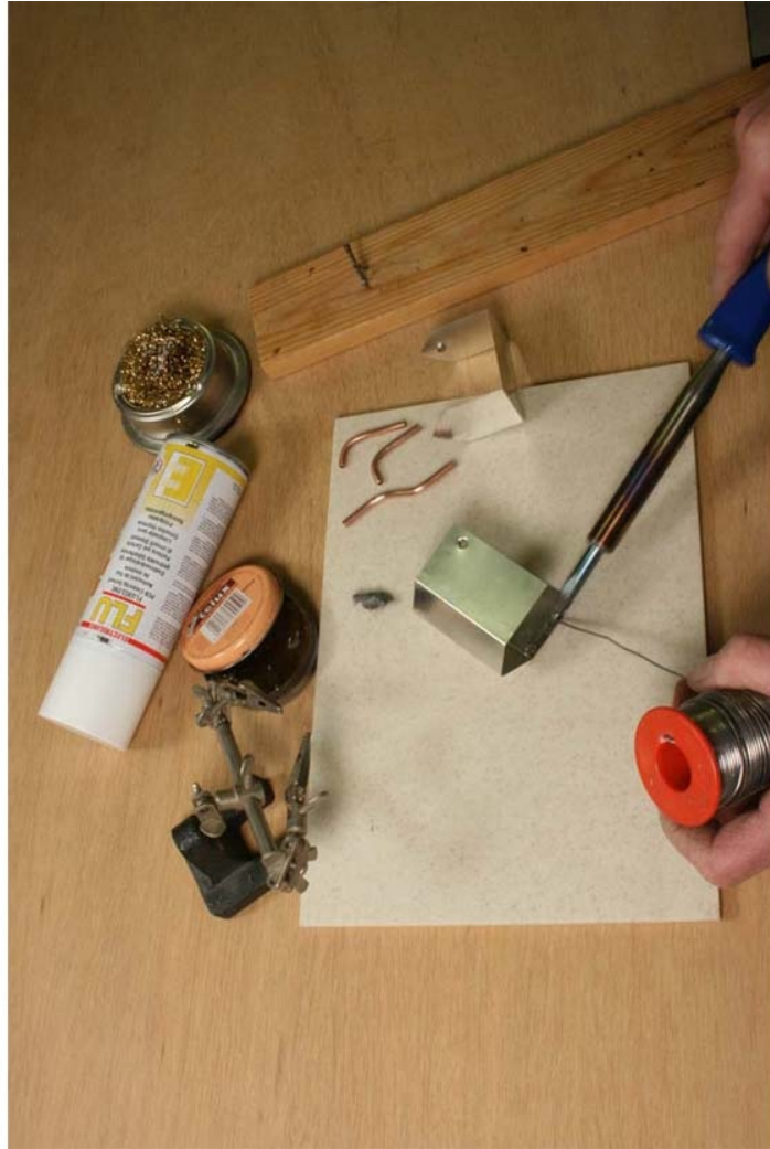
Fig. P1-17: Tinning the inside edge positions.
