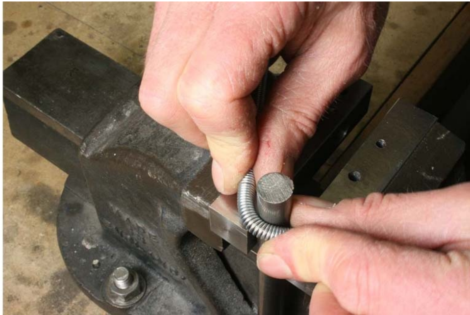
Fig. P1-13: Bending a copper pipe supported by an external bending spring.
