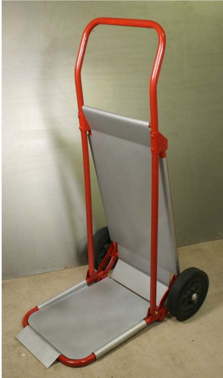
Fig. P6-2: The barrow, refurbished and fitted with additional support panels.
