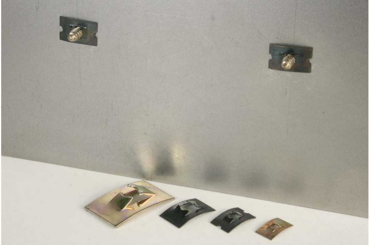
Fig. 8-10: Flat nuts can be used away from an edge and have a 'thread' formed from a punched hole and two flanges.
