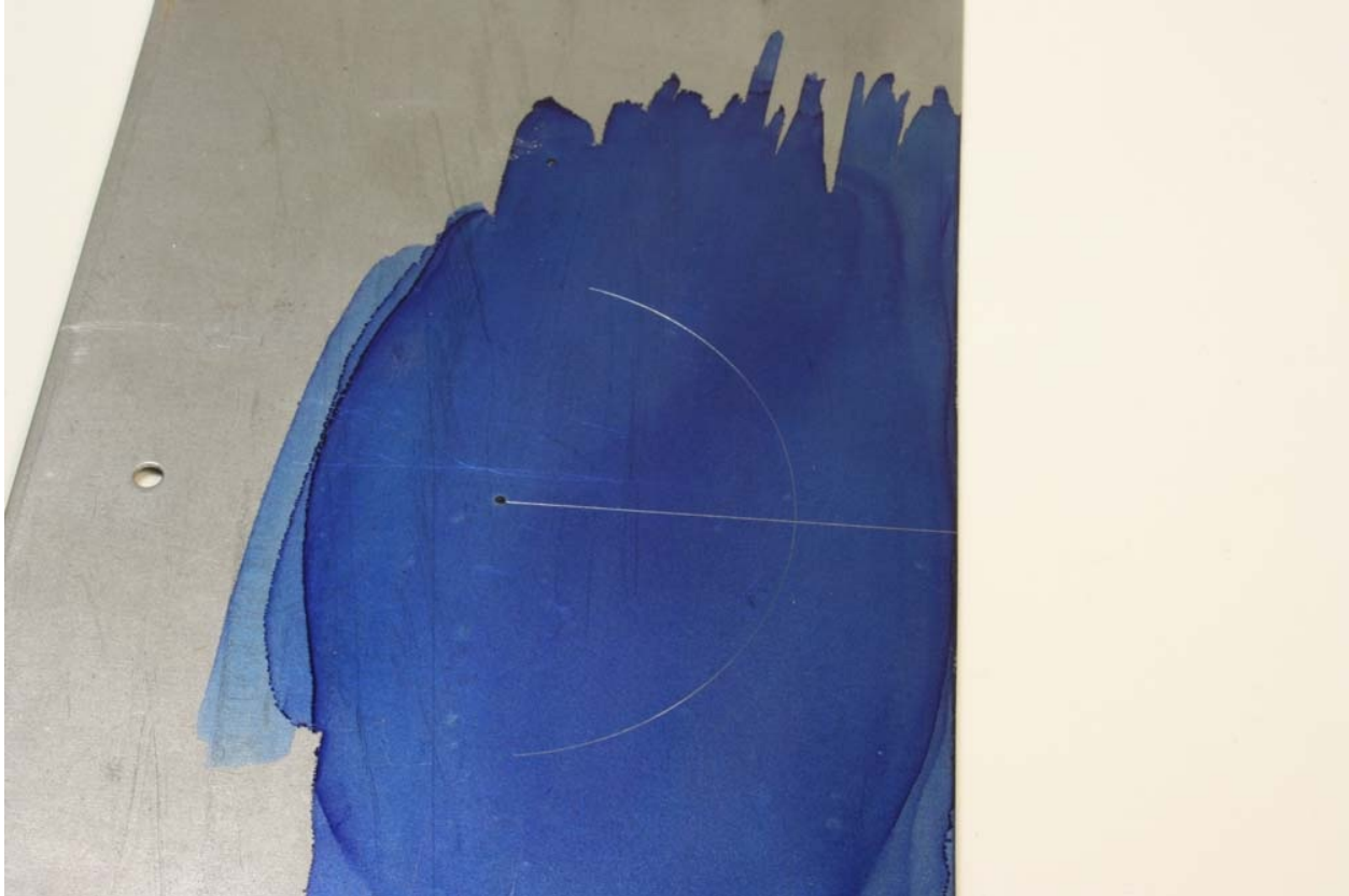
Fig. 3-4: Scribed lines show up well against blue marking-out fluid.
