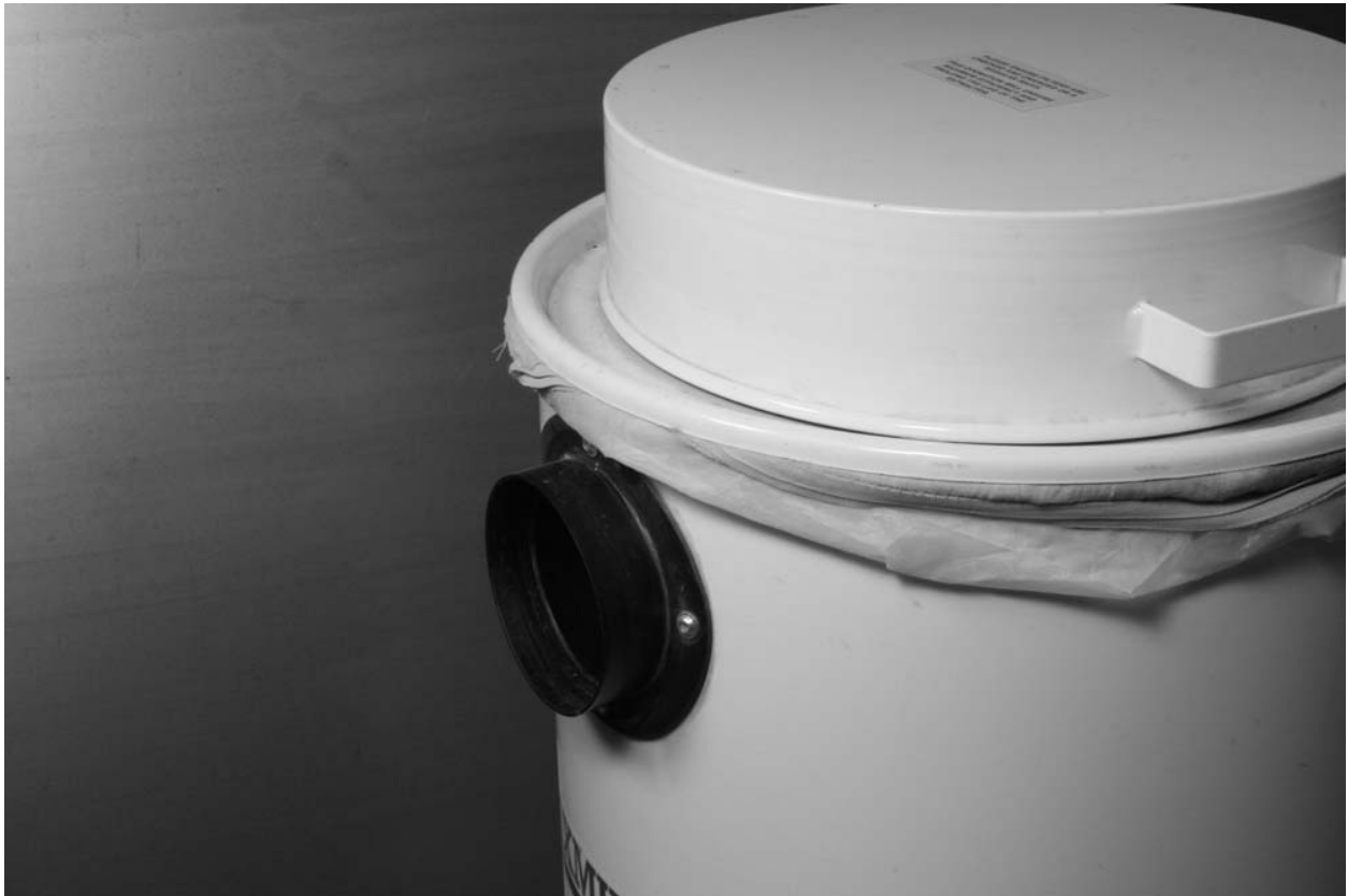
Fig. P4-1: Workshop vacuum extractor, showing the spigot for the hose.
