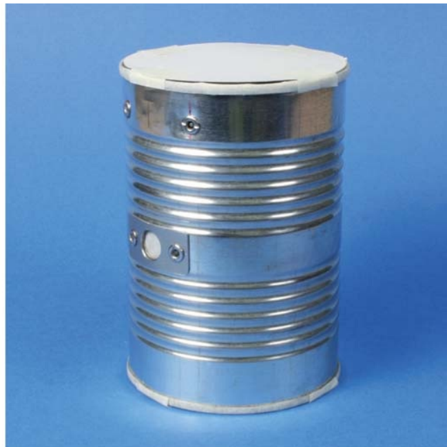
Fig. P2 27: Mask the ends in preparation for painting.
