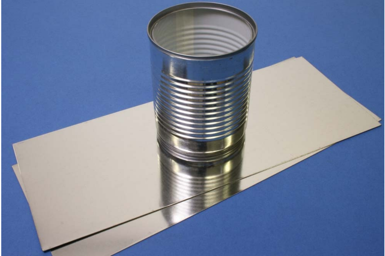
Fig 1-8: Still commonly used for everyday items, tinplate is also available in sheet form.
