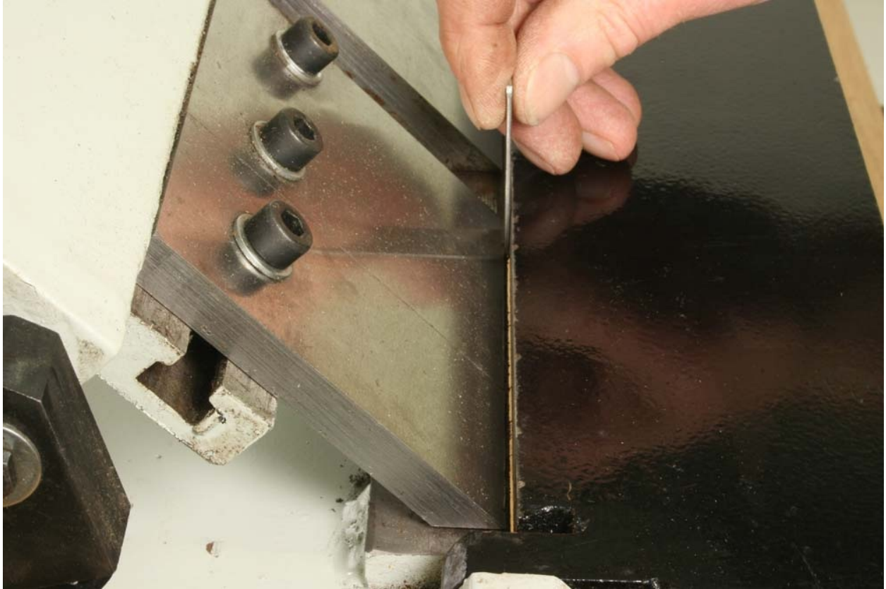
Fig. 6-12: Using a piece of sheet as a gauge to set the distance between the bending beam and the hinge plate.
