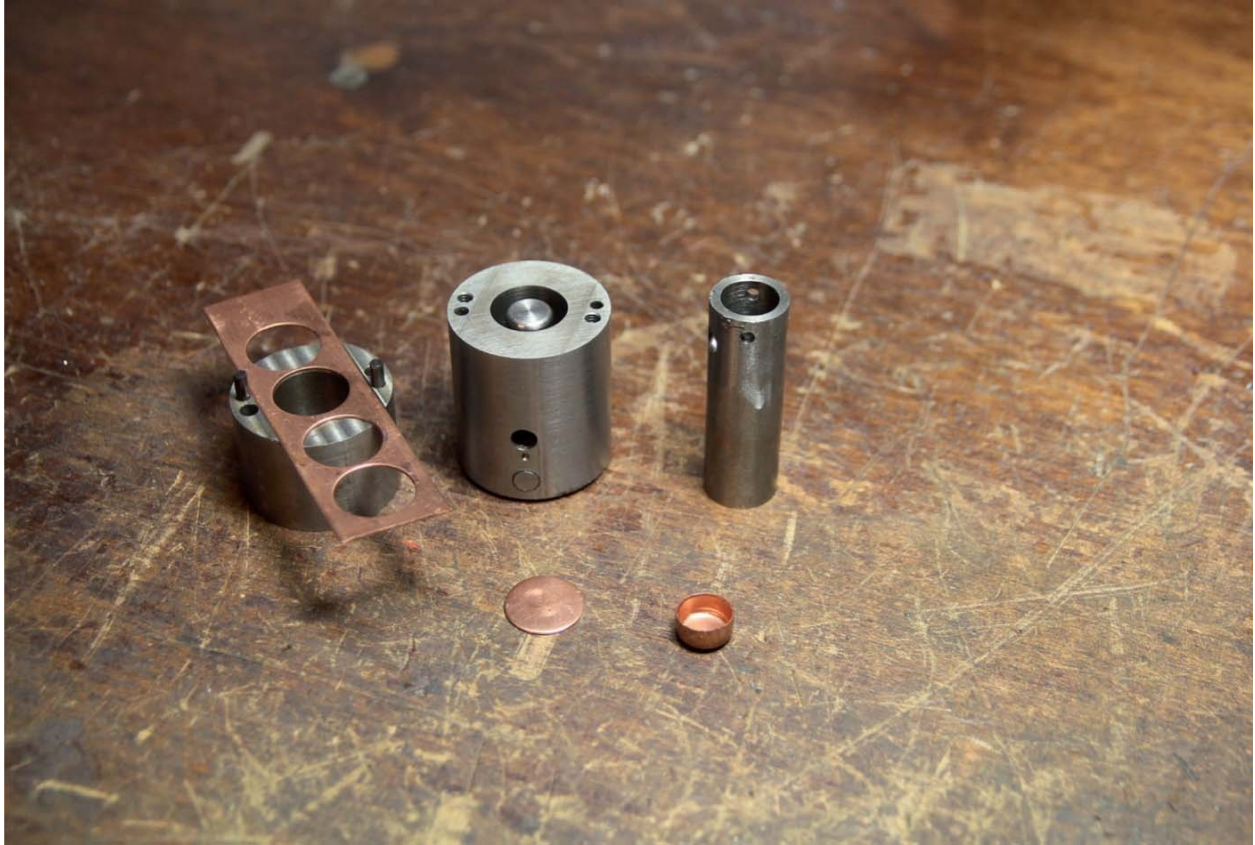
Fig. 9-15: The copper strip is guided inside the upper part of the tool, for blanking. john sanders at nyc cnc.
