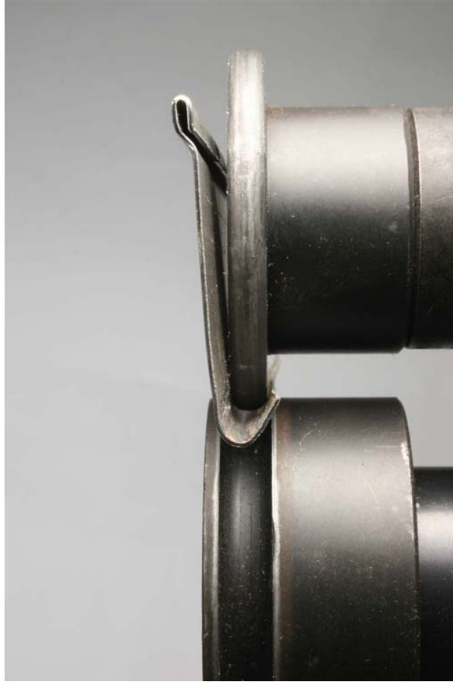
Fig. 7-26: Using beading dies to form a J-shaped edge profile, for wiring an edge.
