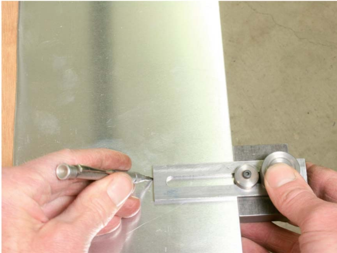
Fig. 3-15: Adjustable parallel scribing guide, which relies on coordinating the movements of both hands.
