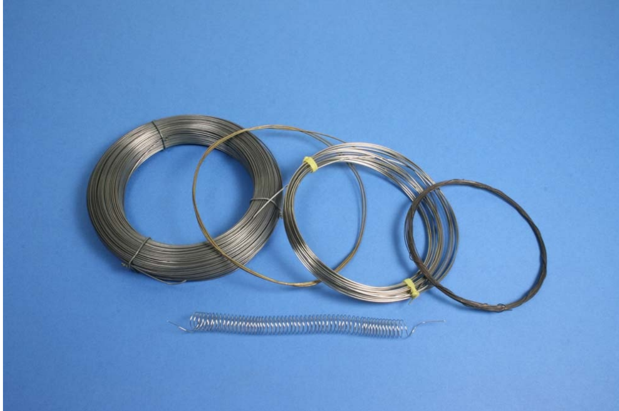
Fig. 1-9: At the rear, from the left: steel, brass, stainless steel and phosphor-bronze wire. At the front: nichrome wire. .
