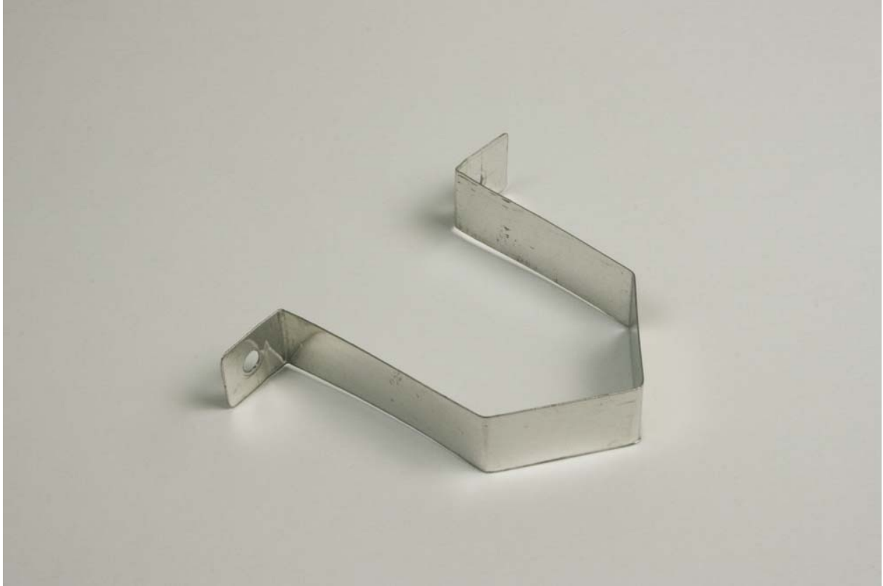
Fig. P1-20: Strap to secure the tank to the flat side of the fuselage.
