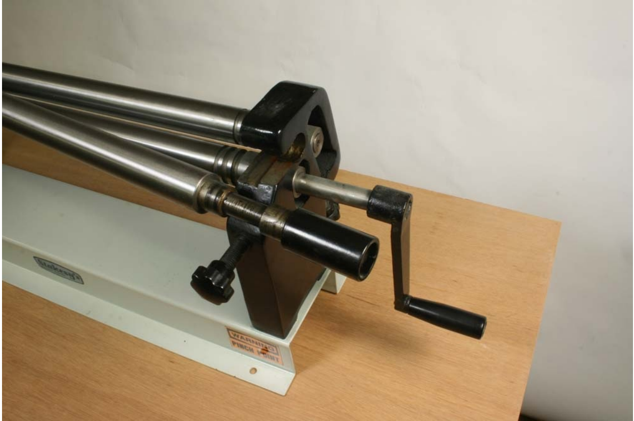
Fig. 7-3: Slip rolls allow the top roll to be swung free, to allow tightly curved work to be removed.
