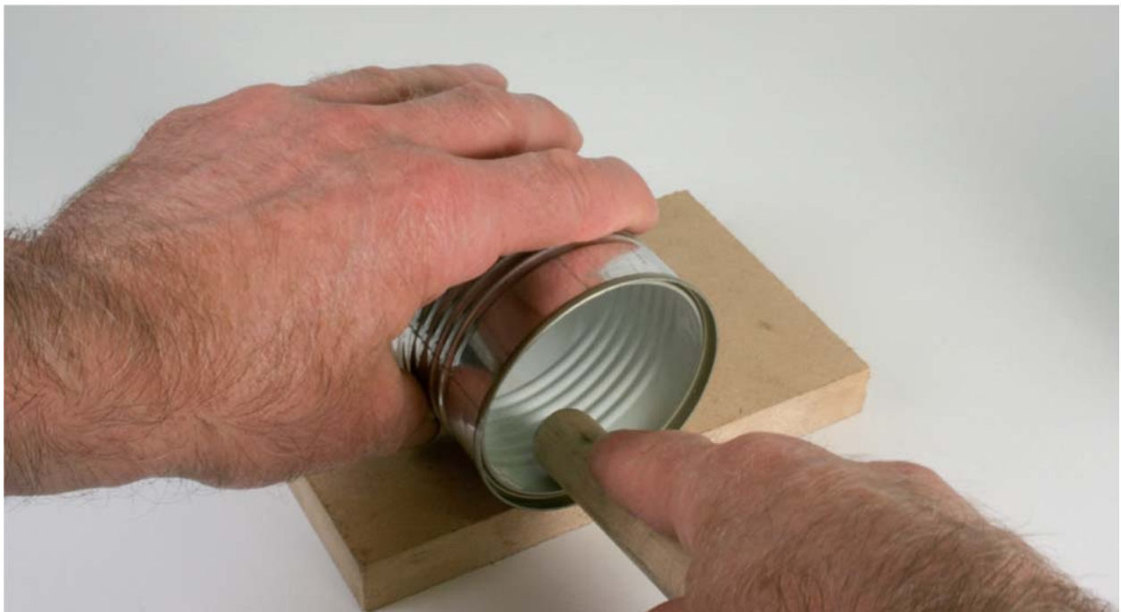
Fig. P2-5: Bumps can be pressed out and smoothed from inside, using a dowel.
