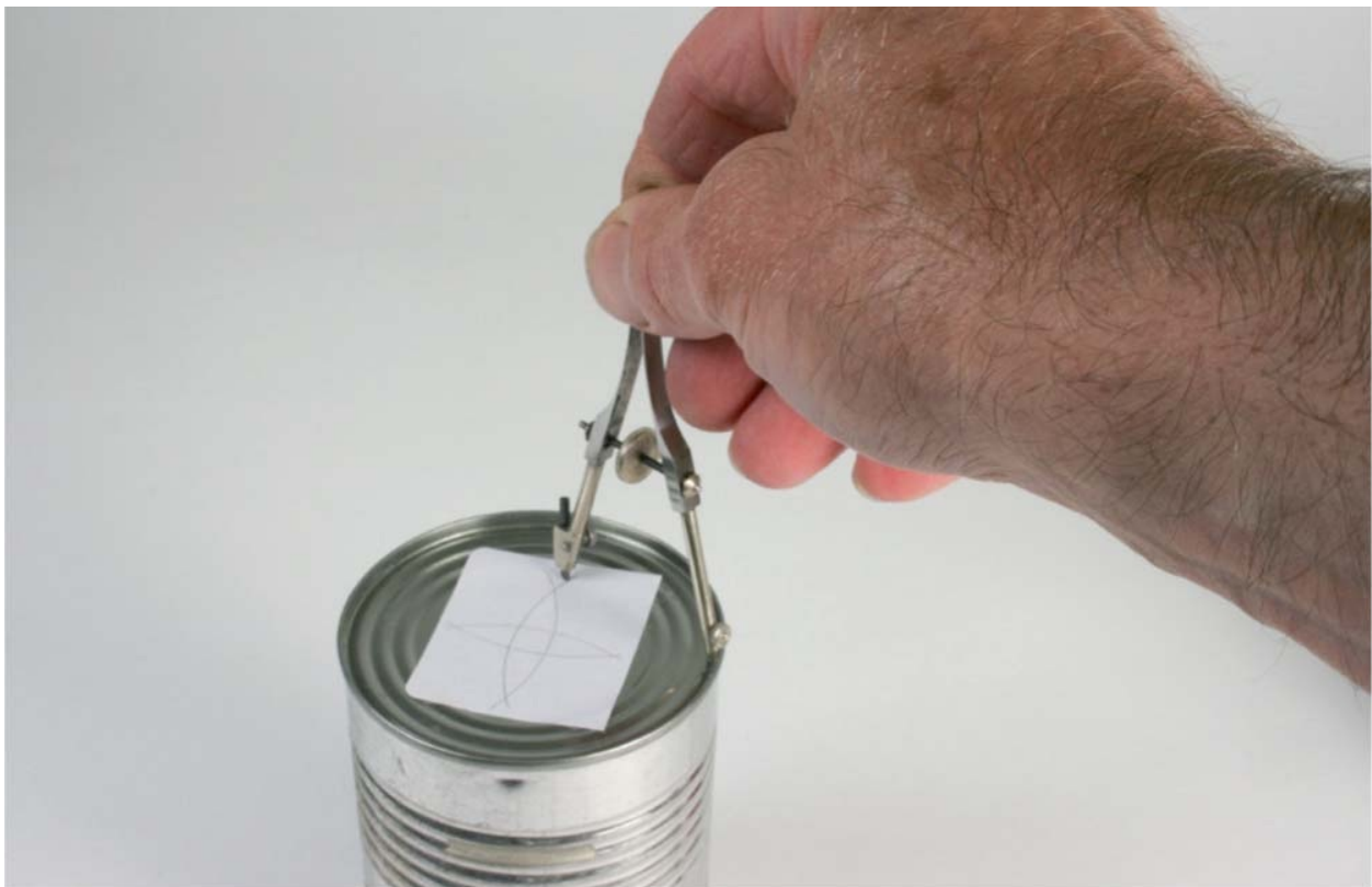
Fig. P2-6: Scribing arcs using a compass.
