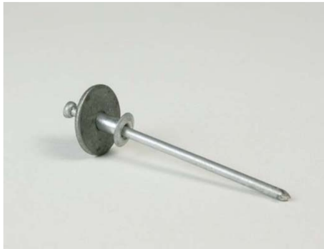
Fig. 8-32: A pop rivet can be set with a large washer under its head to spread the pressure when gripping soft materials.
