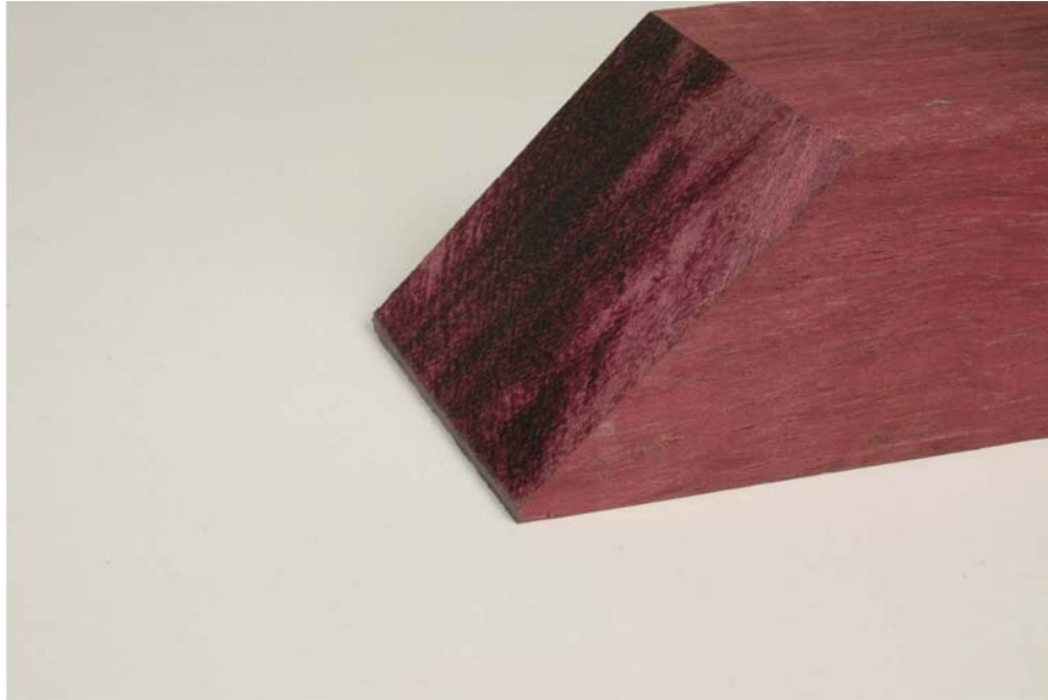
Fig. 7-25: Small flat on the nose of a hardwood striker.
