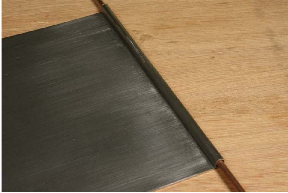
Fig. 7-24: Finished wired edge.
