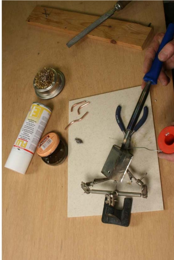
Fig. P1-18: Soldering the seam between the side and the bottom of the tank.
