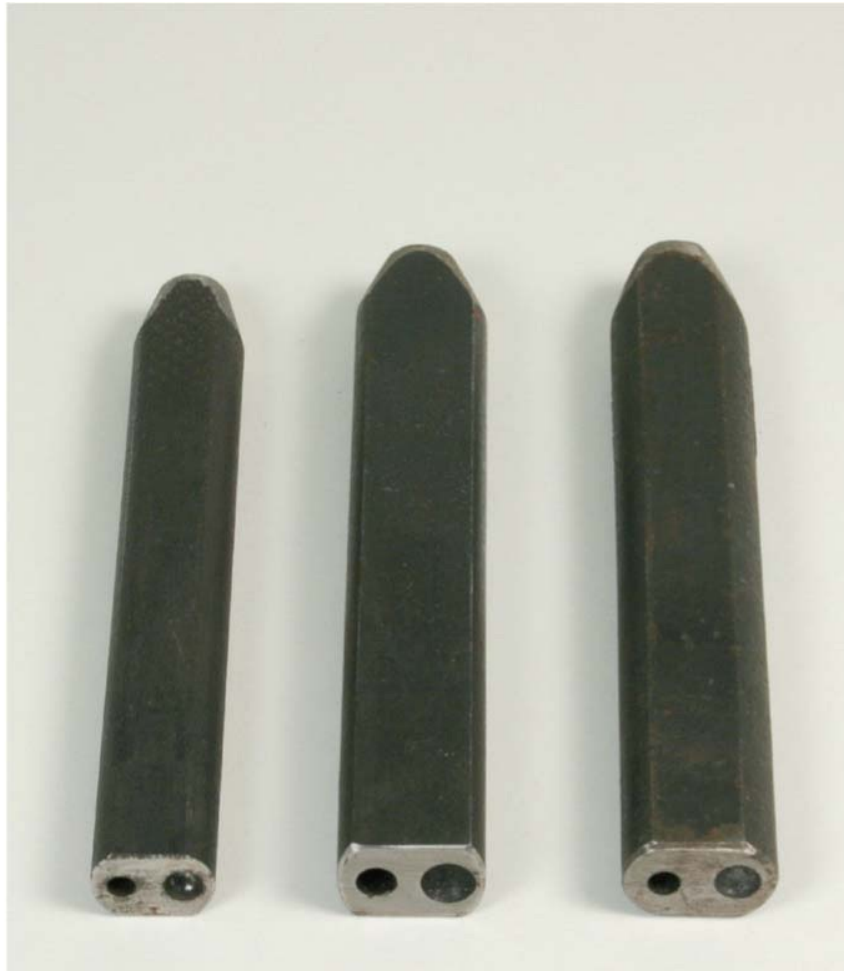
Fig. 8-18: Combined setts (the plain hole) and snaps (the domed recess) for each of three sizes of rivet.
