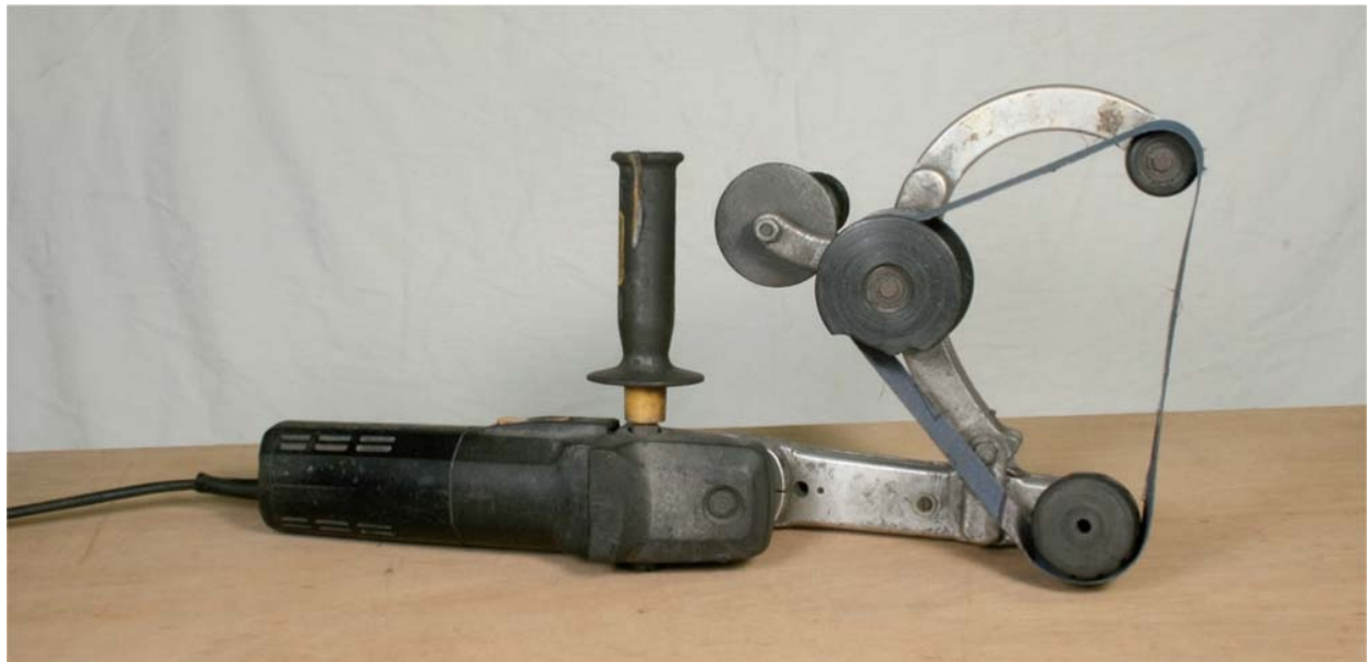
Fig. 10-8: A belt grinder for tubes and convex surfaces.
