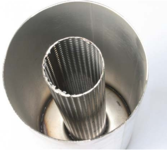
Fig. P5-7: The longer of the perforated tubes is welded into one end of the outer tube so that its free end is flush with the end of the chamber.
