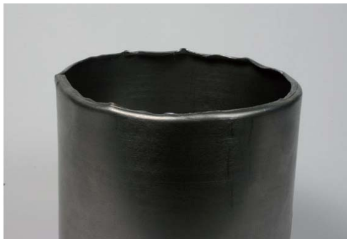
Fig. P4-14: First stage in creating the flange on the end of the sleeve.
