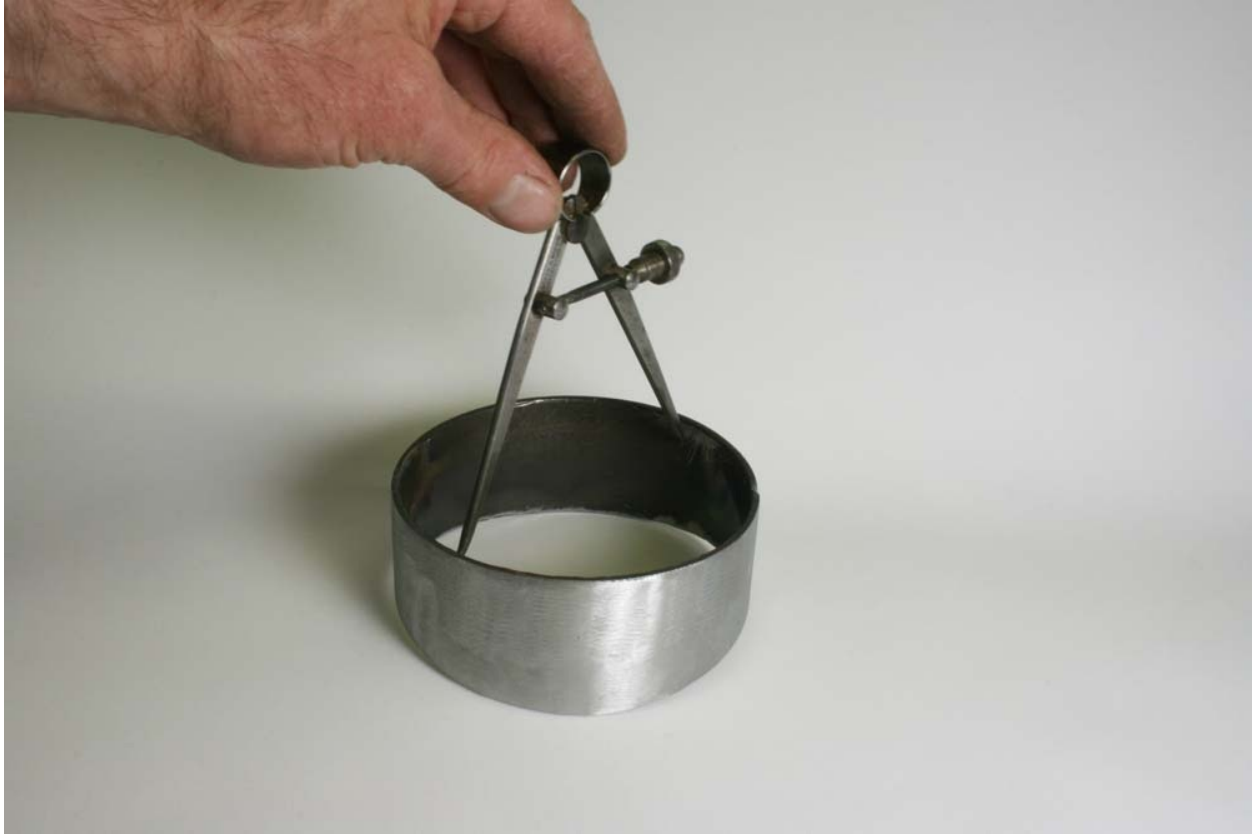
Fig. P4-8: Checking the external tube for ovality.
