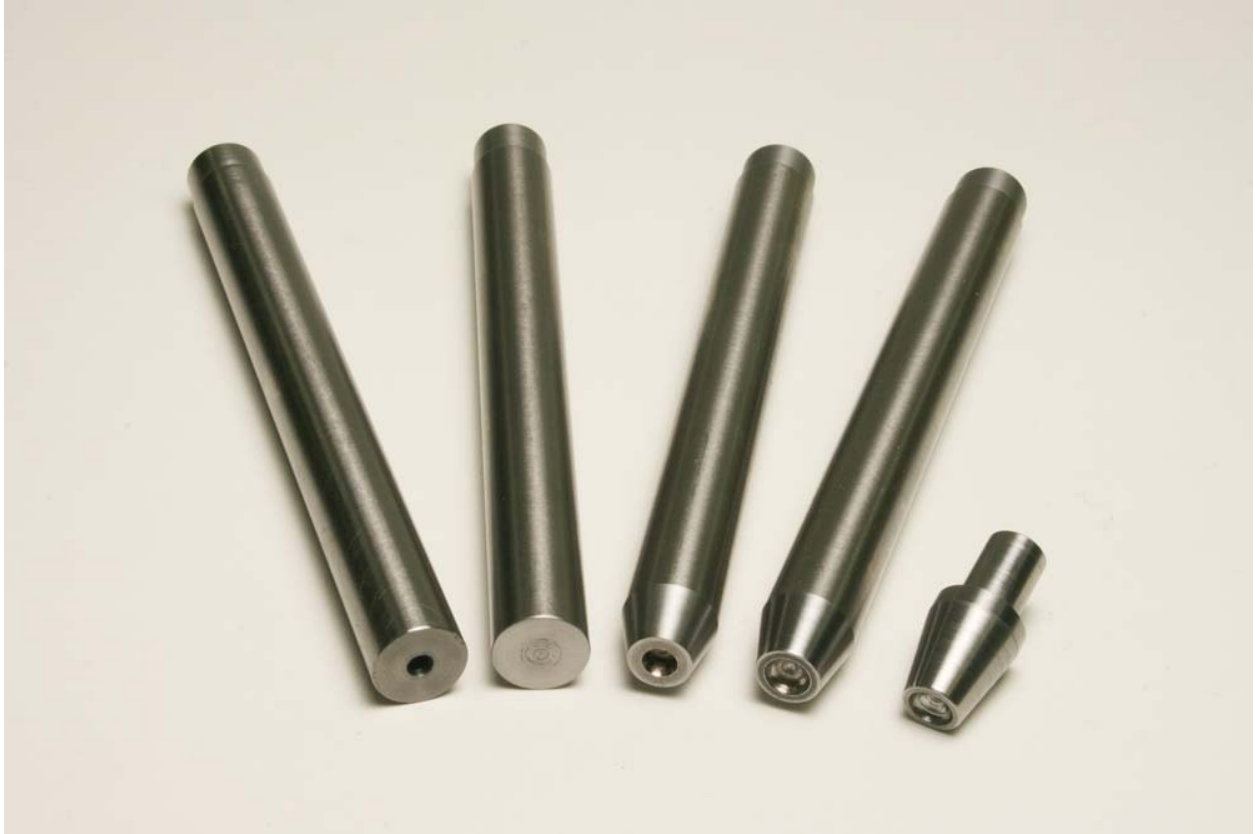
Fig. 8-19: Left to right: a rivet set (sometimes spelt 'sett' for his-torical reasons), a flat tool (flatended punch), a cone tool (conical punch), a snap (rivet head punch), and a stake to support a rivet head in a staking tool.
