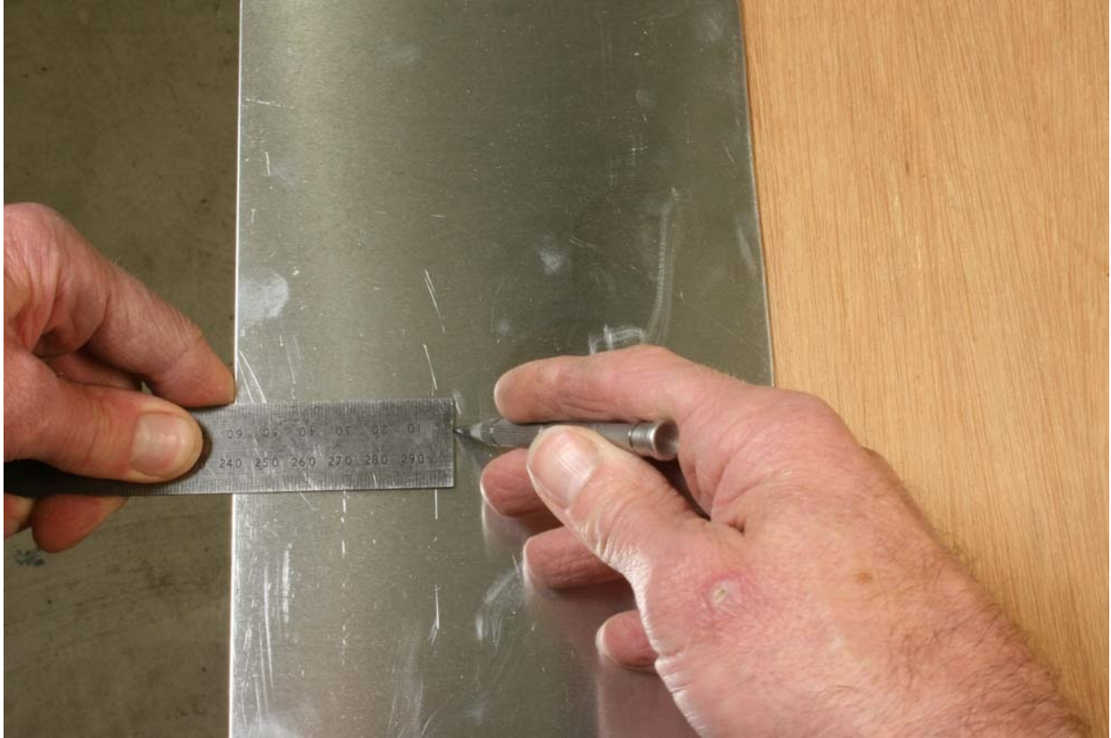
Fig. 3-17: Using a ruler to mark an offset line.
