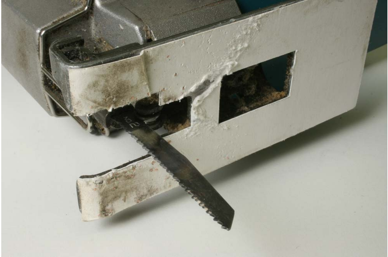
Fig. 4-27: Card on the base of a jigsaw, to protect the metal being cut.
