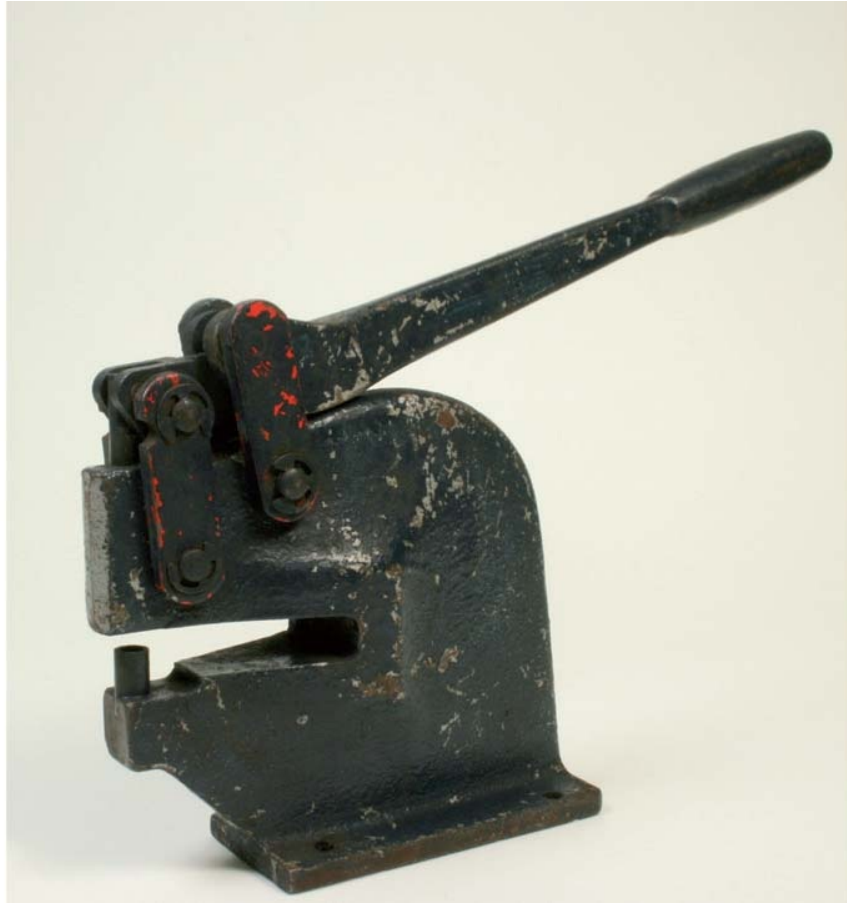
Fig. 5-11: Small toggle press used to punch holes.
