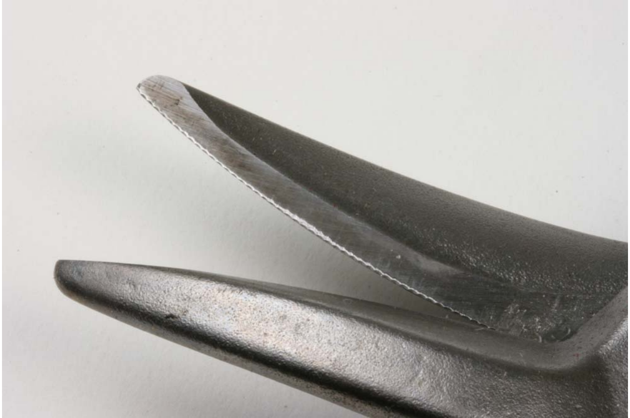
Fig. 4-6: Serrations on the jaws of aviation snips.
