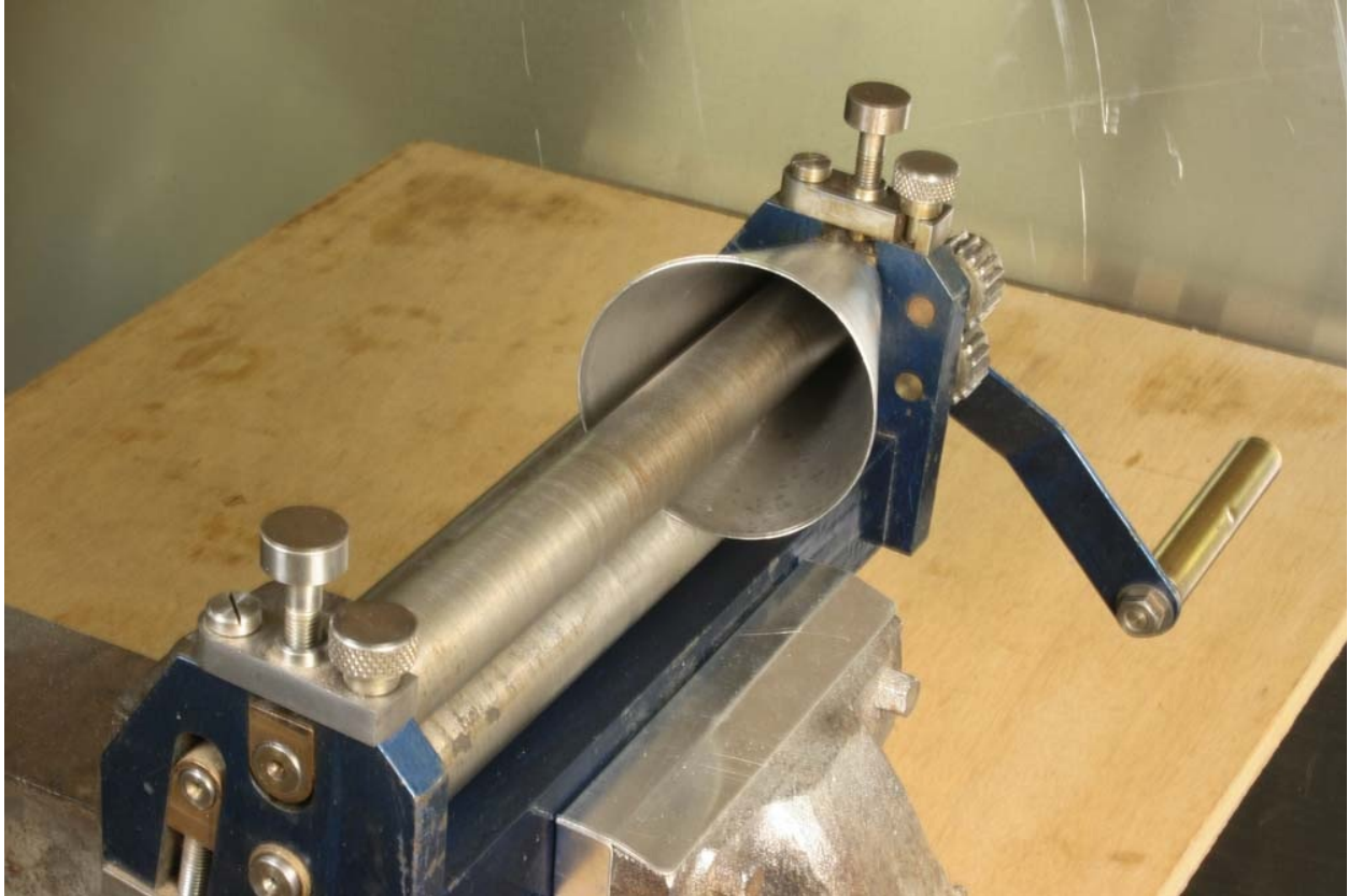
Fig. 7-4: The minimum diameter of a truncated cone is dictated by the diameter of the roller. Use slip rolls, where the top roller can be removed, to release the cone.
