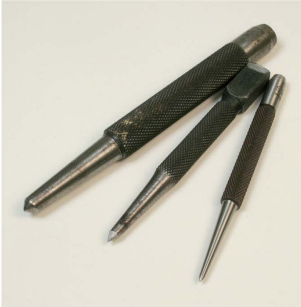
Fig. 3-20: Right to left: Pricker, standard 60-degree and heavy duty 90-degree point centre punches.
