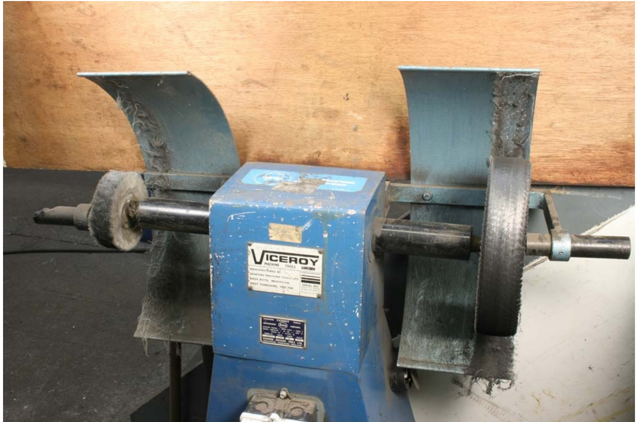
Fig. 10-18: A powered buff with a range of mops may be used, along with different grades of abrasive paste to impart a high polish by holding the work against the rotating mop.
