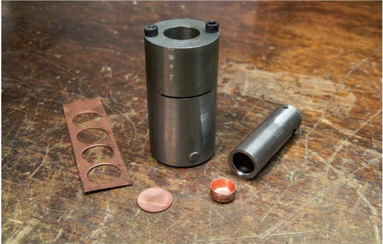
Fig. 9-12: Component parts of the NYC CNC blanking and deep drawing tool, showing the main body, blanking and drawing punch, a punched strip, flat circular blank, and drawn cup. john sanders at nyc cnc.
