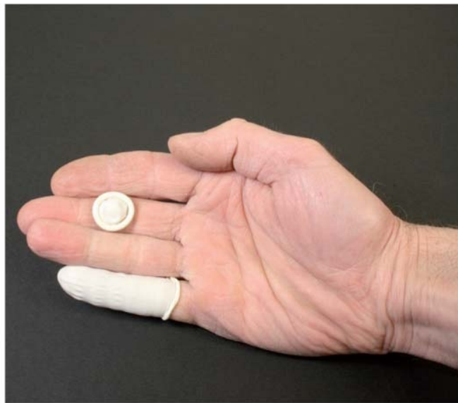
Fig. 10-22: Finger cots should be worn before handling polished work.
