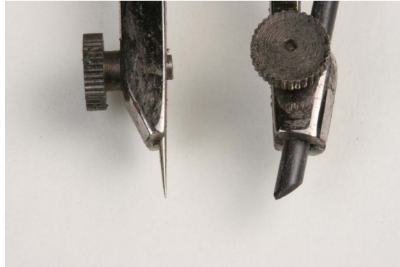
Fig. 3-12: Sharpen a compass lead by giving it one sloping face.
