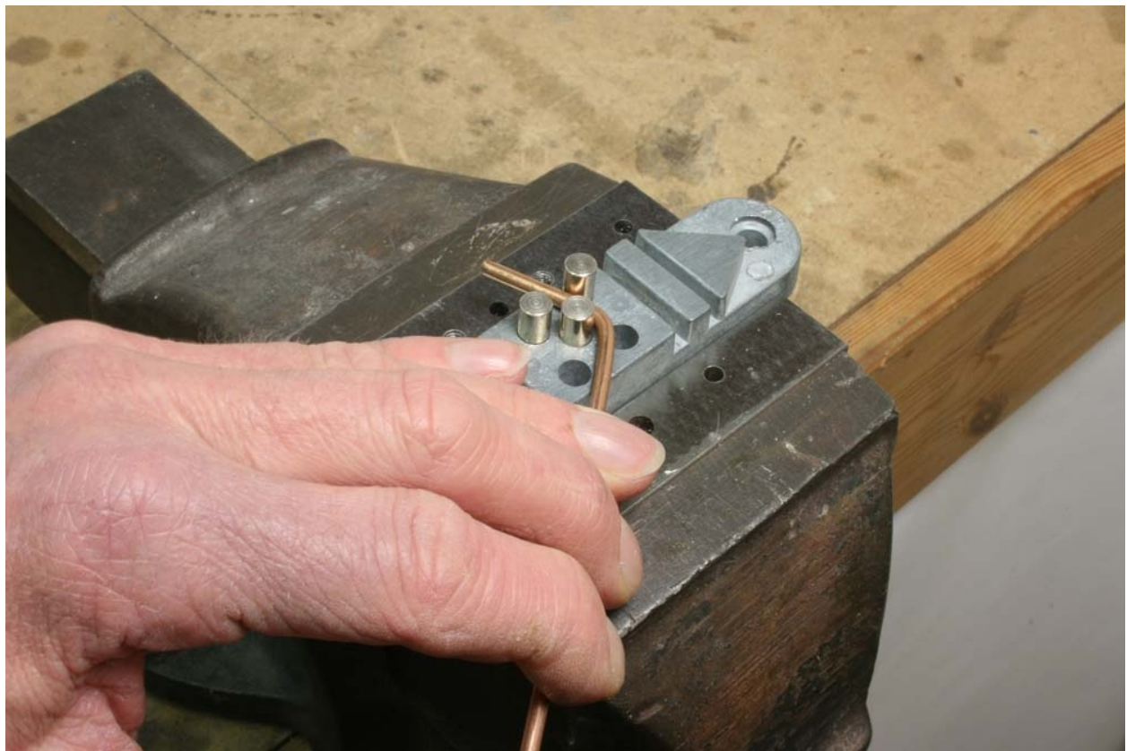
Fig. P7-24: The ends of the wire struts can be bent in a simple multi-purpose jig.
