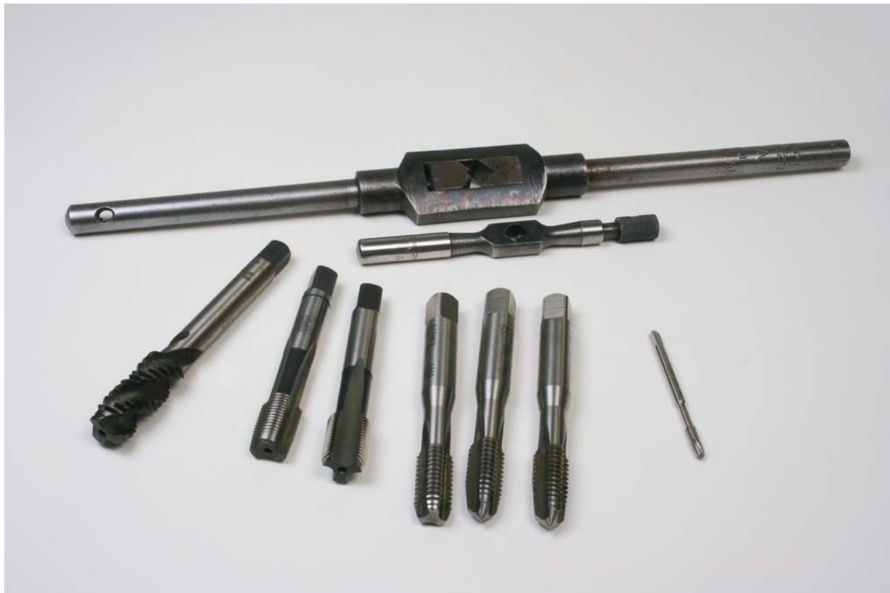
Fig. 8-4: Left to right, bottom row: spiral machine tap, two geometric (progressive) taps, a set of three hand taps (bottoming, second and taper), and a small partially fluted tap. Above the taps are tap wrenches.
