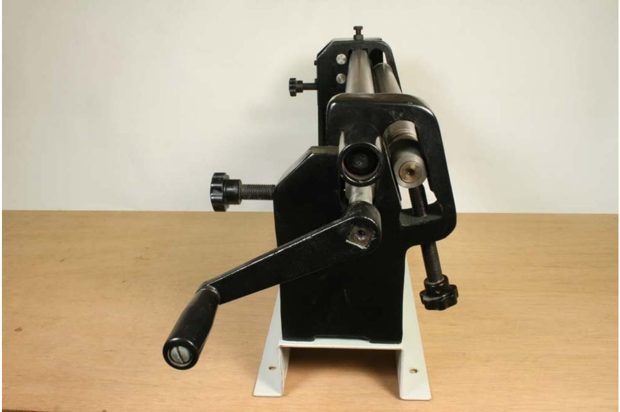
Fig. 7-2: The rear roll has a height adjuster at each end (the knob on the right of the photo). The gap between the two front rolls can be altered, to vary the grip (the knob on the left side of the rolls).
