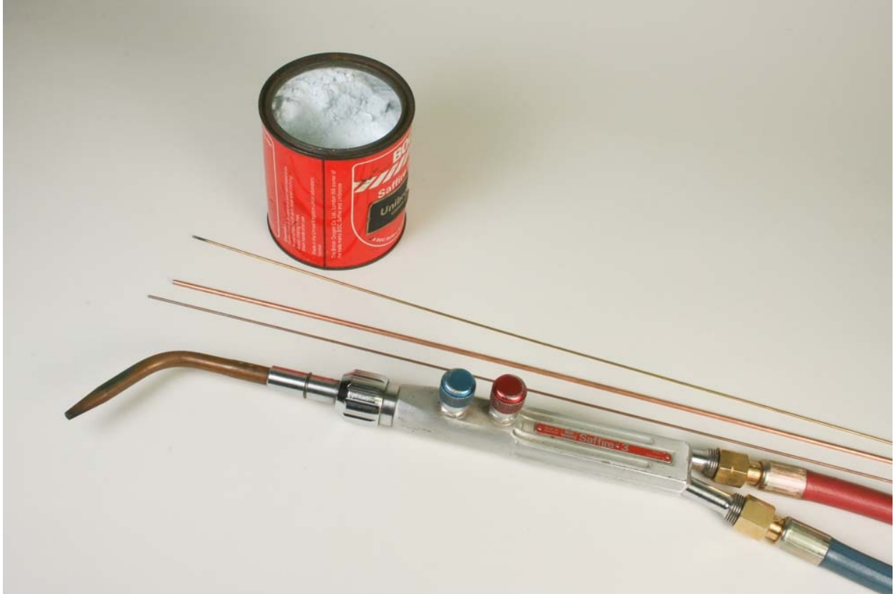
Fig. 8-45: Oxyacetylene torch, copper-coated steel filler rods, brass filler rod and flux used for brazing and bronze welding as well as silver (hard) soldering.
