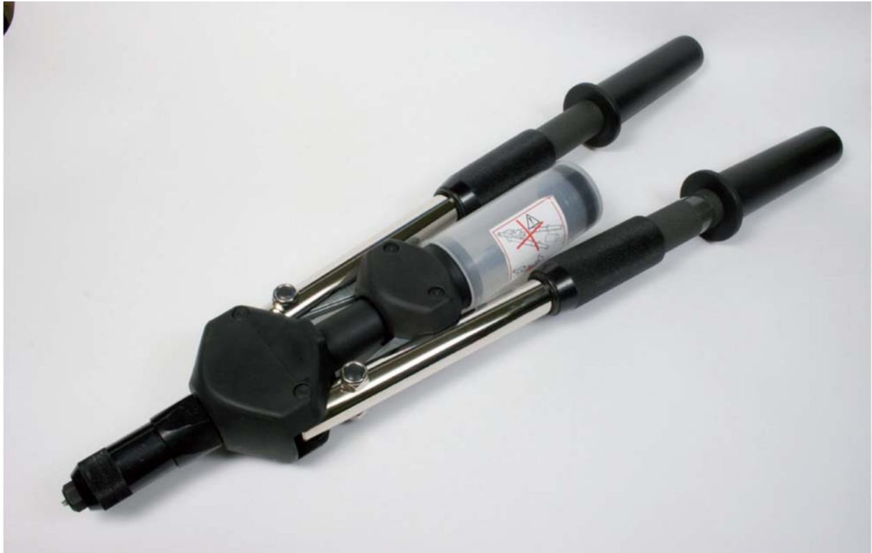
Fig. 8-28: Long-handled rivet pliers used to clench the larger pop rivets.
