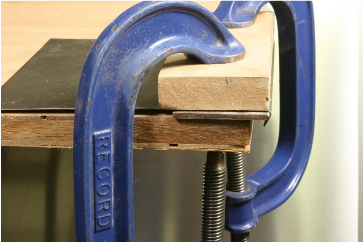
Fig. 7-20: Wired edge: fold over a radiused former.
