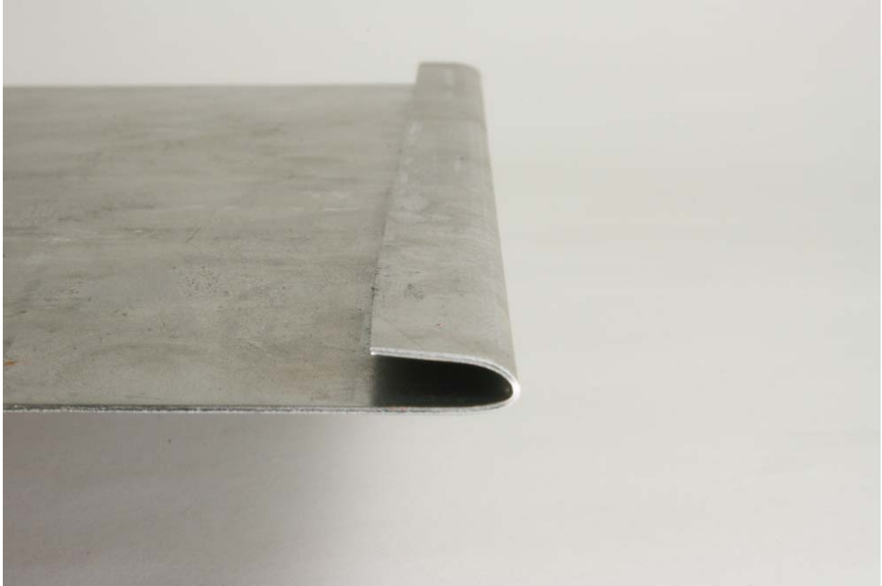
Fig. P6-10: Complete the safe edge by flattening the bent lip.
