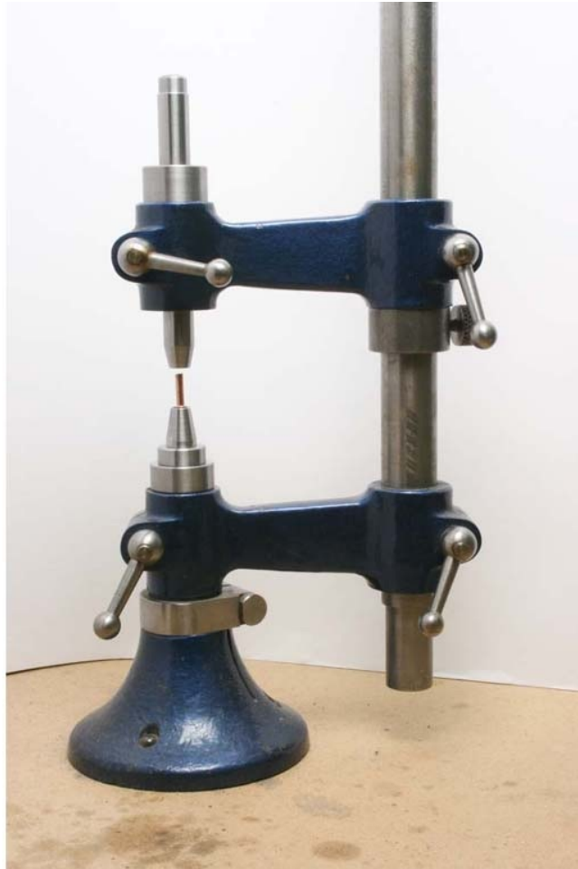
Fig. 8-20: A rivet balanced in a staking tool, for illustration, with a stake underneath to support the head, and a punch above, to form the tail.
