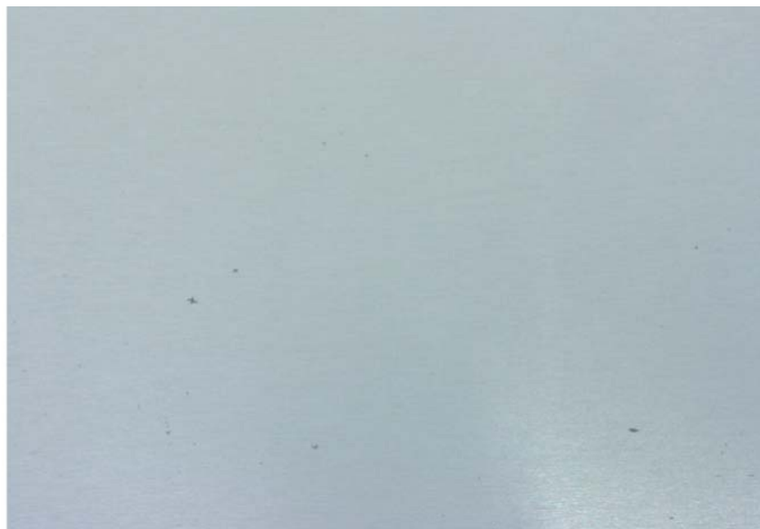
Fig. 6-16: The 'grain' of a sheet may be visible: in this photograph it runs left to right.
