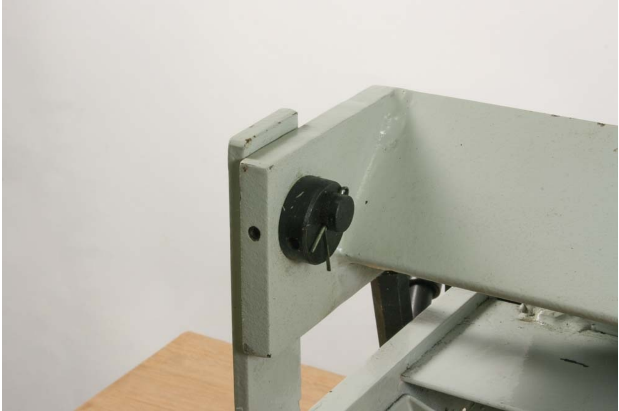
Fig. 6-13: Backset adjustment eccentric collar, with grub screw lock.
