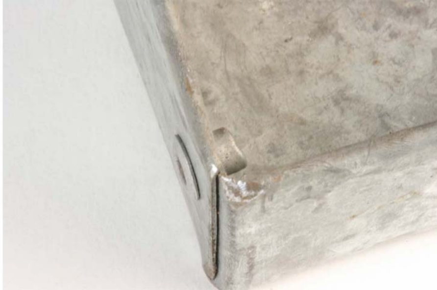
Fig. 8-27: The corner of a tray, secured by a pop rivet.
