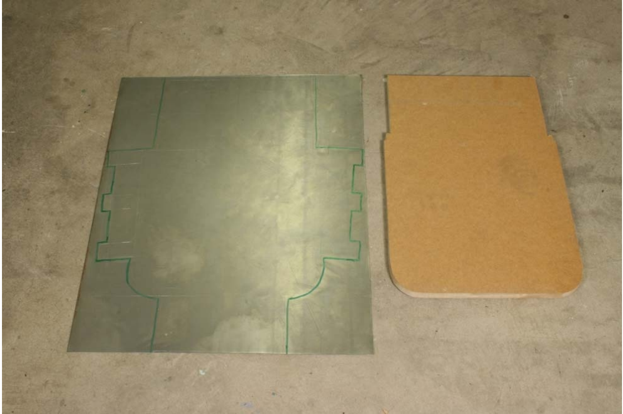
Fig. P6-4: Marked-out sheet, with additional pen lines just outside the scribed lines, as a safeguard.
