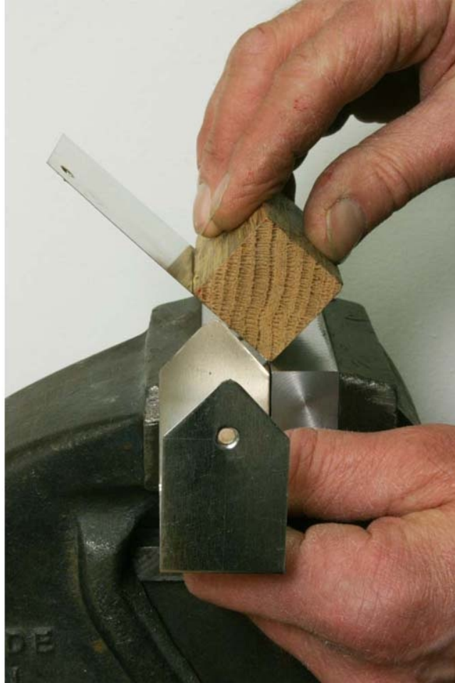
Fig. P1-10: Making the bottom/front fold to match the angle of the taper on the sides.
