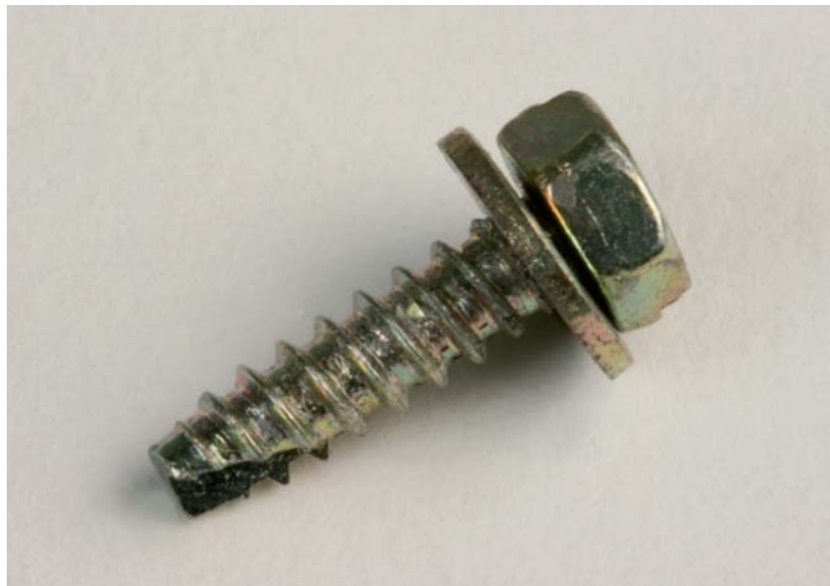
Fig. 8-6: Some self-tapping screws have a gash in the threads at the start, to help cut the threads as the screw enters the material.
