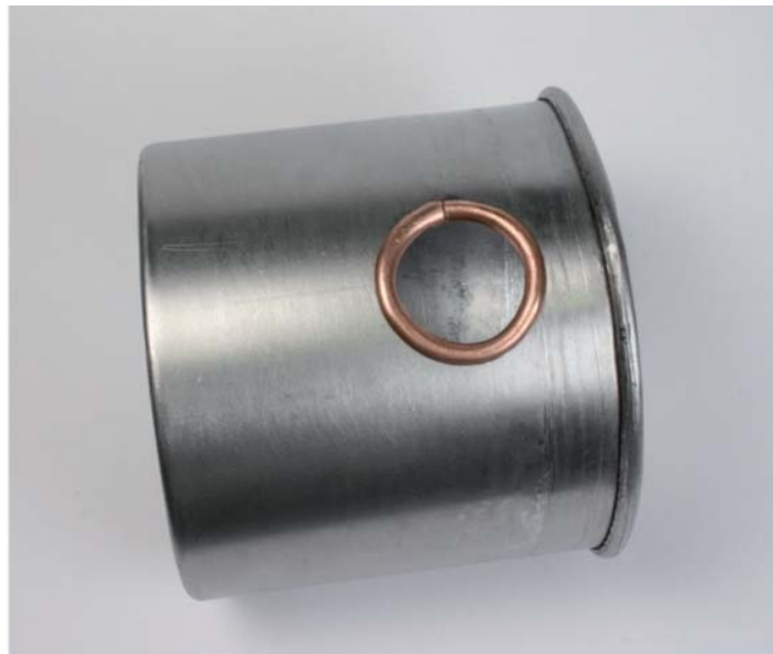
Fig. P4-19: The cut edges of the hole are finished using a length of rolled copper tube slit horizontally around its circumference.
