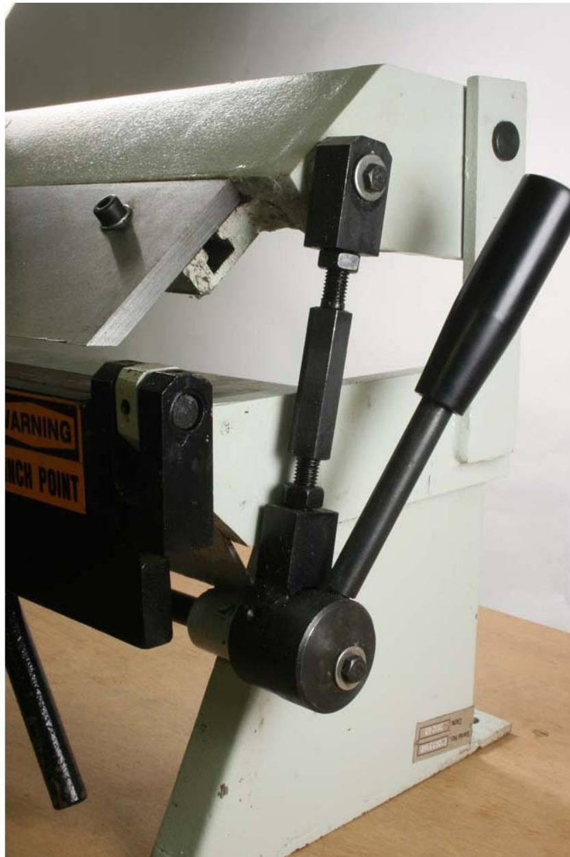
Fig. 6-9: Cam clamping mechanism to control clamping pressure.
