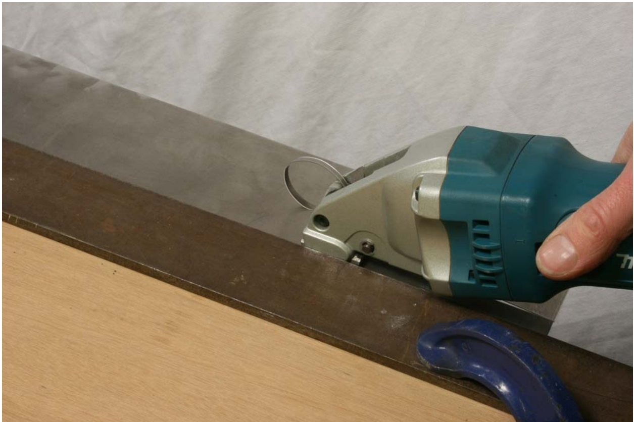
Fig. 4-12: Running shears along a side guide clamped to a sheet.
