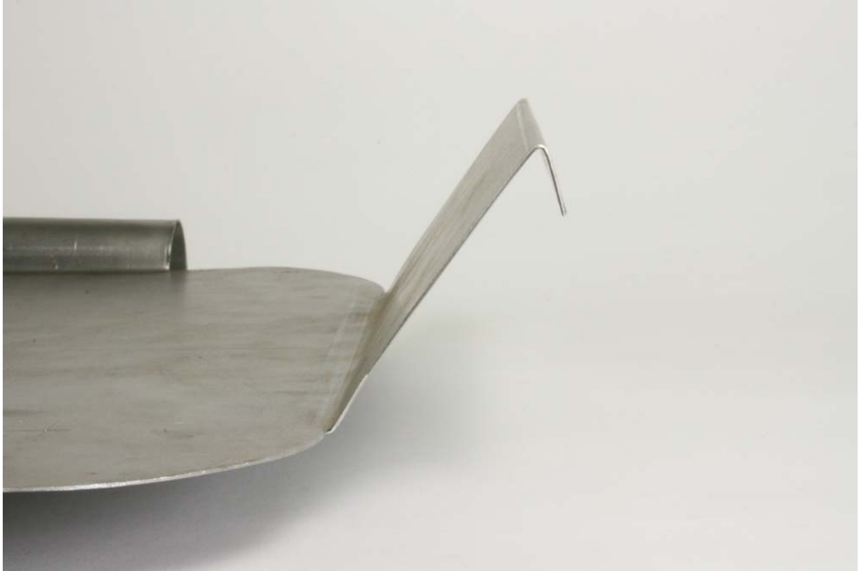
Fig. P6-9: Begin creating a safe edge by folding the edge beyond 90 degrees.
