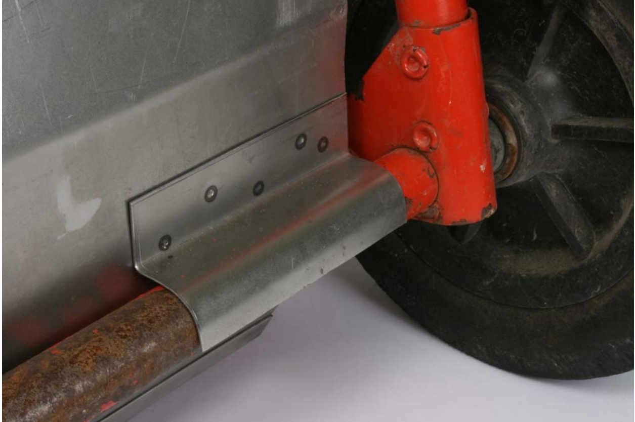
Fig. P6-13: Use a mallet to shape the lower locating brackets over the bottom tube.
