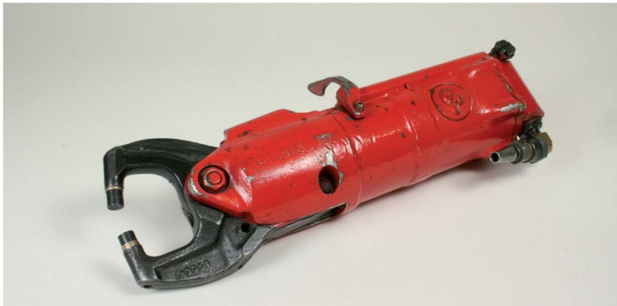
Fig. 8-25: A pneumatic tool for clenching flat-headed rivets by giving them a flat tail.
