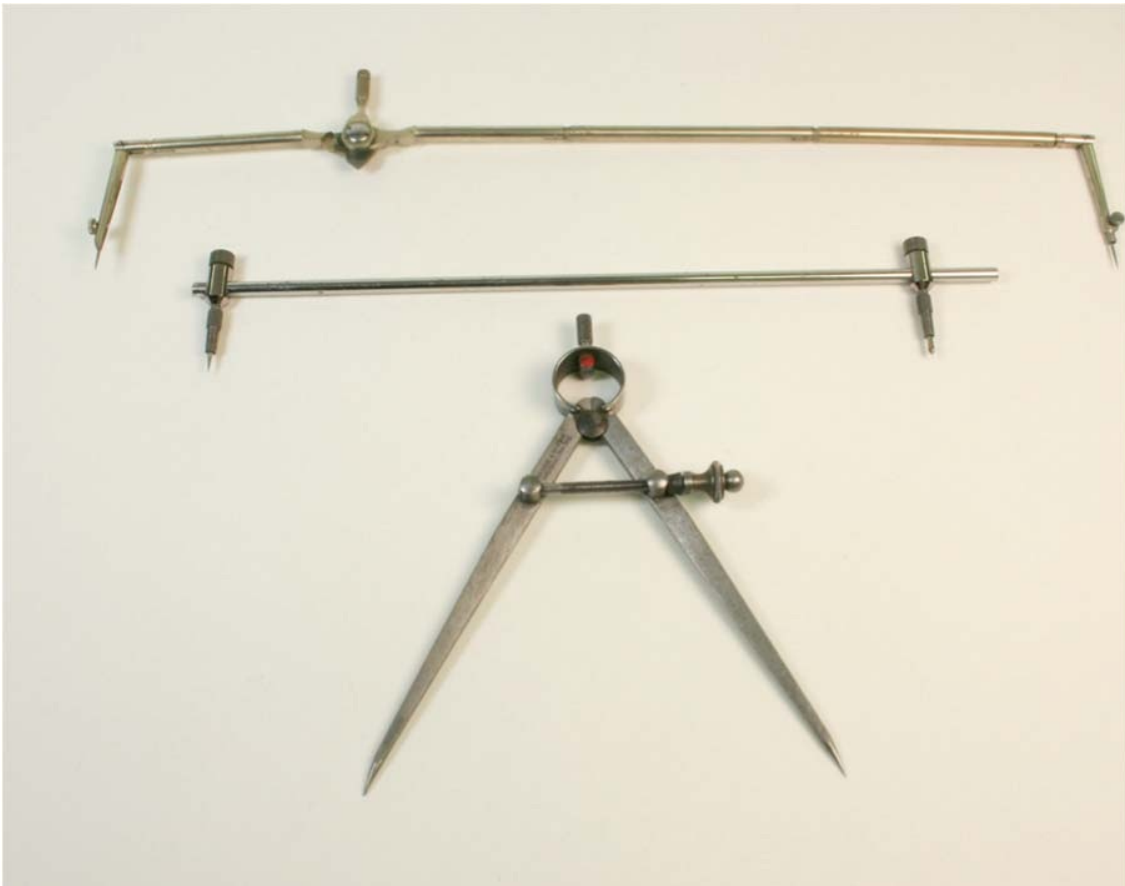
Fig. 3-13: To draw larger circles, trammels or beam compasses locate more securely than widely spread dividers.
