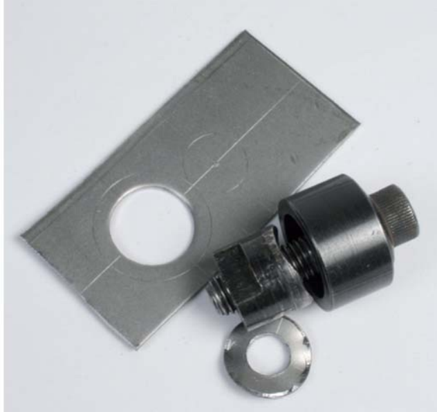
Fig. P2-25: Mark out for the ring-pull tab, then use a Q-Max cutter to punch the larger hole.
