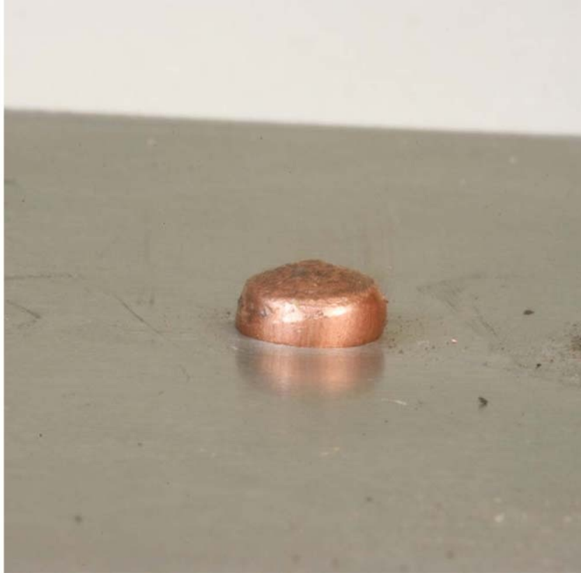
Fig. 8-22: Finished rivet tail.
