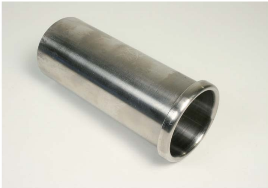
Fig. 9-21: Pusher, tube and ring, with the upturned roll visible at the inner surface of the hole.
