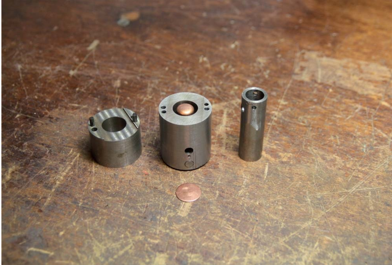
Fig. 9-16: The finished cup, on the top of the pin inside the tool. The copper strip is guided inside the upper part of the tool, for blanking. john sanders at nyc cnc.
