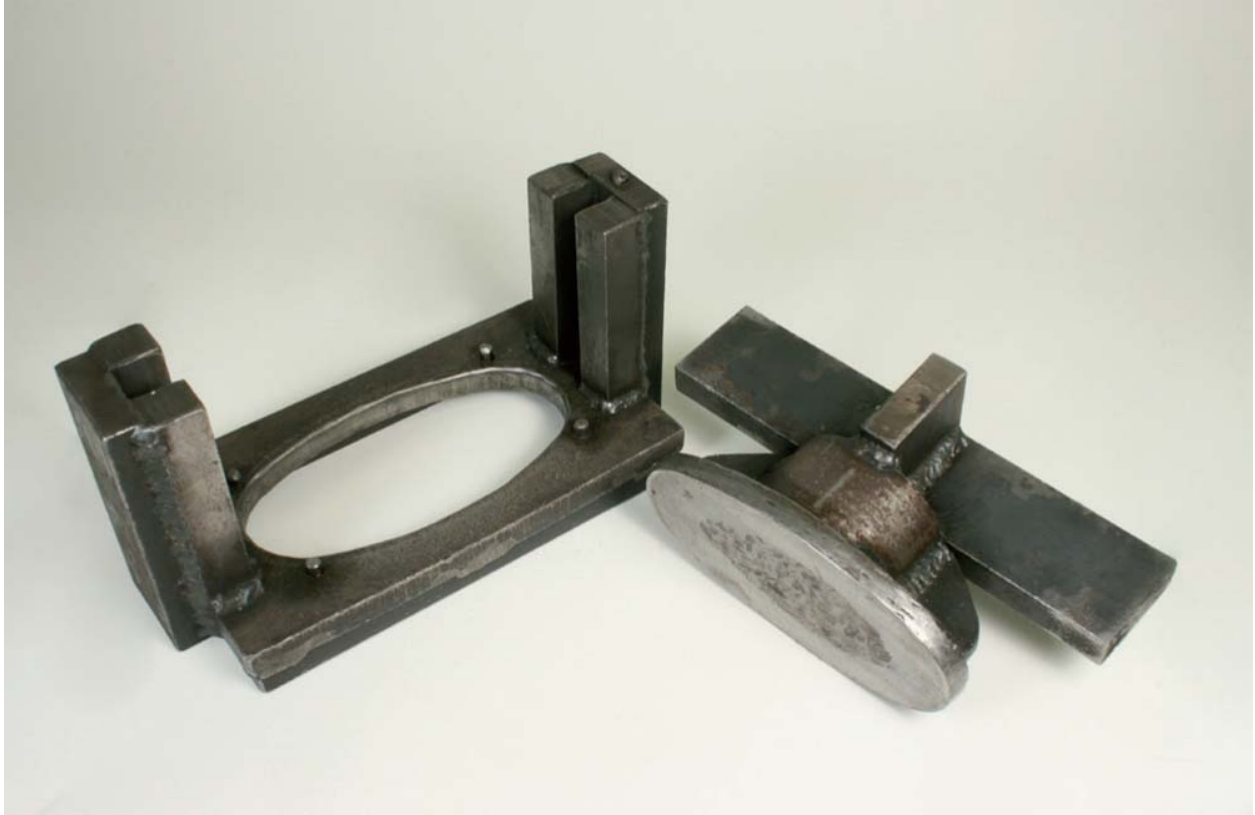
Fig. 9-9: An elliptical flanging tool that will raise a flange around the outside edge of an elliptical blank.
