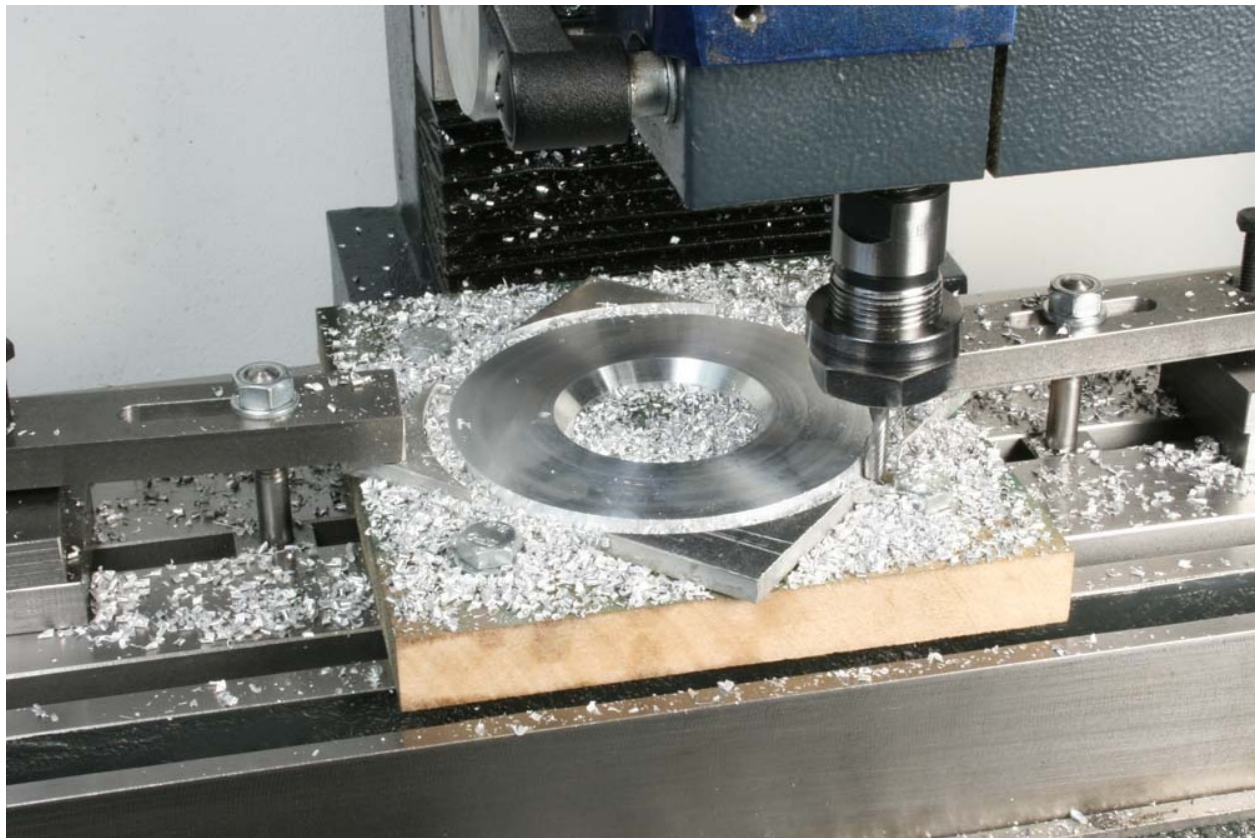
Fig. 5-30: Machining a circular component with a central hole from a 6mm aluminium sheet using a milling machine.
