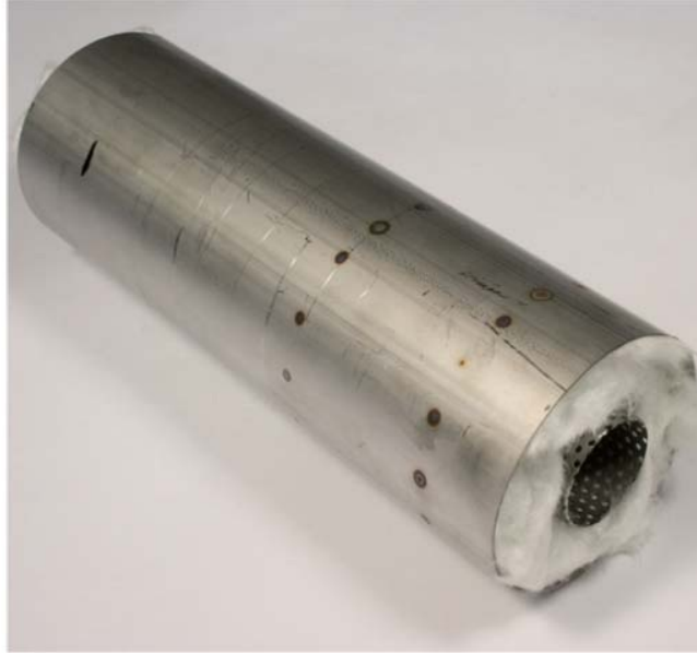
Fig. P5-9: The chamber is packed with Kevlar mat. The internal section between the ends of the perforated tubes was packed before the shorter tube was welded in place.
