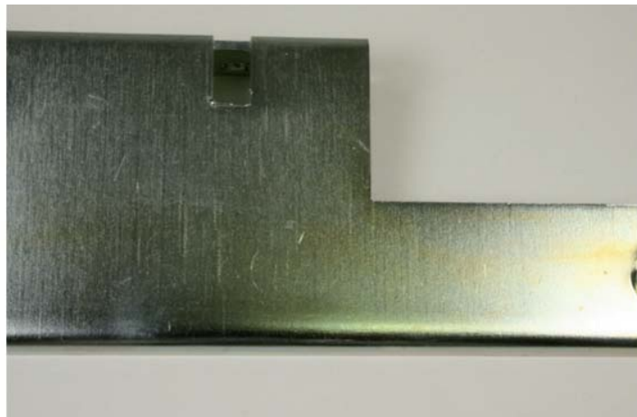
Fig. 10-13: Zinc-passivated steel has a characteristic yellow colour.
