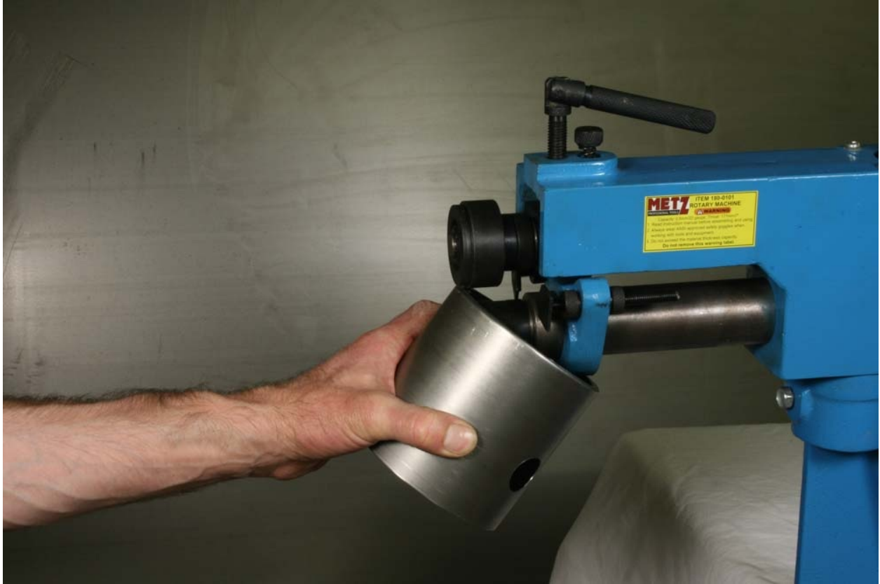
Fig. P4-13: Creating a burr (small flange) using the jenny.
