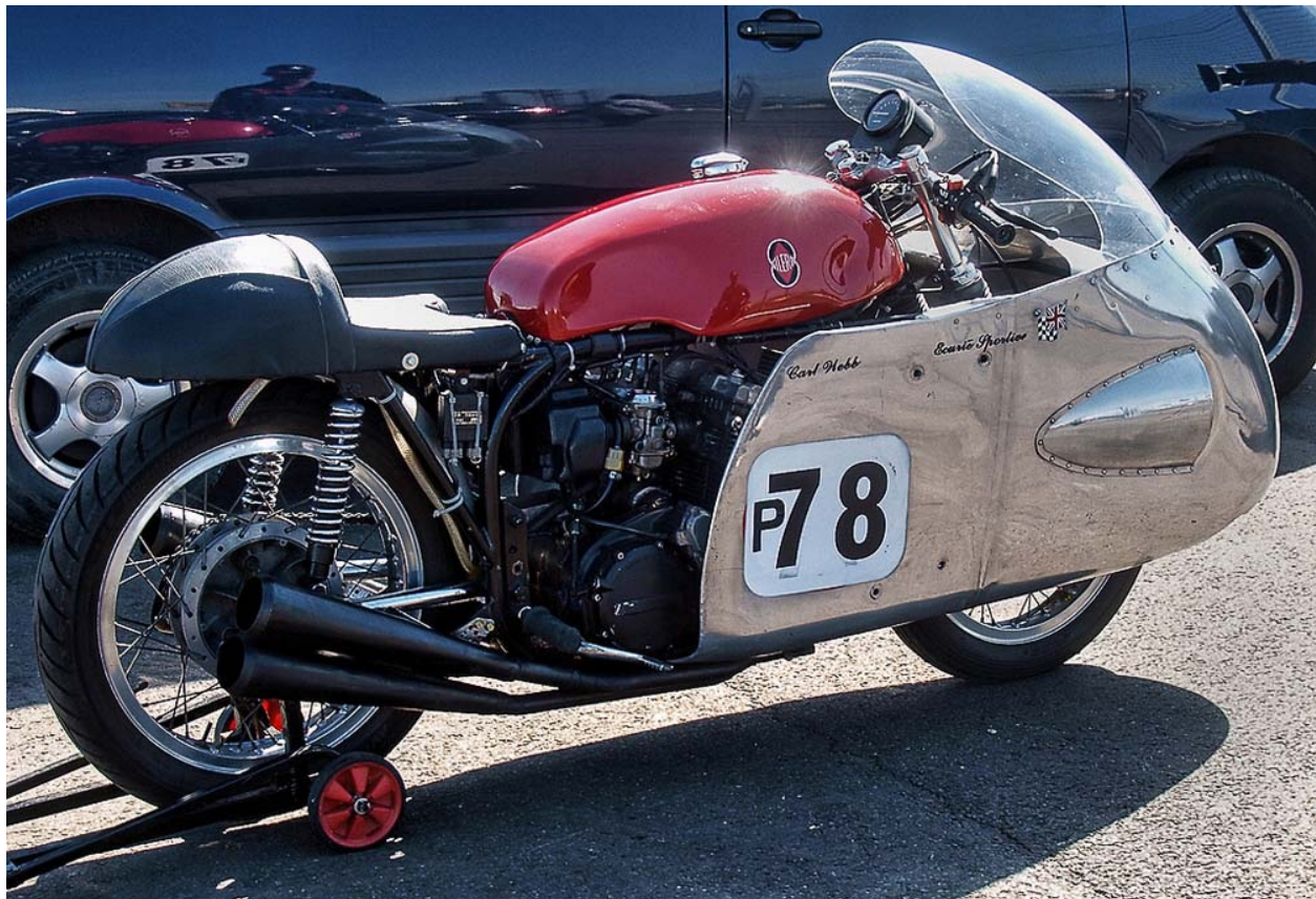
Fig. 8-15: Rivets serve a functional purpose in joining parts together permanently, but they can also be aesthetically pleasing. Photo of the Carl Webb Gilera 500 replica.
