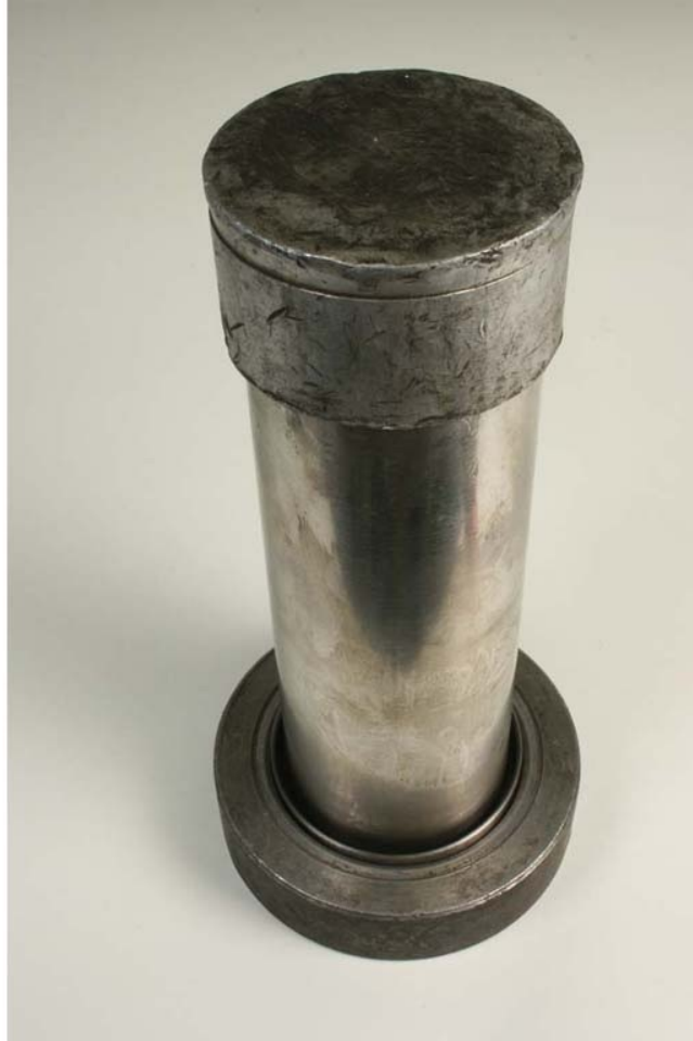
Fig. 9-21: Pusher, tube and ring, with the upturned roll visible at the inner surface of the hole.
