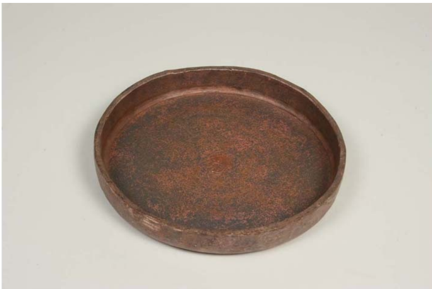
Fig. 9-2: A copper boiler end plate shaped from a flat blank by using a steel former plate.
