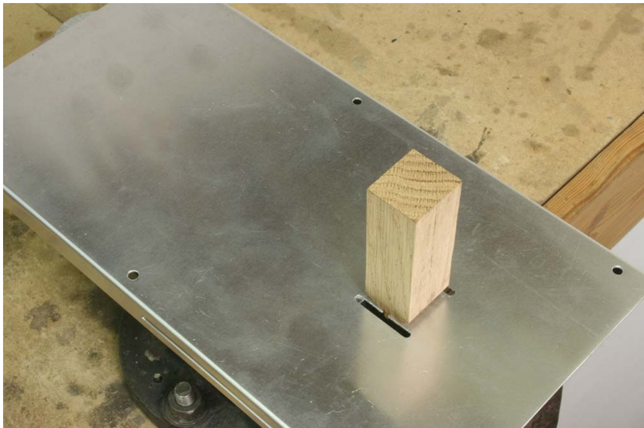
Fig. P7-16: Wooden block in position ready to make the two bends for the spring catch
