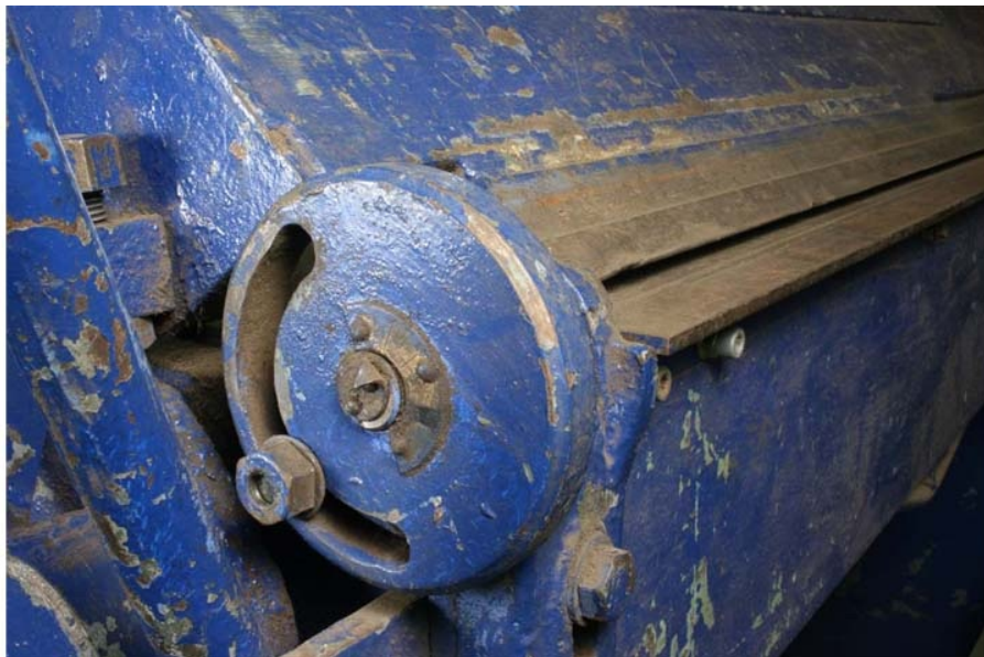
Fig. 6-20: An angle stop (the circular disc) helps ensure accurate folds during repeated operations.
