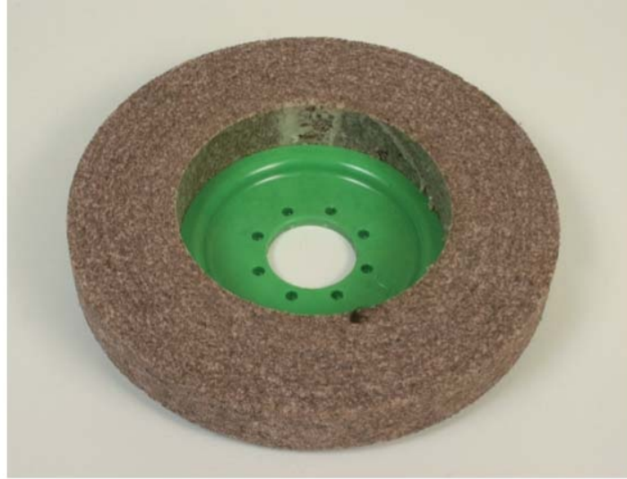
Fig. 10-5: Fine abrasive pads are usually softer and are impregnated with higher-numbered abrasive grits, from 100 to 400 and higher.
