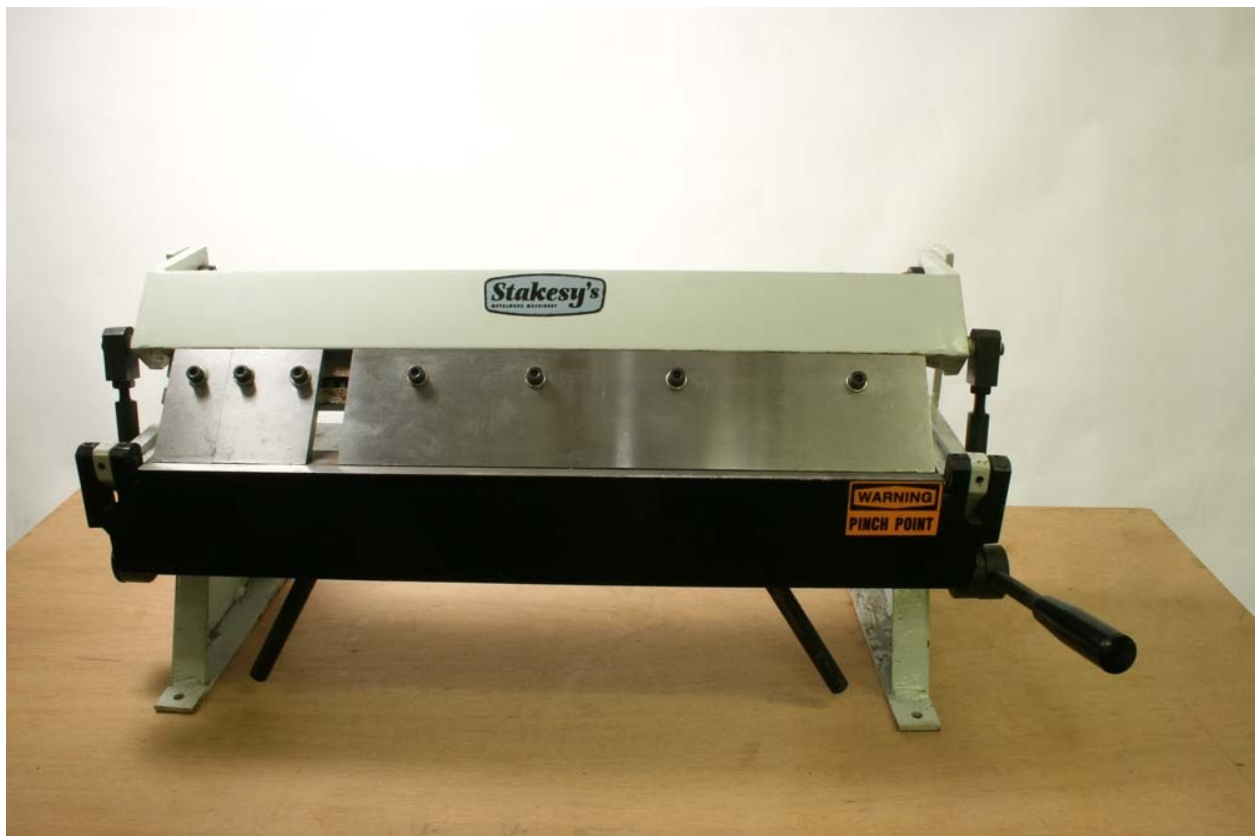
Fig. 6-7: A box and pan folder, with a segmented clamp beam comprising individual fingers of different widths.
