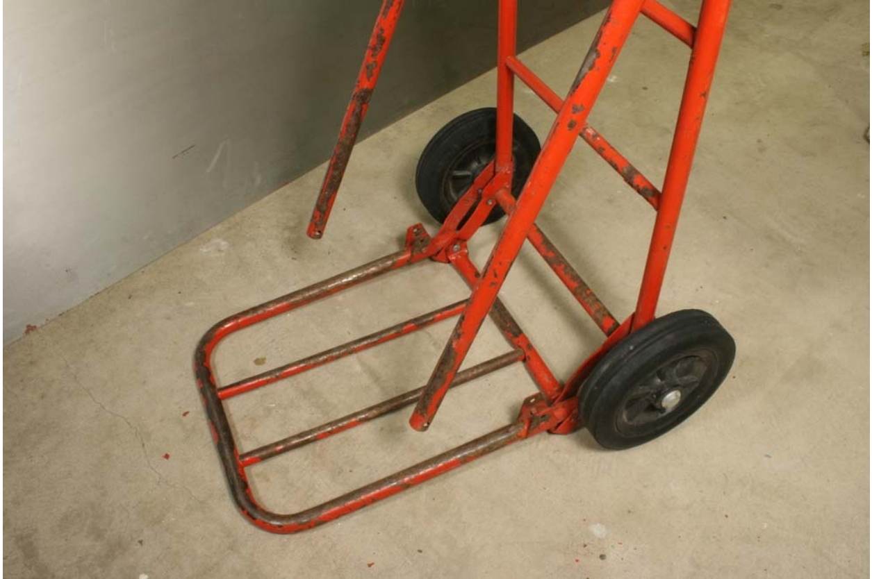
Fig. P6-11: Remove the rivets which hold the bottom of each leg in position, to allow the back panel to be fitted.
