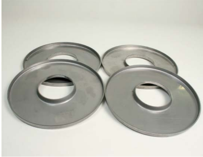
Fig. P5-5: Flanges formed and ready for welding to the tube.
