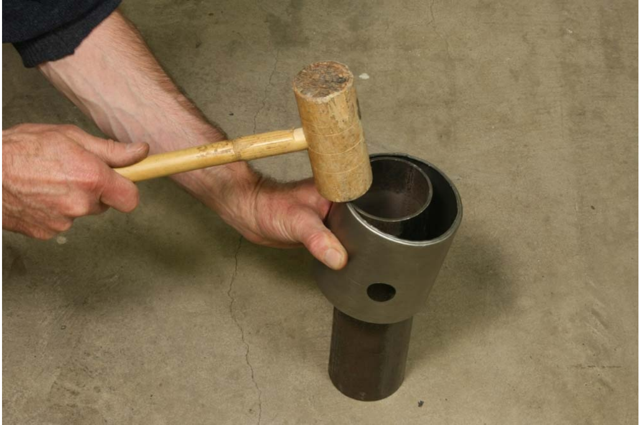
Fig. P4-15: Using an upturned tube as a dolly to finish the flange.
