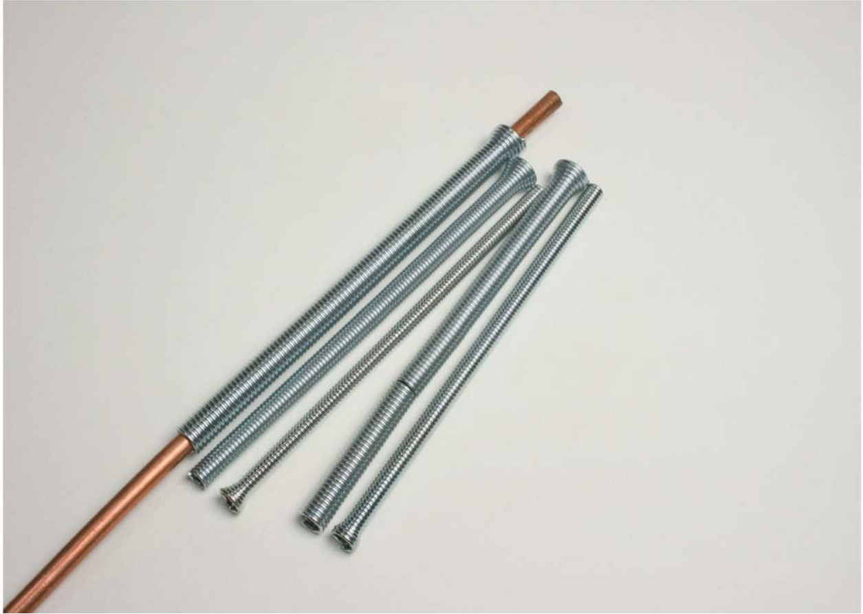
Fig. P1-12: External bending springs to support small-diameter pipe during bending.
