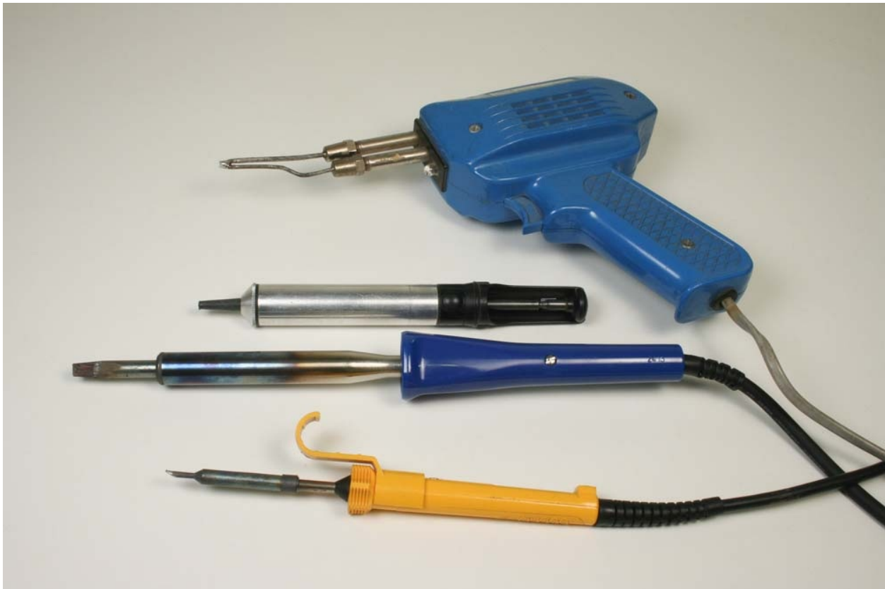
Fig. 8-42: Soldering irons with different heat outputs, and a solder sucker tool.
