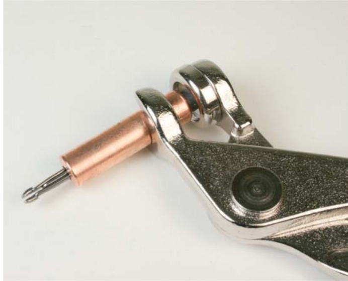
Fig. 8-59: Cleco being operated by pliers, showing the bottom barbs being pushed out beyond the central tongue to allow them to move closer together so that the fastener can slip into a hole.
