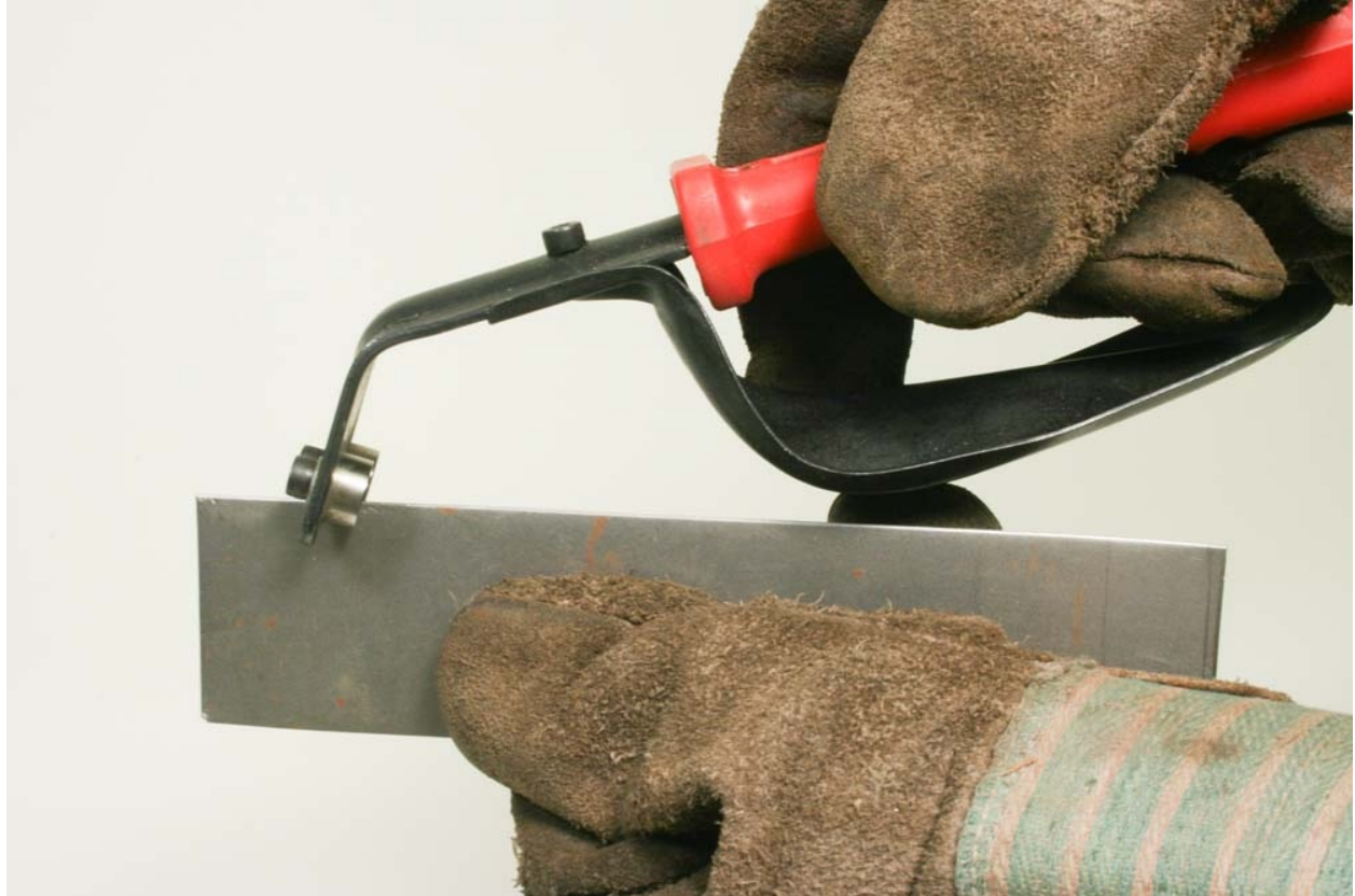
Fig. 4-35: Pull the tool along the edge of the sheet. .
