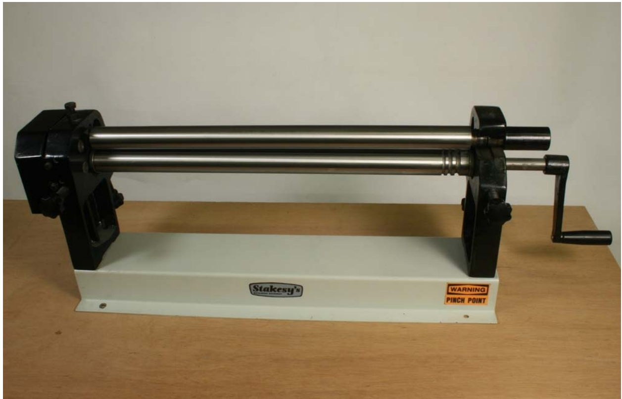
Fig. 7-1: Geared rolls with three rollers. The front two rolls are geared together, and have an adjustable gap. The rear roll is free-running and height-adjustable.
