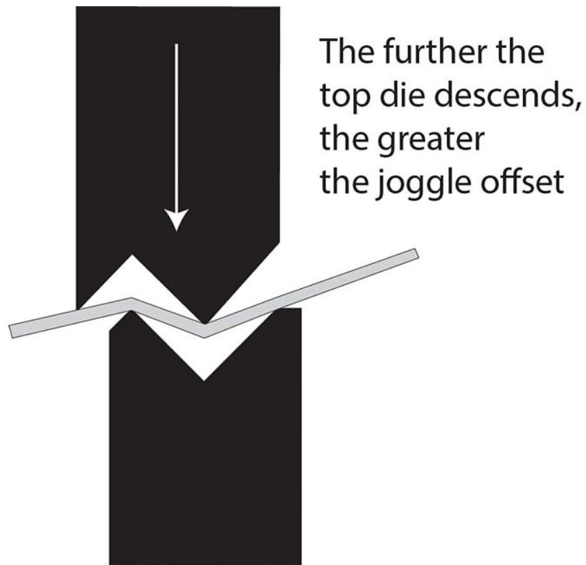
Fig. 8-34: A joggle can be produced in a press brake using appropriate tooling.
