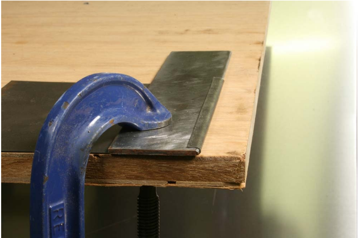
Fig. 7-21: Wired edge: close the flange on the former.
