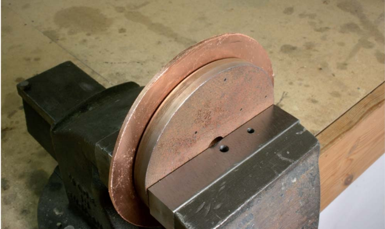
Fig. 9-3: Clamp the former plate and the blank.
