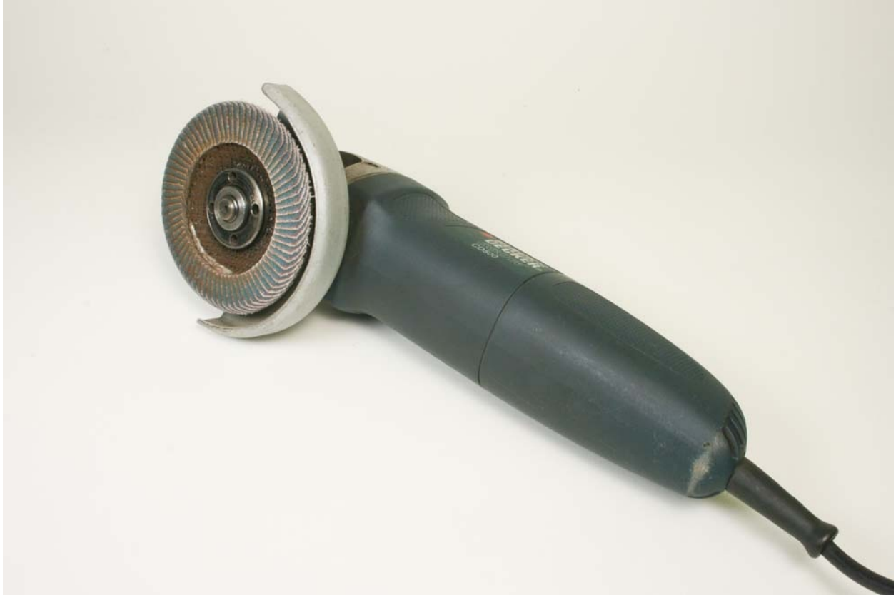
Fig. 10-3: A hand-held grinder fitted with a 115mm Zirconium flap disc.
