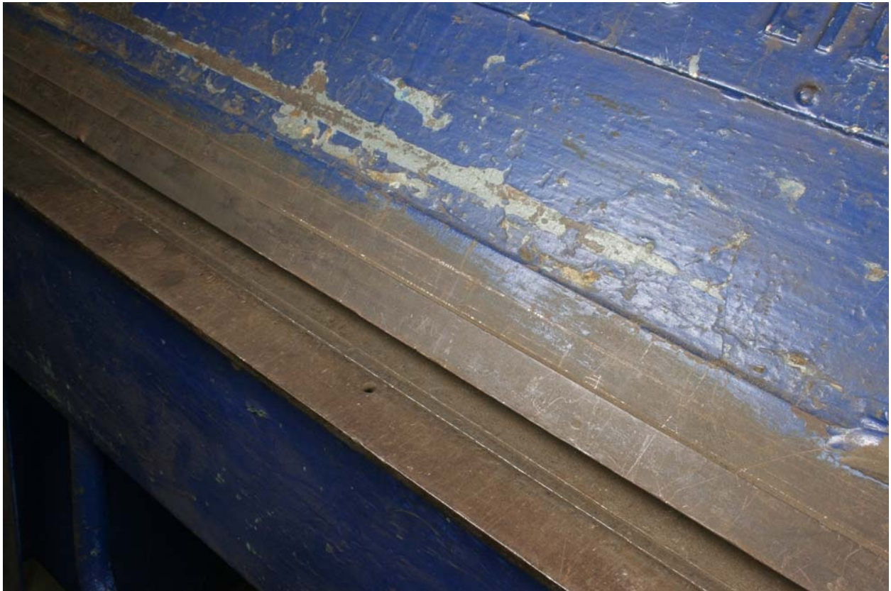
Fig. 6-4: Folder featuring a solid clamp beam.
