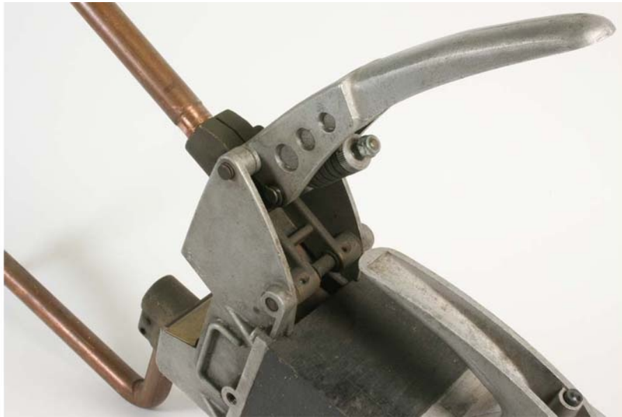
Fig. 8-51: Pressure adjustment under the top handle.
