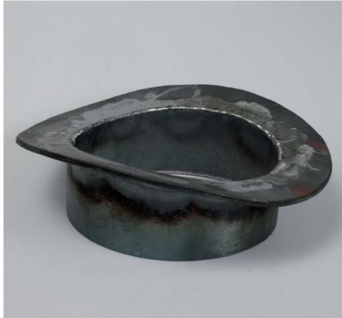
Fig. P4-12: Completed external tube and flange.
