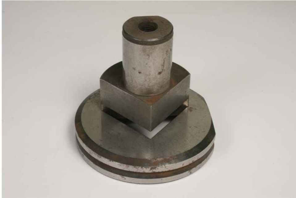
Fig. 5-22: The rear circular portion of this corner-notching punch locates in the die and acts as a guide.
