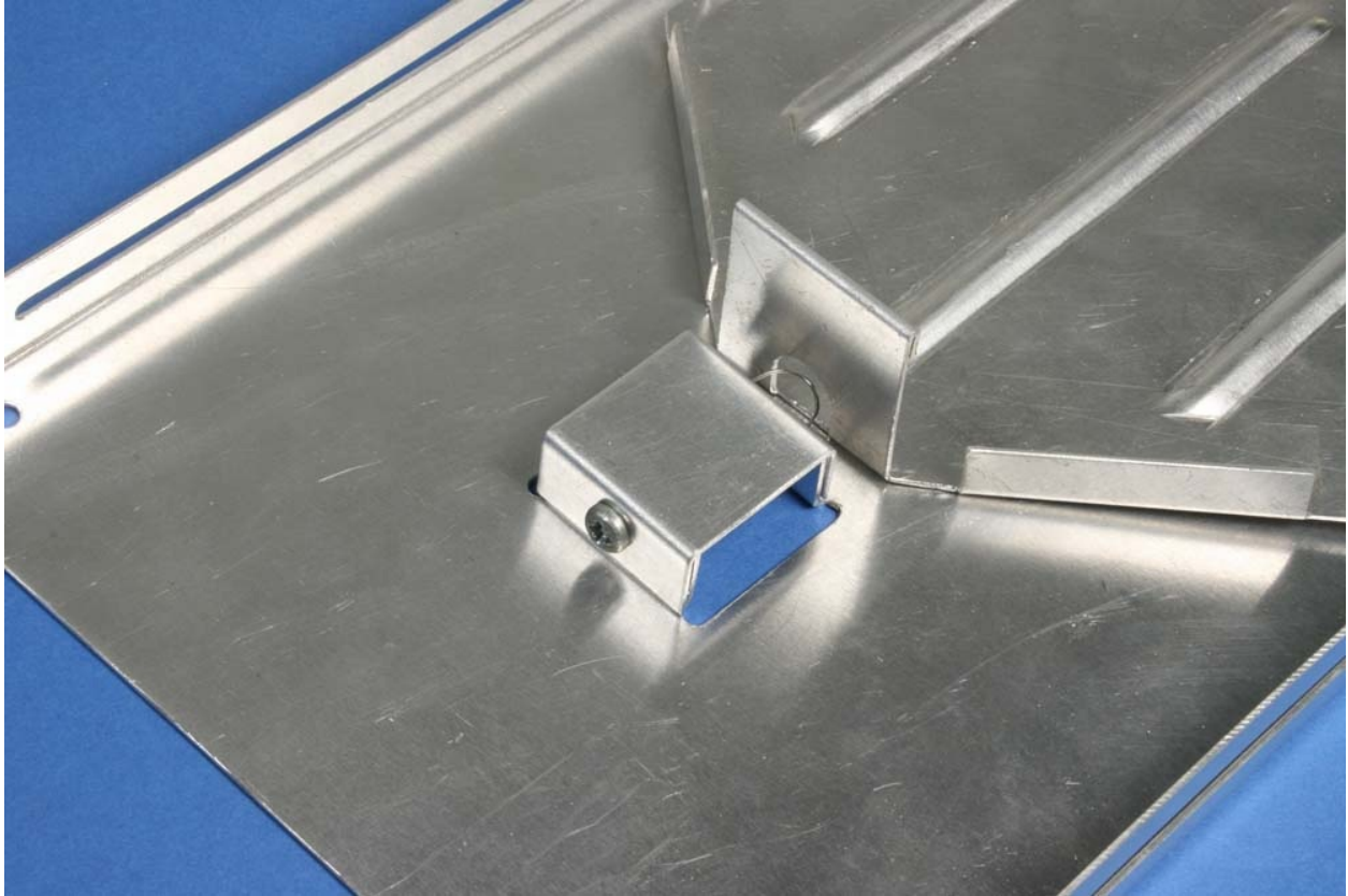
Fig. P7-18: The completed catch, with the wire loop positioned to just catch the shelf.
