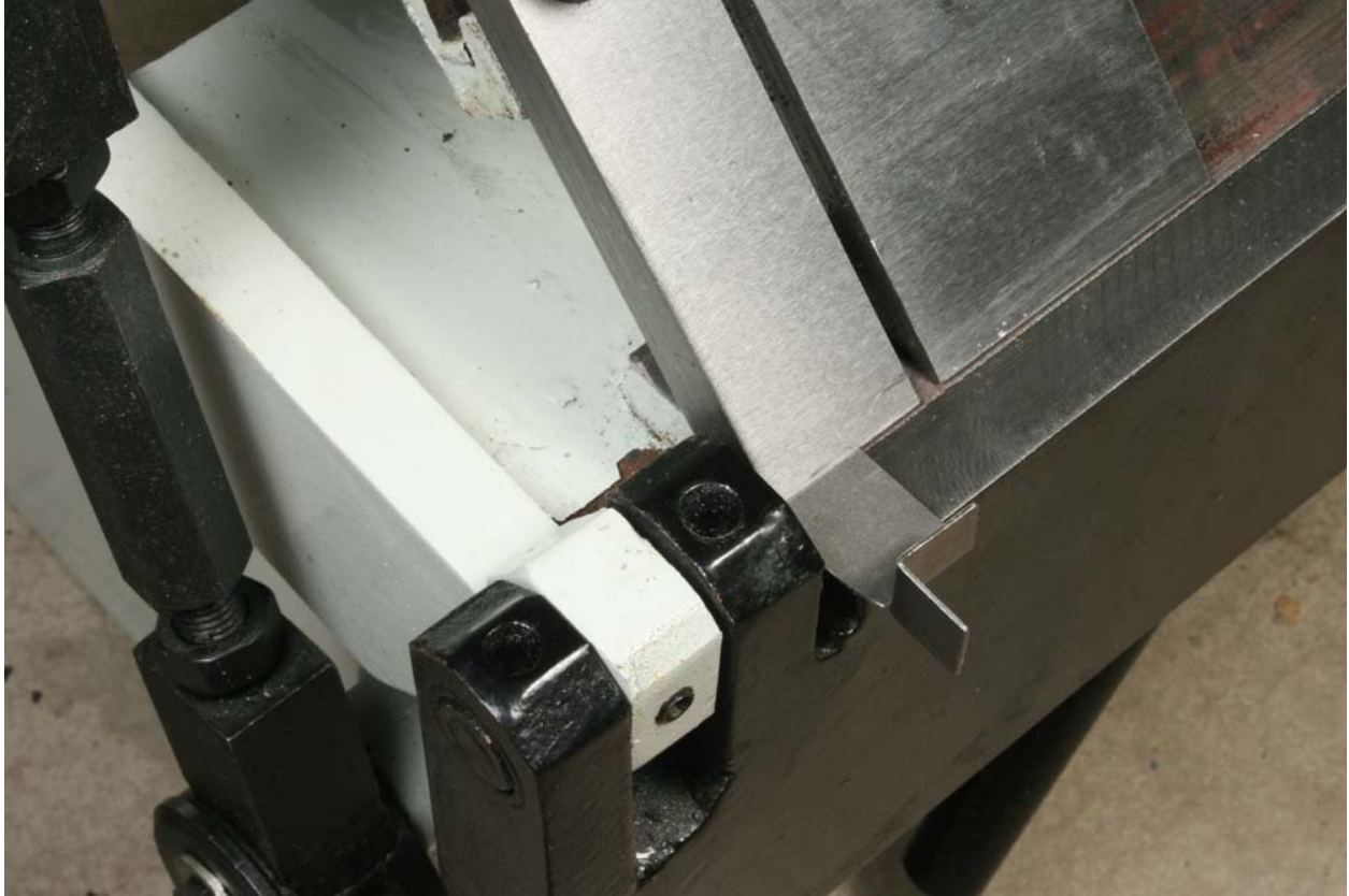
Fig. P2-21: Working at the edge of a finger, fold the body up towards the ear and side.
