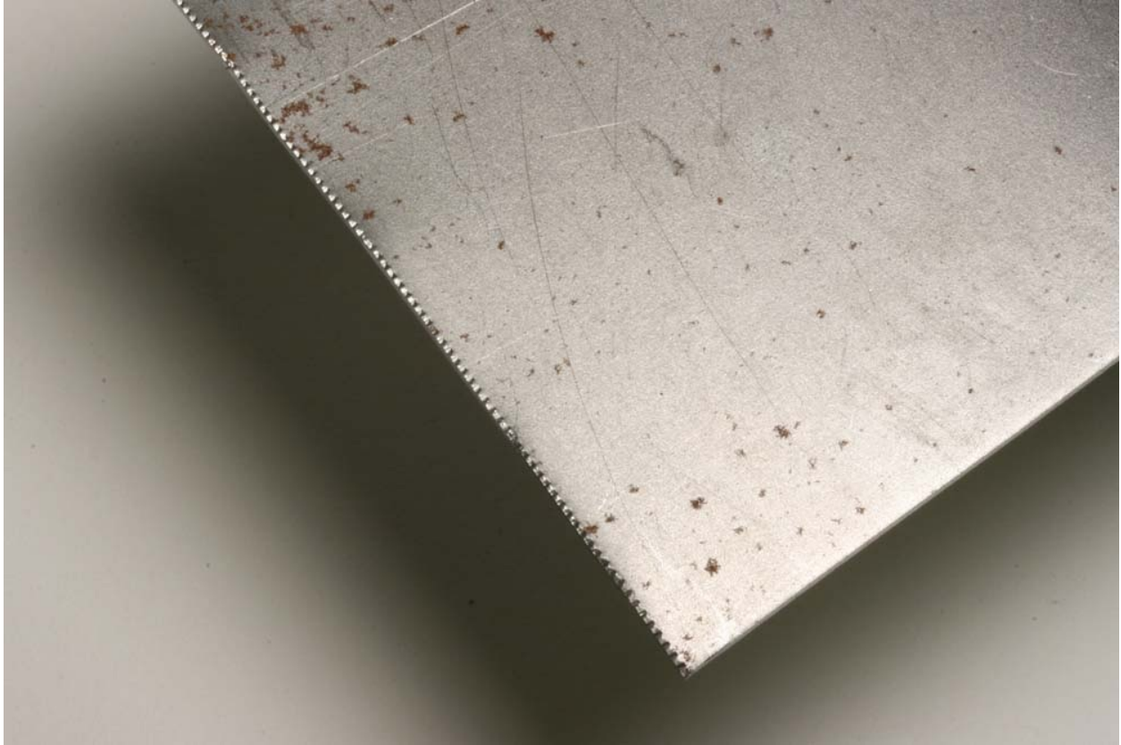
Fig. 4-7: Serrations on an edge left by aviation snips.
