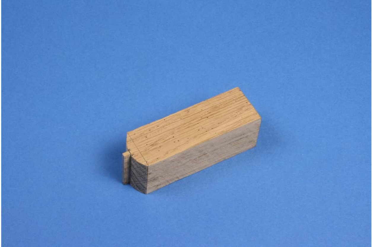
Fig. P7-14: Wooden punch to bend the sides of the spring holder.
