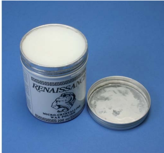
Fig. 10-16: Polished surfaces can be protected by applying a thin layer of microcrystalline wax, which is then polished to a high finish.
