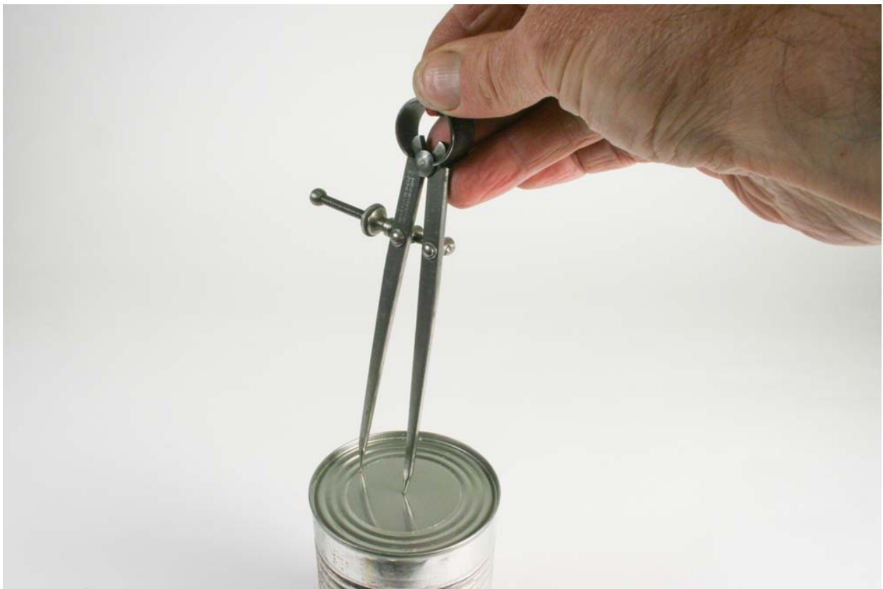
Fig. P2-8: Scribing the circle to be cut for the ammeter, using dividers.
