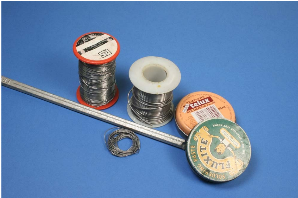
Fig. 8-43: Soft solder in wire and stick form, and tins holding different grades of soldering paste.
