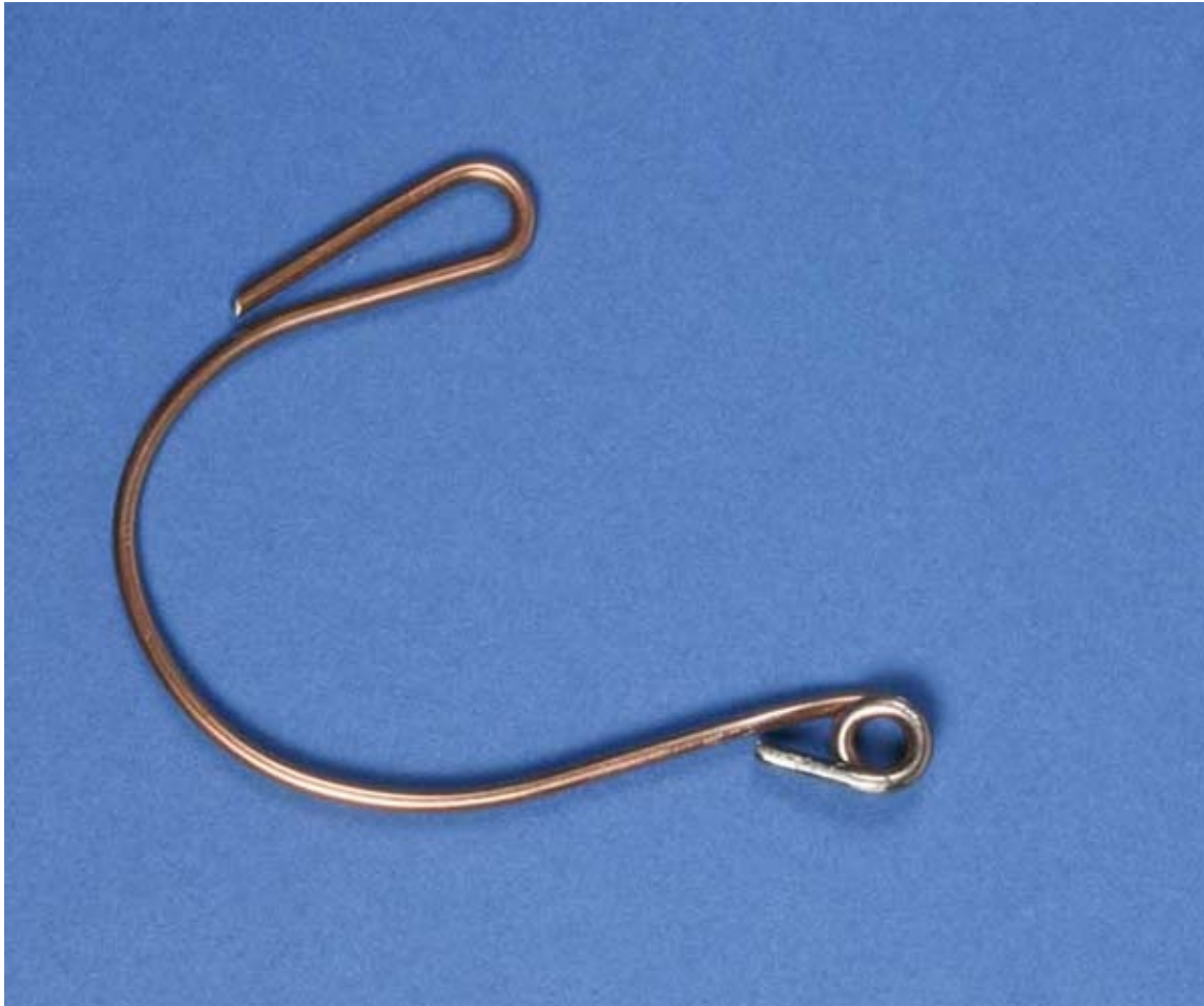
Fig. P7-27: The cable hook is bent to a pleasing shape, and the cut ends are tucked out of the way.
