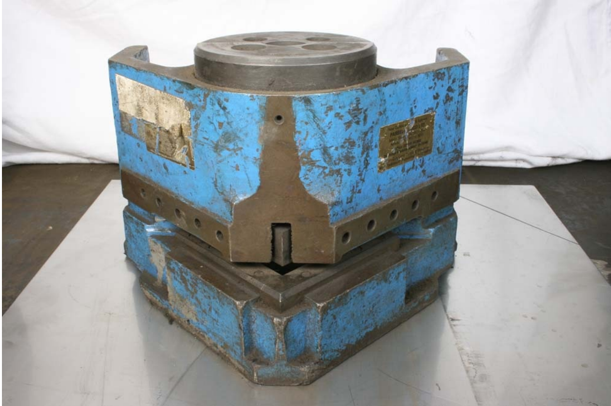
Fig. 4-20: Self-contained corner notching punch and die set for use in a hydraulic press. The notch can be cut the full length of the aperture.
