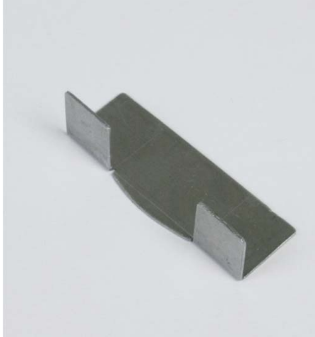
Fig. P2-19: Fold the ears individually, in a vice.
