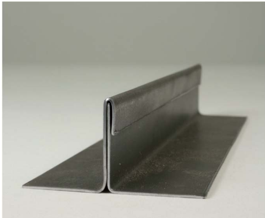
Fig. 8-37: A folded edge holding a second sheet part in position.
