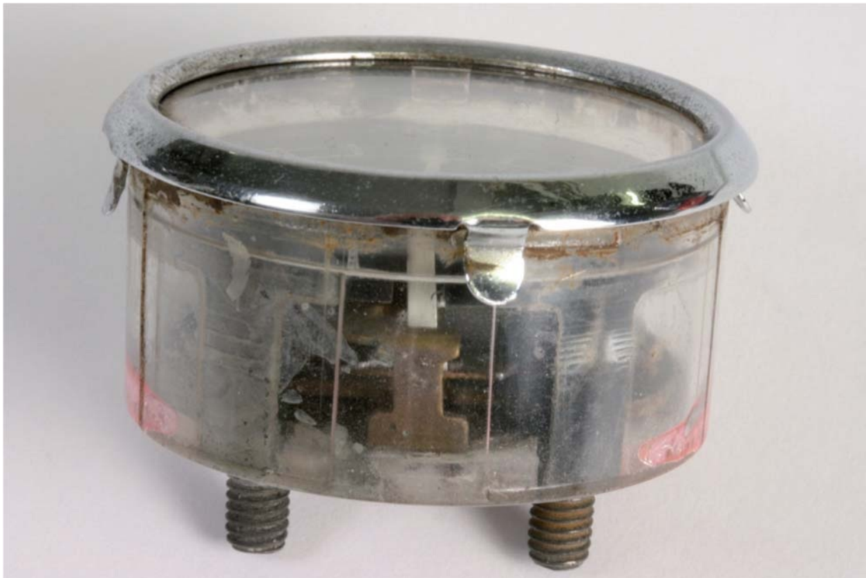
Fig. P2-2: The ammeter has four tabs under the bezel.
