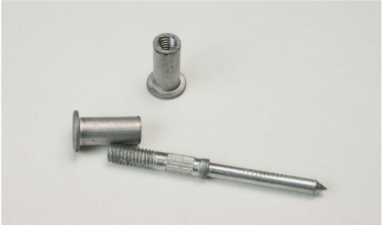
Fig. 8-31: Rivnuts and a closing mandrel which can be gripped and pulled by pop rivet pliers.
