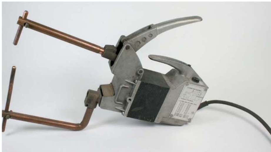
Fig. 8-53: Fitted with appropriate tips and arms, a spot welder can reach into a narrow gap.
