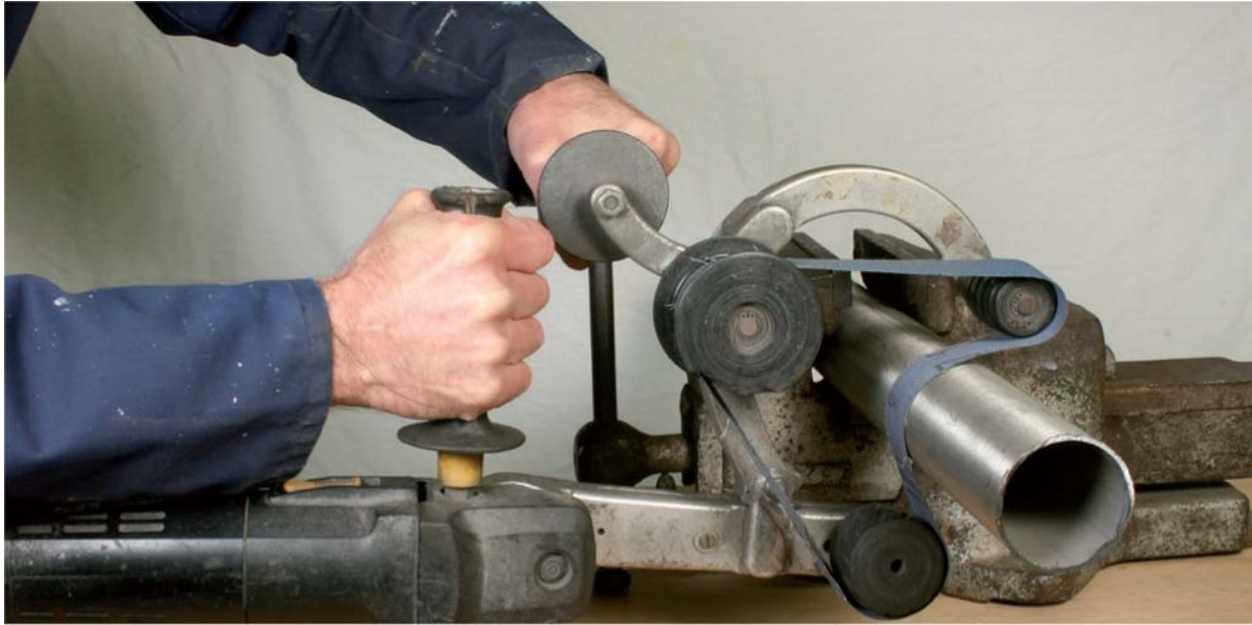
Fig. 10-9: Pressing the free section of the belt against the tube lowers the arms and wraps a section of the belt around part of the curved surface.
