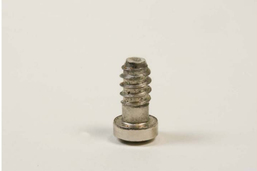
Fig. 8-3: Threads for use in soft materials may have a coarse thread and a substantial core diameter.
