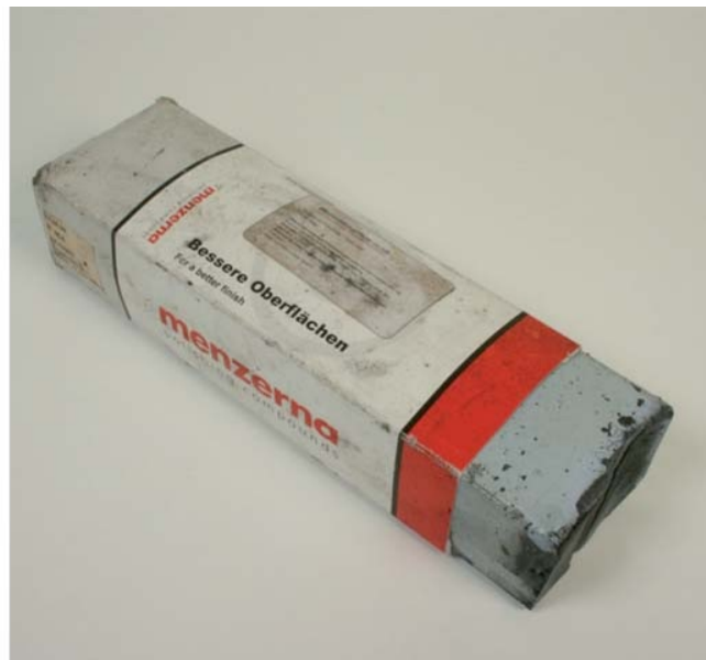
Fig. 10-19: Polish for use on a powered buff is normally supplied in a bar, and is rubbed against the rotating mop, charging it with abrasive.
