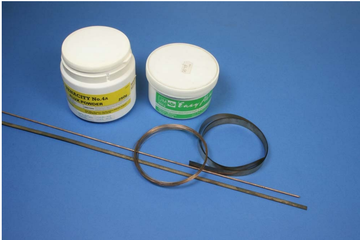
Fig. 8-44: Silver (hard) solder in strip, rod, wire and foil form, and silver-soldering apastes.
