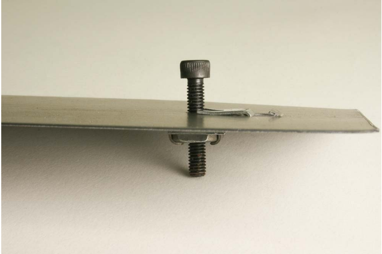
Fig. 8-12: U nuts can also be used in the centre of a panel by punching a slot and creating a bent tab.
