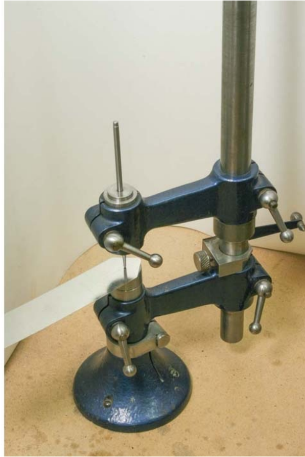
Fig. P1-7: Piercing punch in a staking tool.
