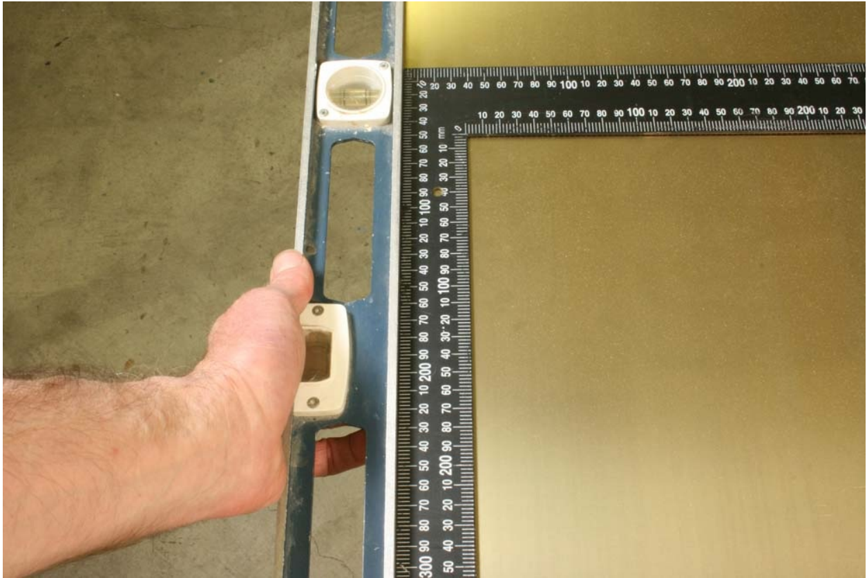
Fig. 3-8: Use a straight-edge to make sure a framing square is aligned with an edge. .
