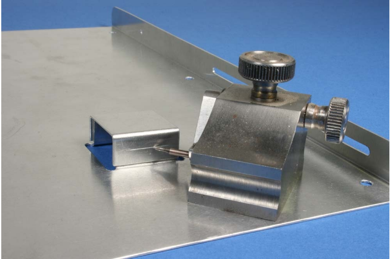
Fig. P7-22: Transferring the distance to the top clip.
