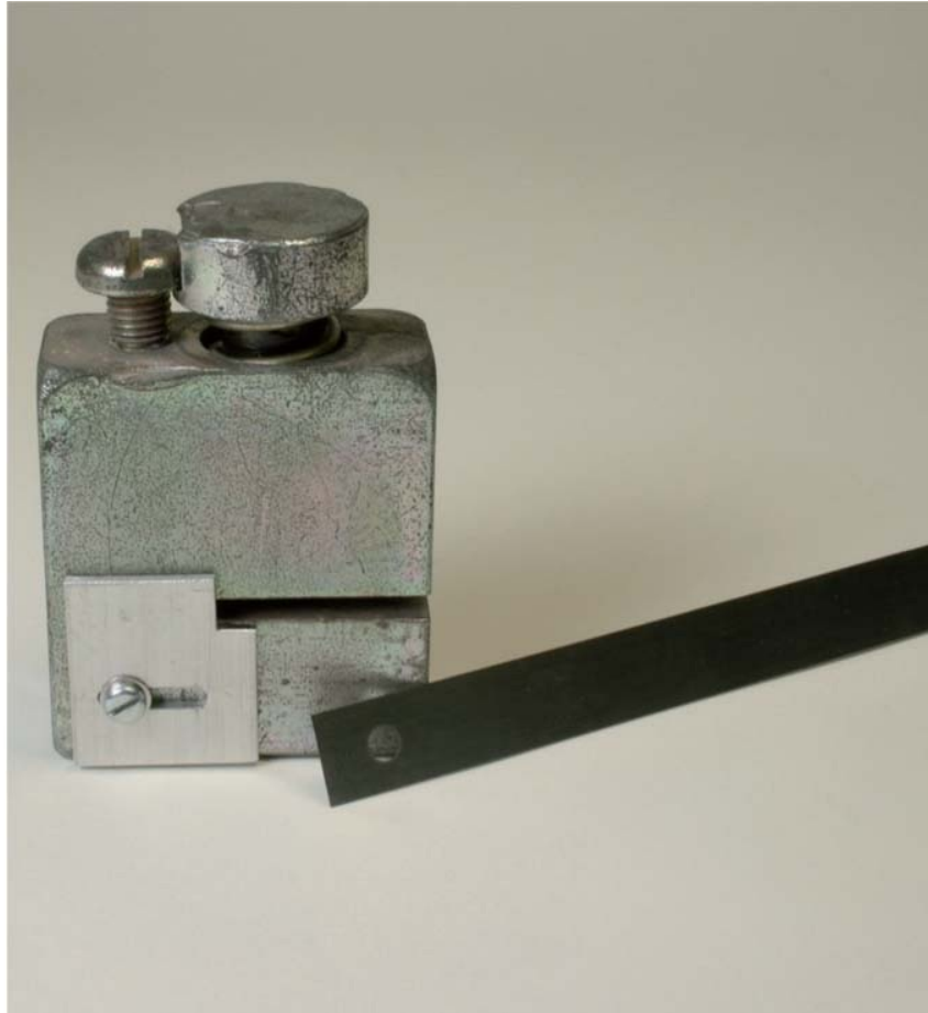
Fig. 5-12: Small hammer-operated punch, fitted with a width guide.
