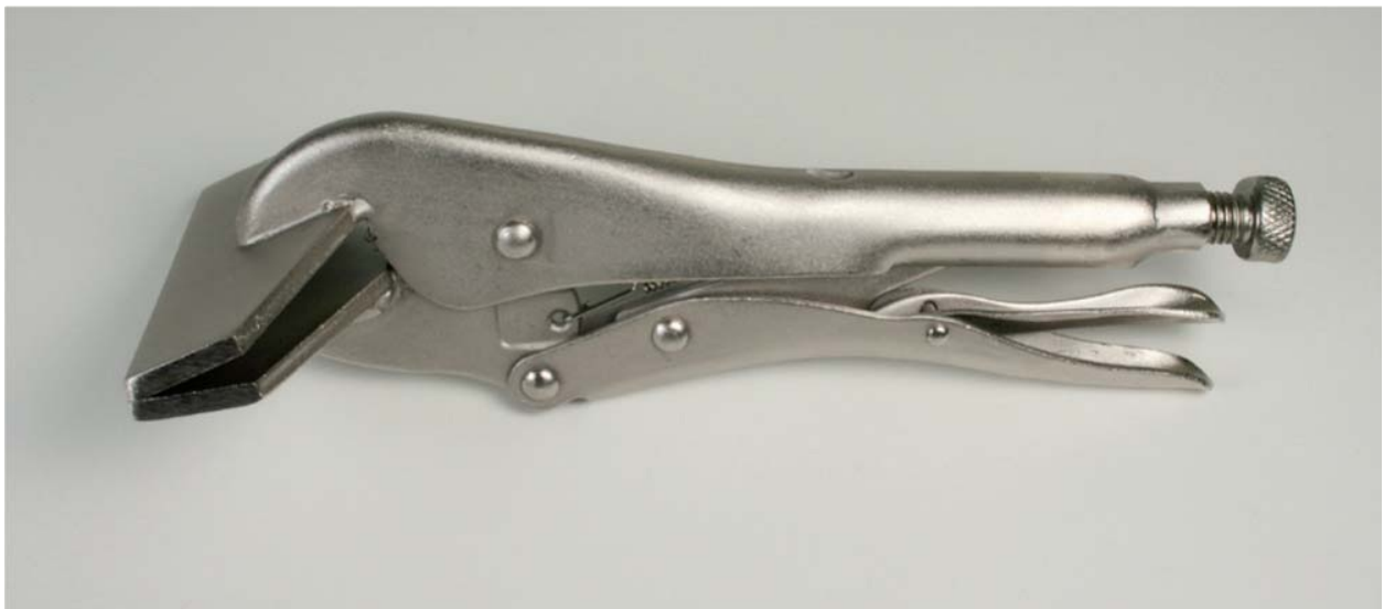
Fig. 8-57: Self-gripping pliers designed for sheet use.
