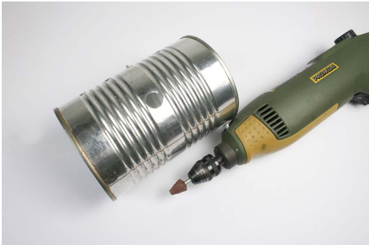
Fig. P2-15: Drill the hole, then bring it to size and finish the edges with a small grinder.
