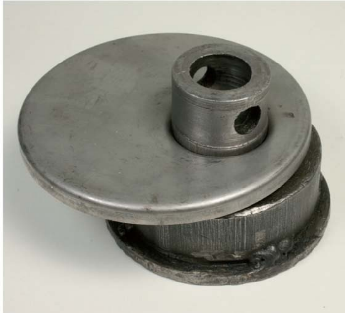
Fig. 9-11: The plate is located by its outside flange, and the die is forced through the hole to produce a flange.
