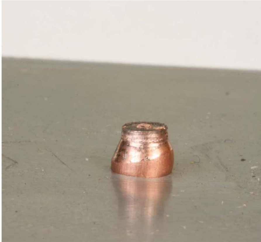
Fig. 8-21: The tail of a rivet after the cone tool has been used.
