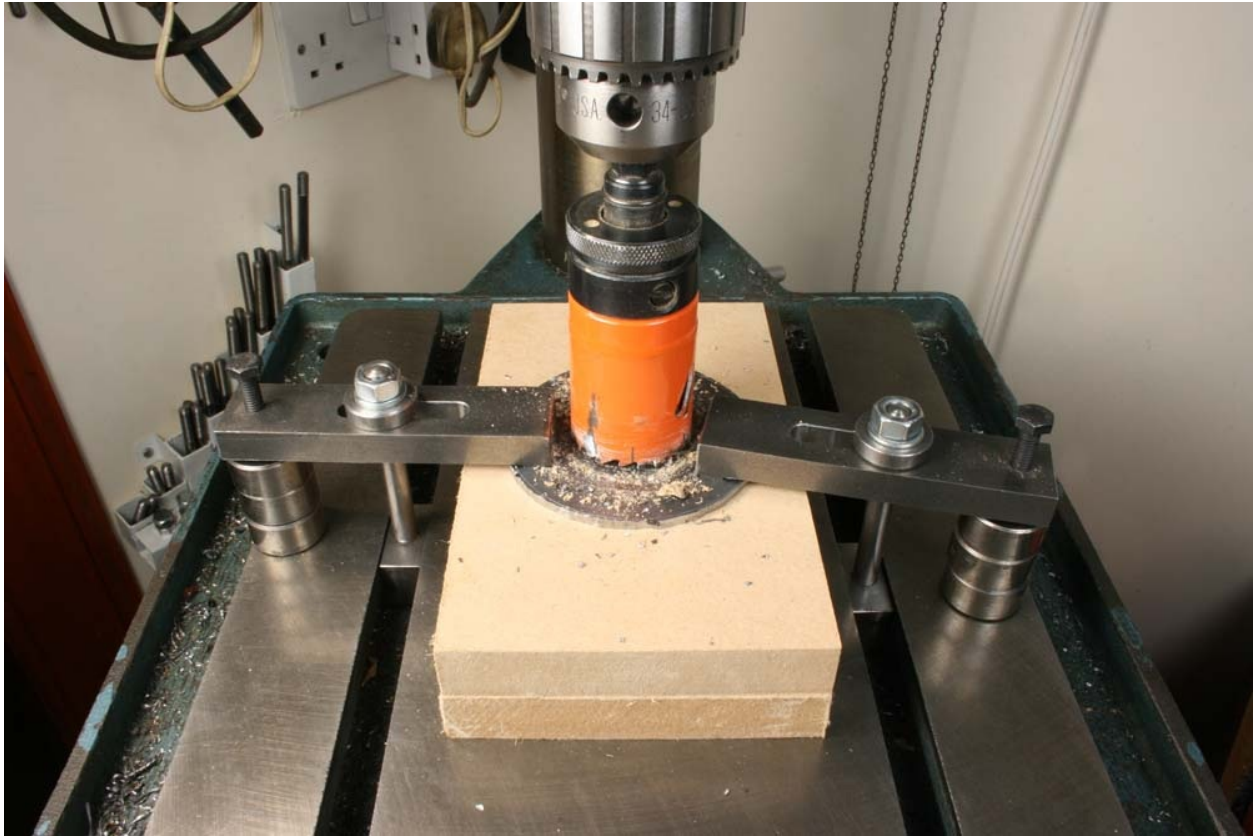
Fig. 5-1: Use at least two strong clamps to secure work in the drilling machine.
