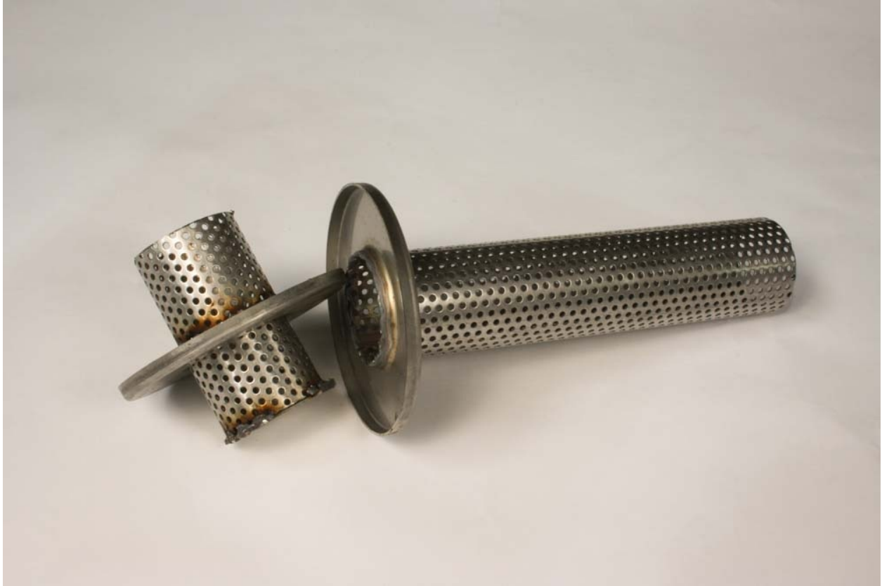
Fig. P5-6: The inner supporting flanges welded to the perforated tubes. The smaller tube has a blanking plate welded to the inner end.
