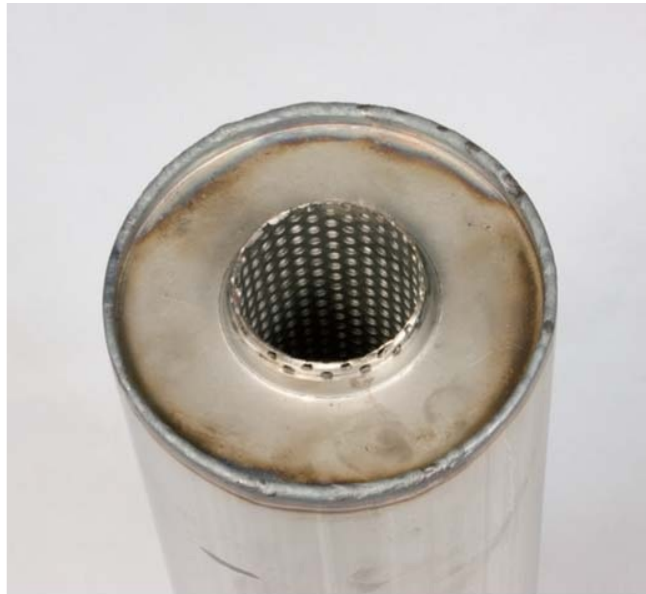
Fig. P5-10: The end flanges are inserted then fully welded to the outer tube. The inner welds will be made as the chamber is fitted to an exhaust system.
