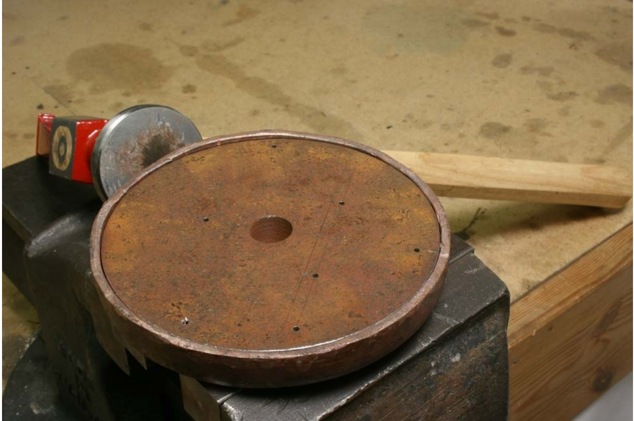
Fig. 9-5: After annealing the blank, tap it into close contact with the plate, then use a plan-ishing hammer to finish the work.
