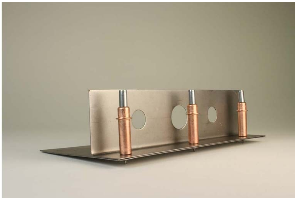
Fig. 8-60: Clecos in use holding two parts together.
