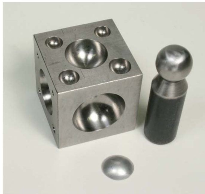
Fig. 9-6: A doming block, doming tool with spherical head, and an aluminium item made from a flat blank by placing it in a recess and using a hammer to tap it down with a doming tool.
