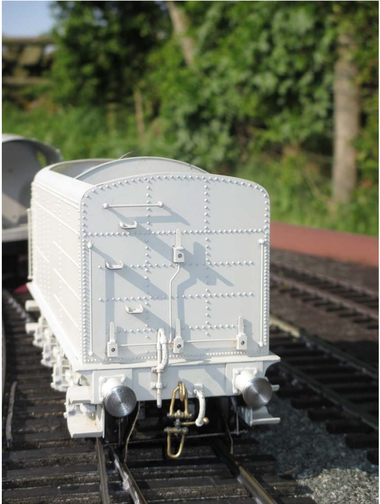
Over 1,000 hand-set rivets. A Gauge 1 model of the tender of an A1 locomotive built by Dave
