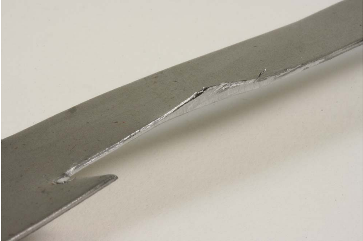
Fig. 4-2: A chewed edge as a result of the shearing action of snips.
