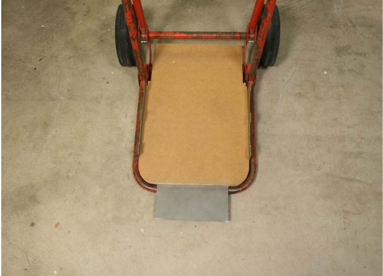
Fig. P6-7: Hold the wooden former in place while forming the sides of the base over the side tubes of the barrow.
