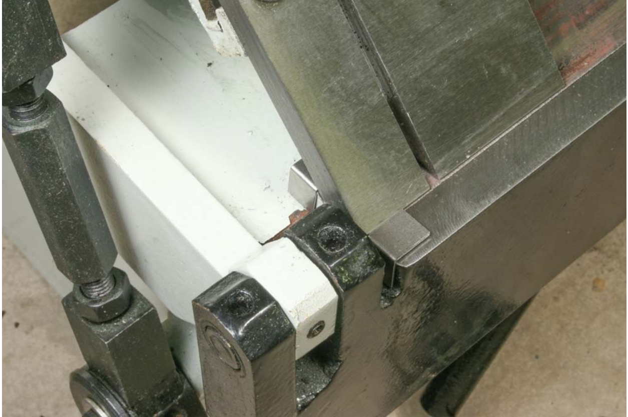
Fig. P2-20: Fold one side using the channel at the end of the folder to accommodate the folded ear.
