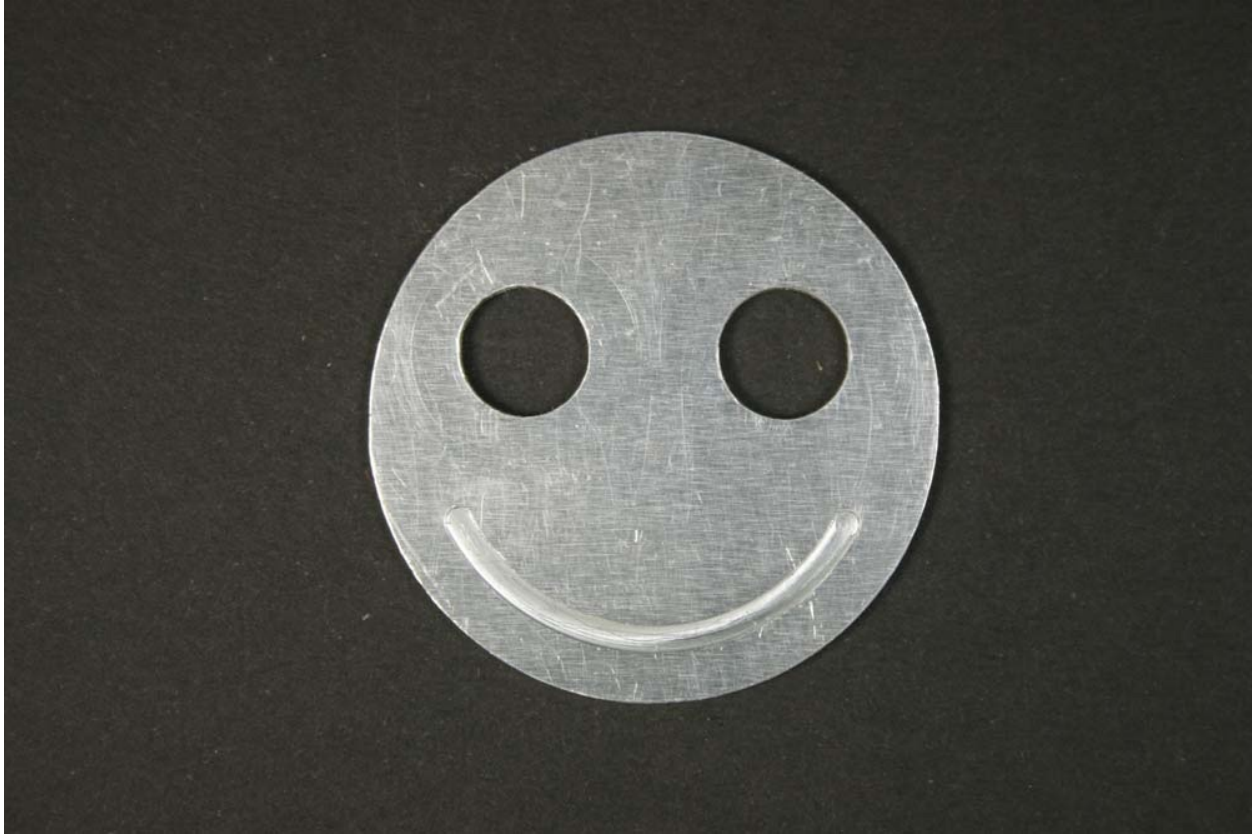
Fig. 3-1: Sheet component made by cutting out on a milling machine.
