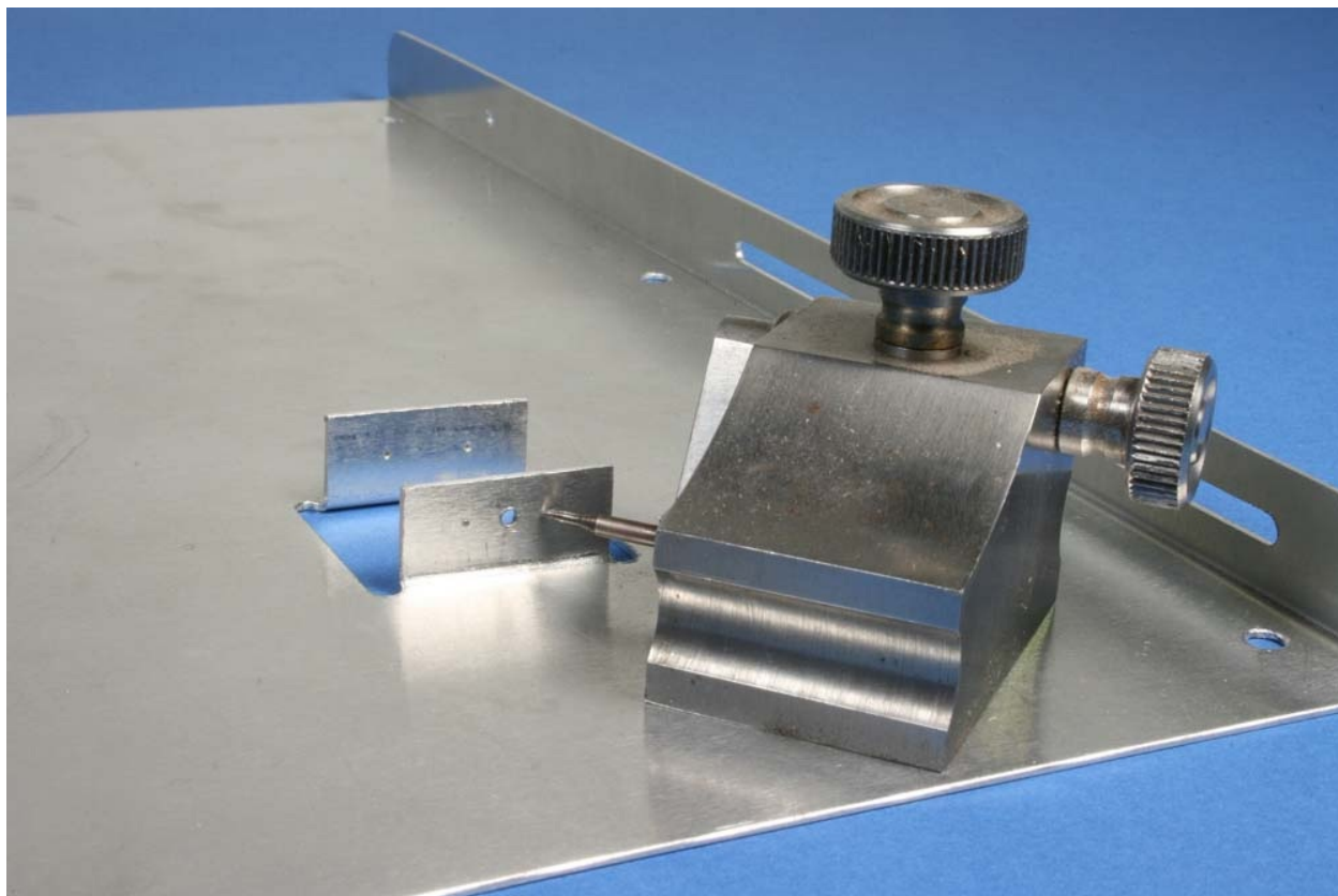
Fig. P7-21: Using a height gauge to find the distance from the base plate to the spring holes.
