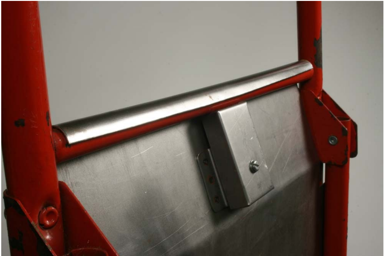
Fig. P6-16: Lock box fitted, and preventing the rear panel from coming loose by moving upwards.
