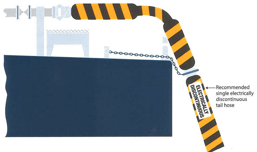
Figure 2.7: Recommended method for providing electrical isolation
