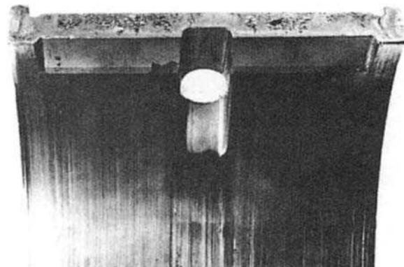
Figure 13.20 Fretting of a bearing joint face due to inadequate bolt load
