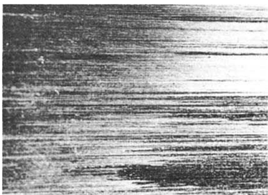
Figure 13.22 Pitted surface caused by electrical discharge
