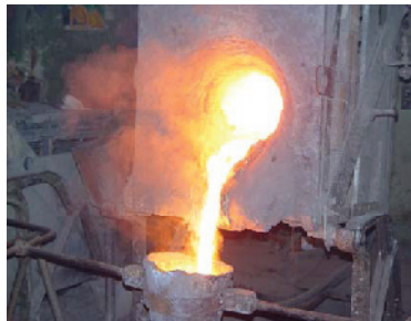
Figure 5.19 Melting of bronze in an induction furnace. Reproduced from Mansurov ZA, Fomenko SM. (2014). Carbonaceous refractory materials on SHS-technology. Adv. Sci. Technol. Mater. Res. , 88 : 112–128.
