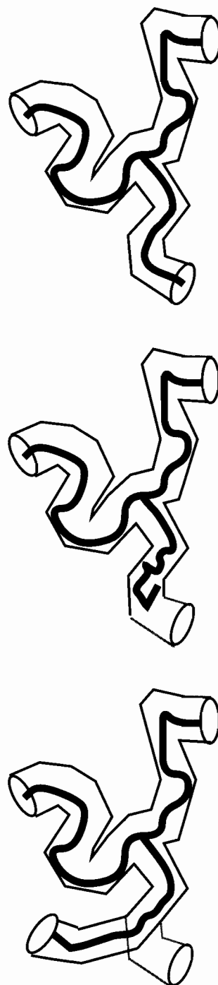
Fig. 5.11 Tube relaxation by contour length fluctuation in a star polymer. The star is unable to escape from its non-linear tube by reptation (top), but if one of the arms is retracted into the tube by a fluctuation in contour length (middle) it will re-emerge in a new relaxed configuration (bottom).
