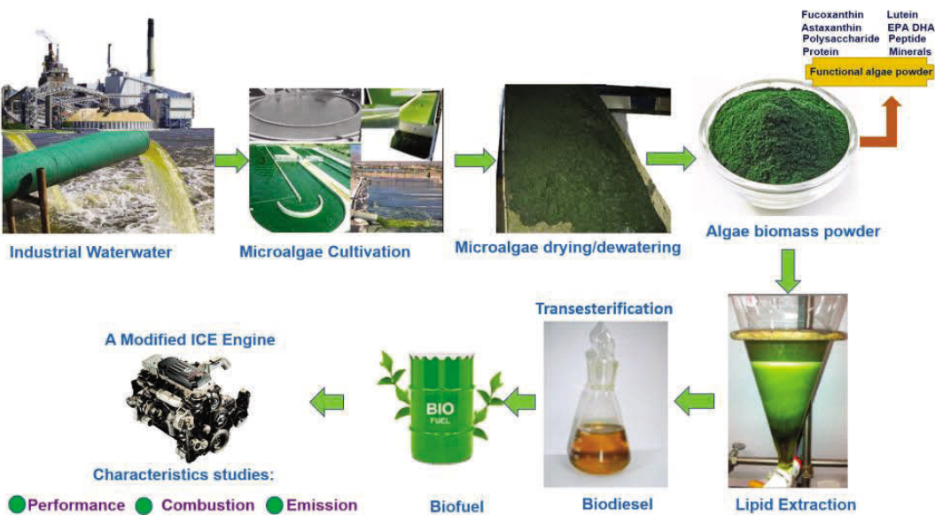
Figure 6. Microalgae-based biofuel production method.
