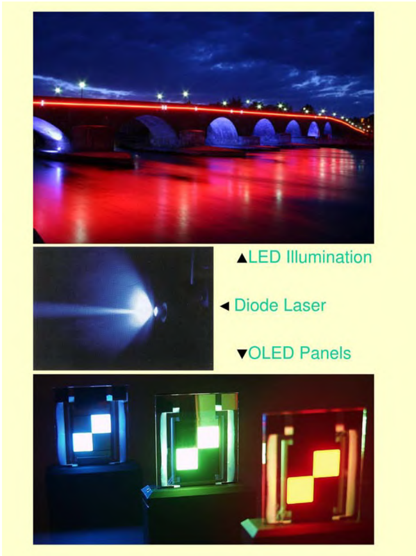
Fig. 7.18. Demonstration of light emitting diodes: Illumination of the Stone Bridge in Regensburg (Germany) with 142 red, green and blue diodes made from III-V nitride semiconductors (top); after [7.21]. Pulsed laser light emission from an InGaN multi-quantumwell laser (center); after [7.19] and blue, green and red light panels from organic light emitting diodes (bottom); after [7.22]
