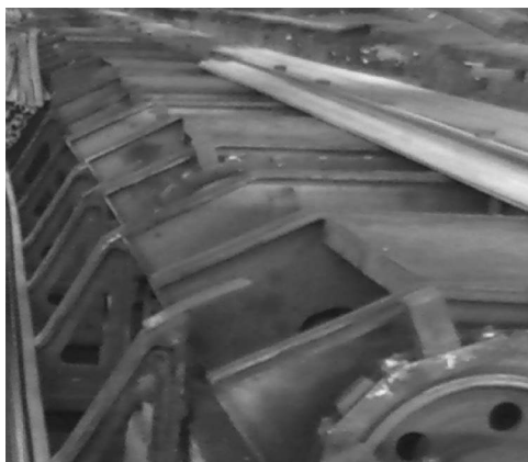
Fig. 13.3 Piling of stock by chain Transfer.
