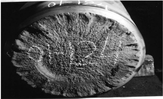
Fig. 3.14 Roll Failure–Brittle Fracture.
