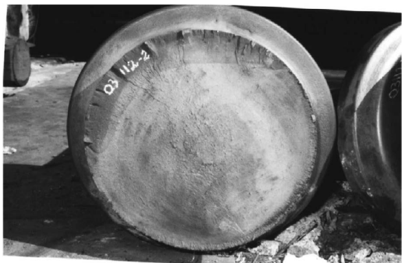
Fig. 3.15 Roll Failure–Fatigue Fracture.
