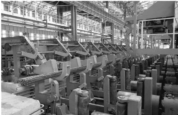
Fig. 14.9 Typical Bundling Station with Strapping Machine.
