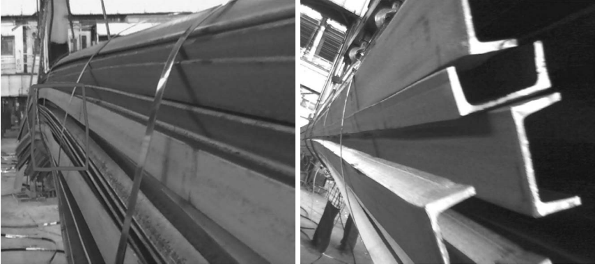
Fig. 13.6 Straps for Strapping of Bundle.
