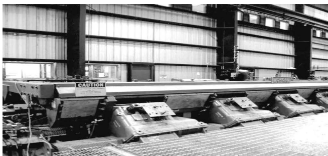
Fig. 14.7 H/V Finishing Block.
