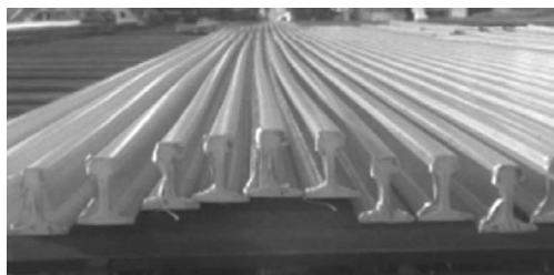
Fig. 14.46 Camber in Rail while transferring in cooling bed.
