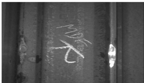
Fig. 14.48 MDF (Mechanical Defects during Finishing).
