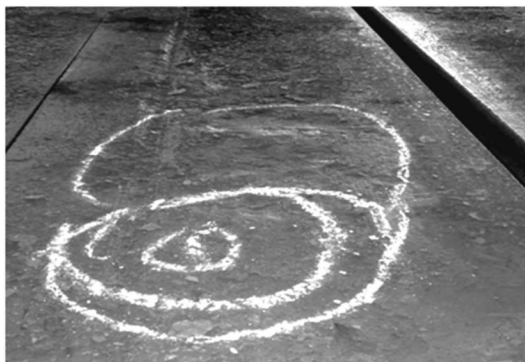
Fig. 11.36 Casting Powder Entrapment
