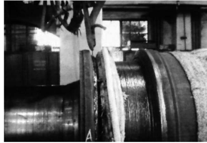
Fig. 3.23 Welding of Rolls.
