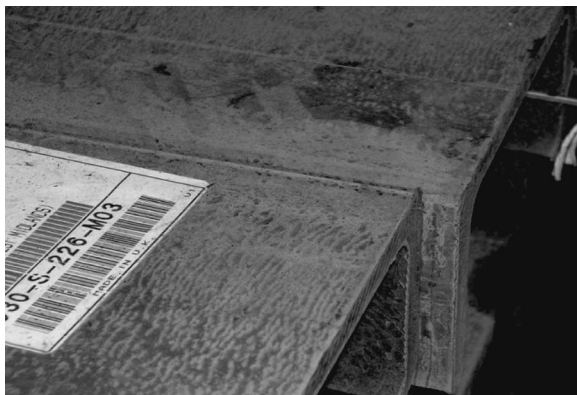
Fig. 9.40 Fins & Bevelled Corners on Channels.
