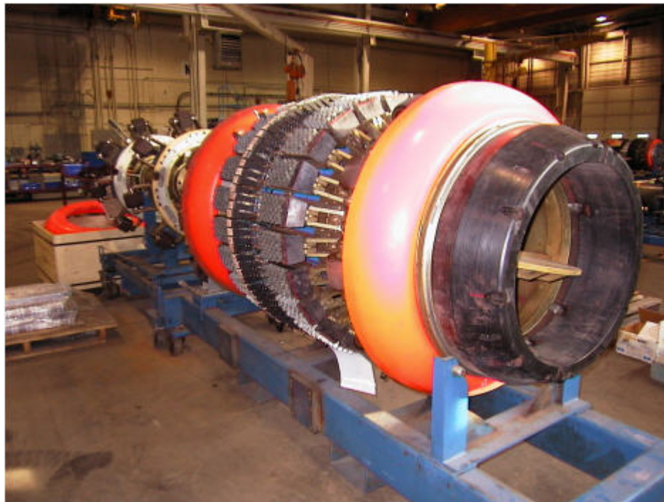
Figure 6.3: MFL ILI tool with bypass – product flow is allowed to ‘bypass’ through internal bore and tool travel speed is controlled by valves
