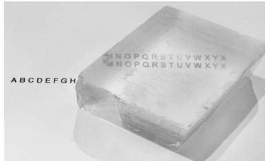
Fig. 1.2 Double refraction of calcite. The light passing through the crystal is split into two separate beams that are refracted differently, leading to two images transmitted through the crystal. The way that the double refraction changes as the crystal is rotated points to the presence of special axes within the crystal.
