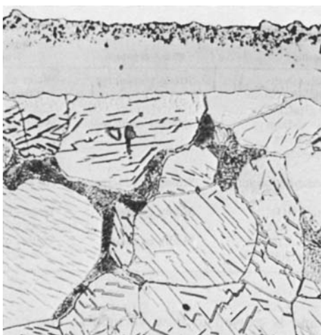
Fig. 20 Nitrided case and diffusion zone produced by cyanide-cyanate liquid nitriding. The characteristic needle structure is seen only after a 300 °C (570 °F) aging treatment.
