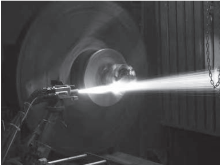
8.11 HVOF process where particles in the spraying jet are seen.
